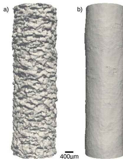
**Figure 1.36:** 3D renderings reconstructed from X-ray tomography scans of a sample gauge length portion before (a) and after (b) USP. After the USP treatment, the sample presents a surface state close to the one obtained by machining.
