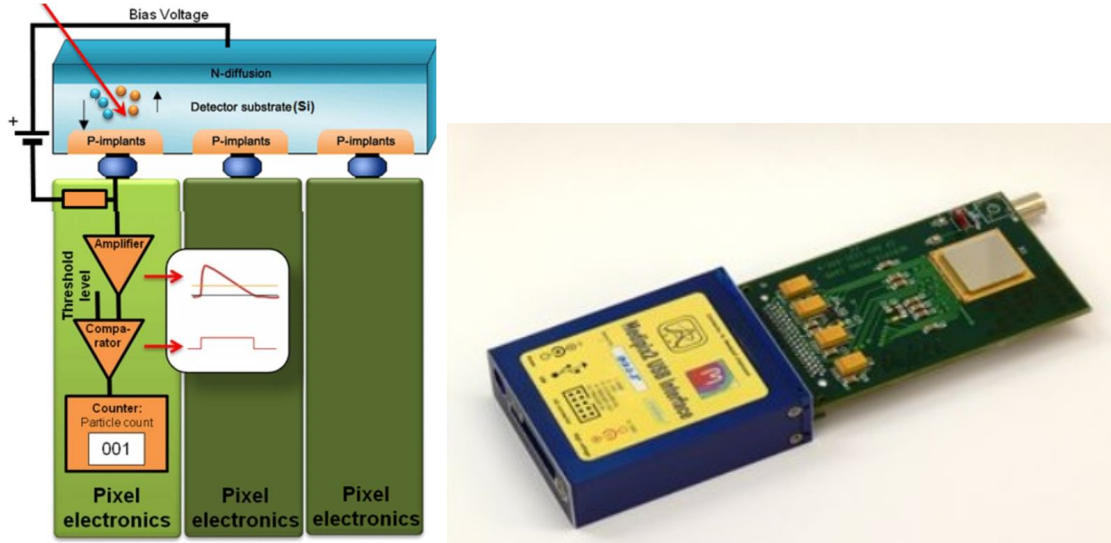
Figure 1.10: (Left) Principle of the photon counting in a single pixel.(Right) Standard, single chip MEDIPIX carrier board with USB readout.
