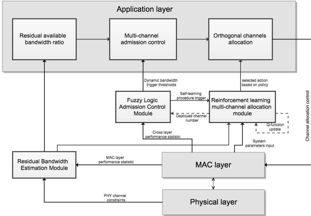
Figure 4.2: Multi-channel Dynamic Bandwidth Assignment Structure
