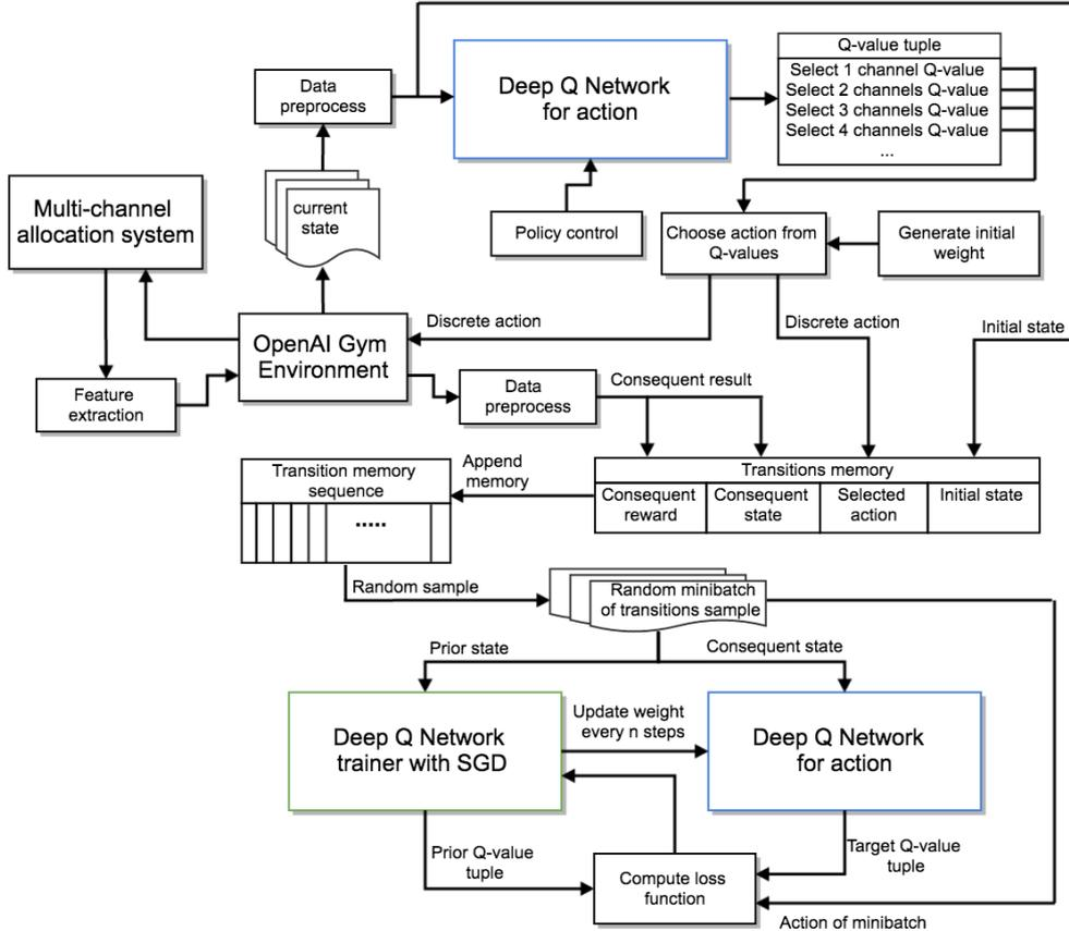
Figure 5.1: Reinforcement learning of multi-channel allocation with deep Q-network (DQMC)
