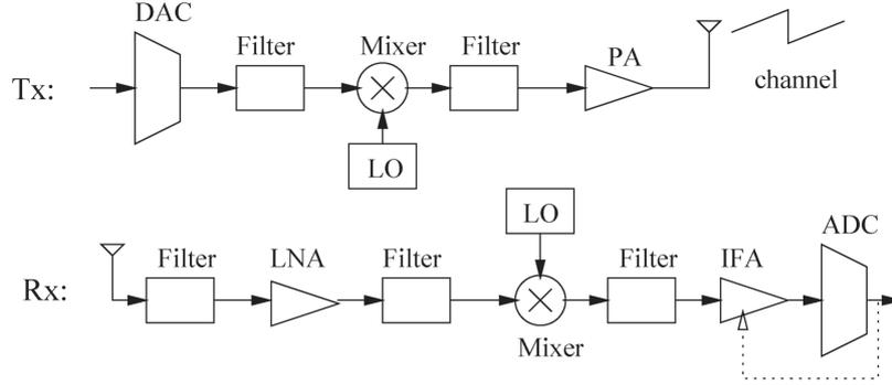
Figure 3.4: Typical transceiver structure
