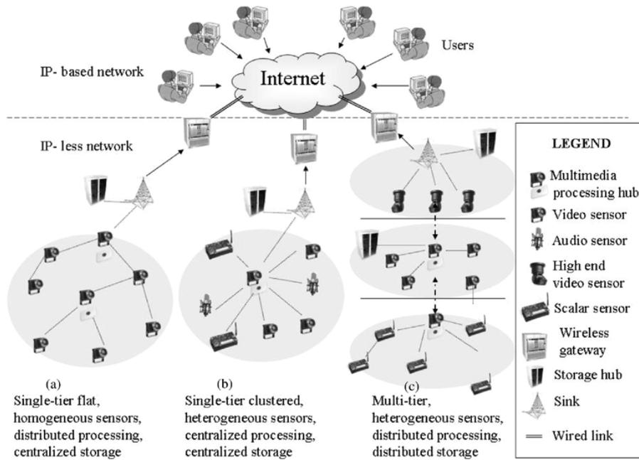
Figure 1.2: Reference architecture of wireless multimedia sensor network.
