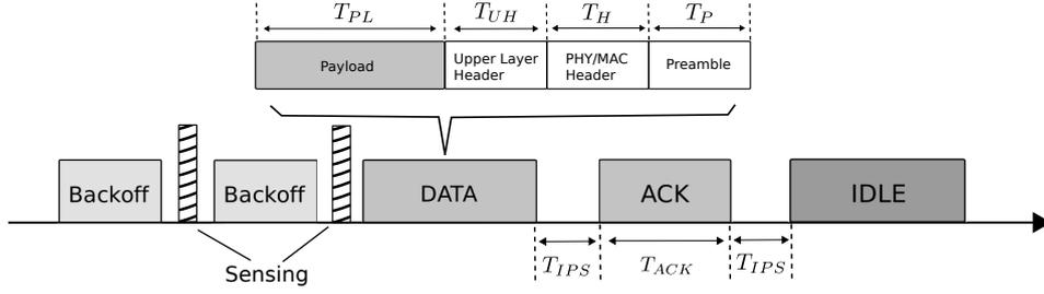
Figure 4.3: IEEE 802.15.4 frame exchange sequence
