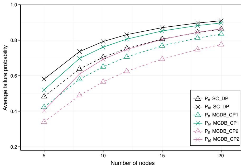
Figure 4.9:  $P_{tf}$  and  $P_{bf}$  of different sensor nodes
