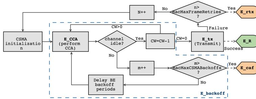
Figure 3.5: Effective energy consumption in CSMA/CA mechanism
