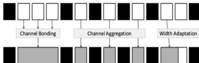
Figure 2.1: Concepts of Channel Bonding, Channel Aggregation, and Channel Width Adaptation.
