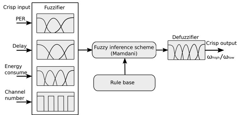
Figure 4.4: Structure of fuzzy logic system
