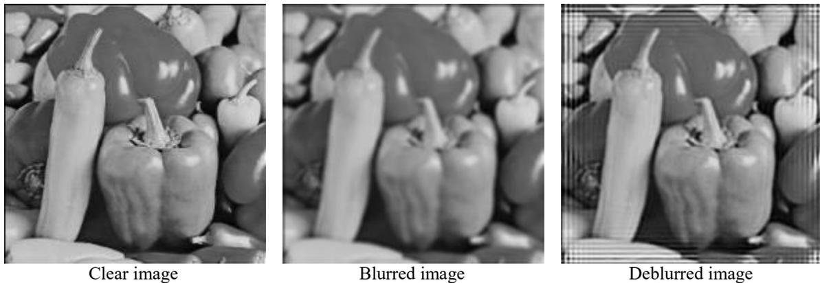
**Figure 2.9:** Deblurring by Constrained Least-Squares filter.
