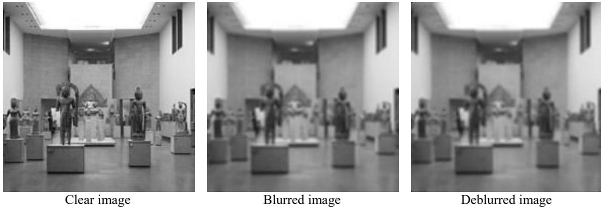
**Figure 2.11:** Deblurring by Median filter.
