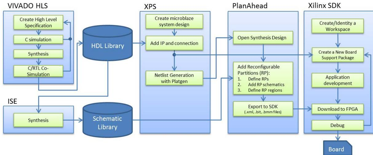
Figure 4.6 Step-by-step development flow using Xilinx tools.
