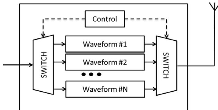
Figure 2.5 Basic software-controlled radio.
