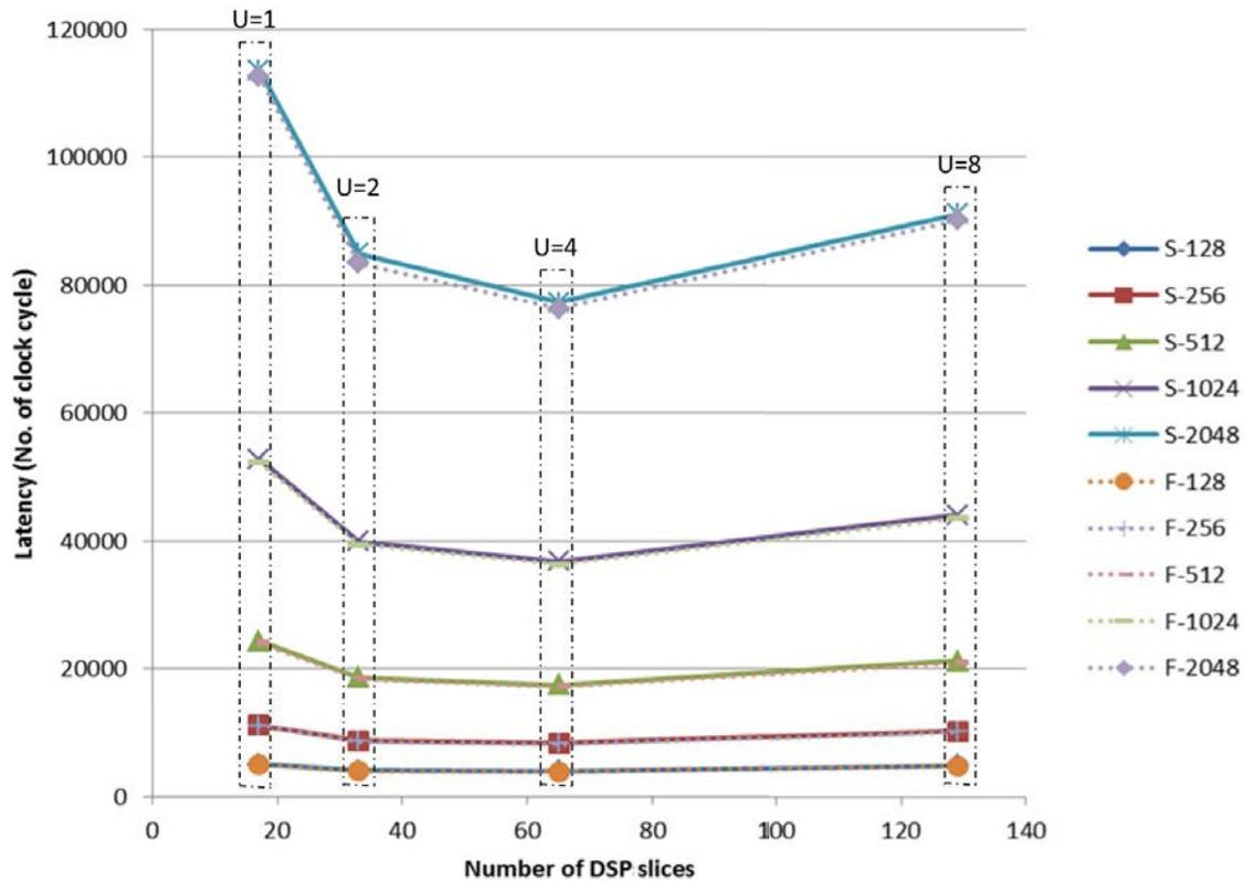
Figure 5.5 The latency vs number of DSP slices (S is for Simulation after synthesis and F is for the Formula estimate) (frequency = 100 MHz).
