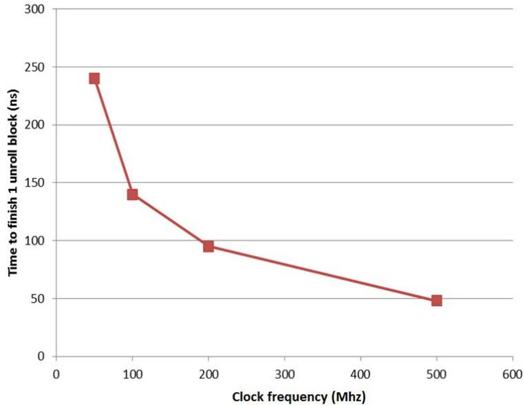
Figure 5.12 The third loop computation time vs clock frequency for U = 4
