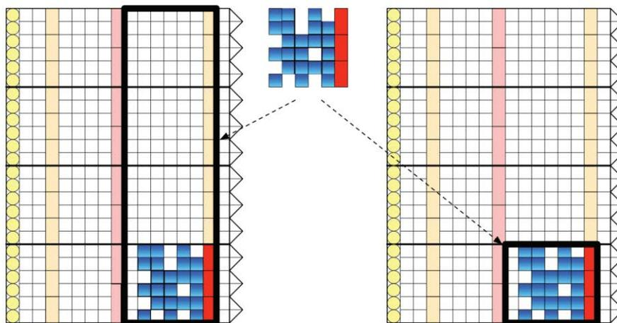
Figure 3.8 Configuration uses 1 address dimension (left) and 2 address dimensions (right) [68].
