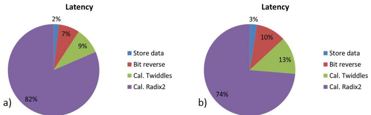
Figure 5.4 FFT latency with unrolling factor U = 1 a) FFT 2048; b) FFT 128.
