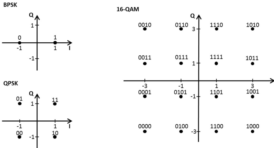
Figure 2.3 The constellations for BPSK, QPSK and 16-QAM.
