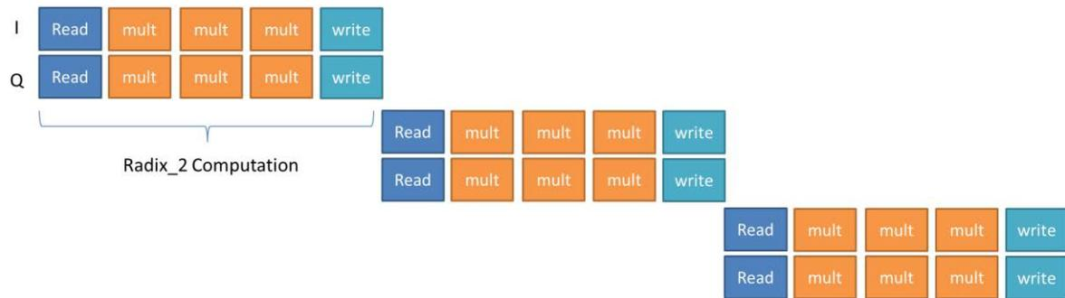
Figure 5.6 Timing chronogram of the third loop based on Algorithm 6.
