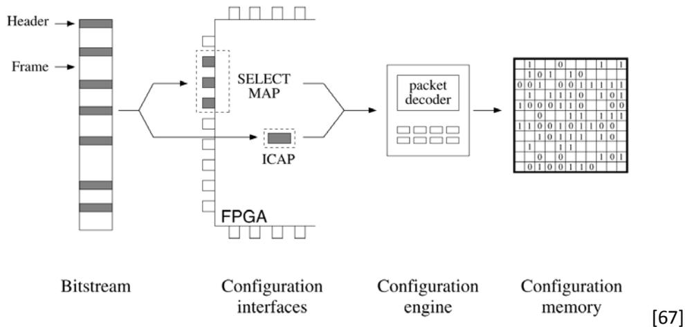
Figure 3.7 The reconfiguration chain for a Virtex FPGA.
