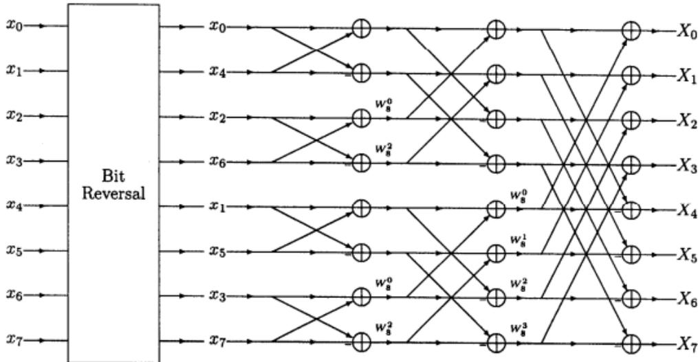
Figure 2.11 An eight-point DFT, divided in four two-point DFTs with bit reversal on inputs [33].
