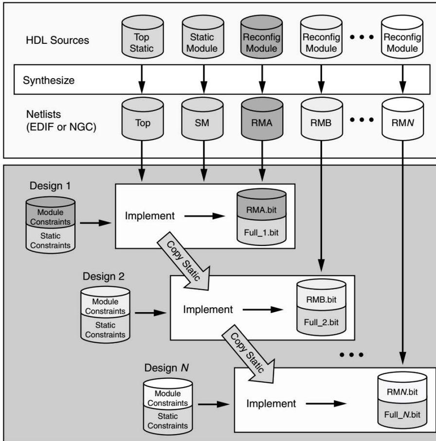
Figure 3.10 Partial reconfiguration software flow [66].
