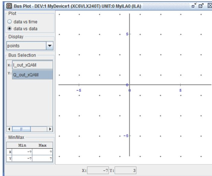
Figure 4.9 Example of baseband level verification using ChipScope Pro Analyzer for 64-QAM data.
