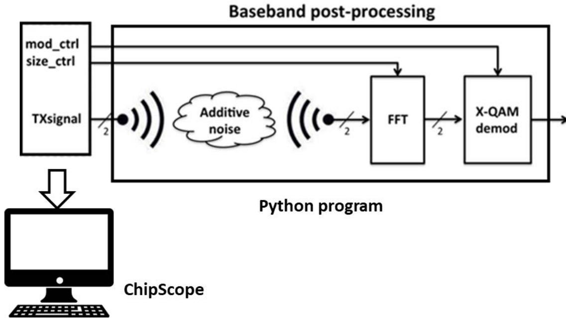
Figure 6.5 The testbed description.
