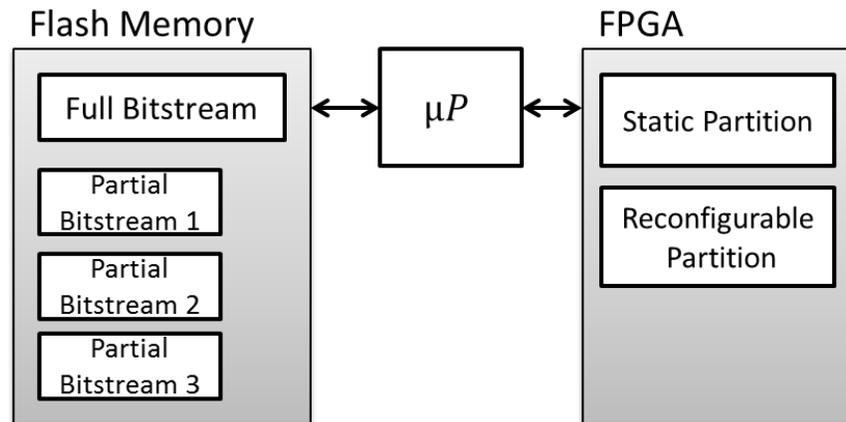
Figure 2.15 Partial reconfiguration.
