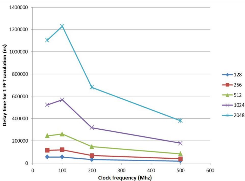
Figure 5.11 Time to compute 1 FFT vs clock frequency,  $U = 1$
