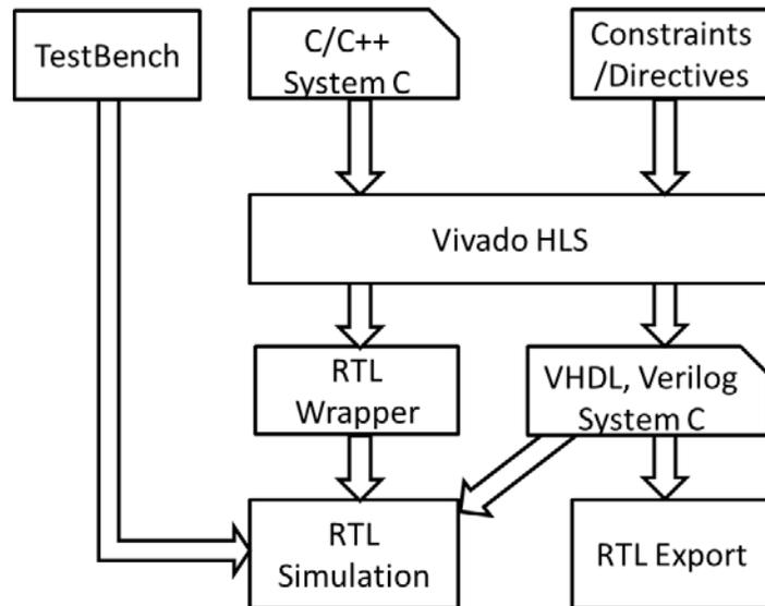
Figure 3.2 The Vivado HLS design flow.
