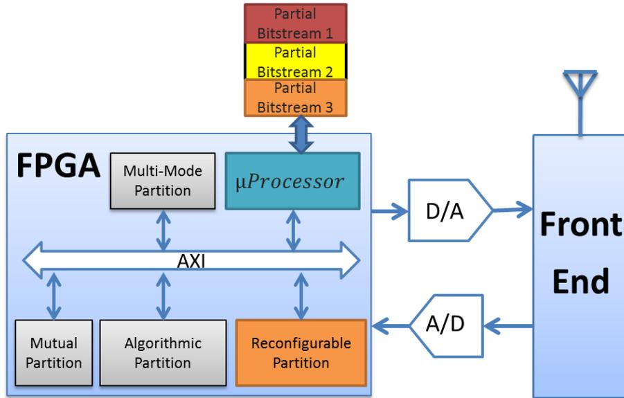
Figure 4.4 System architecture for FPGA-based SDR.
