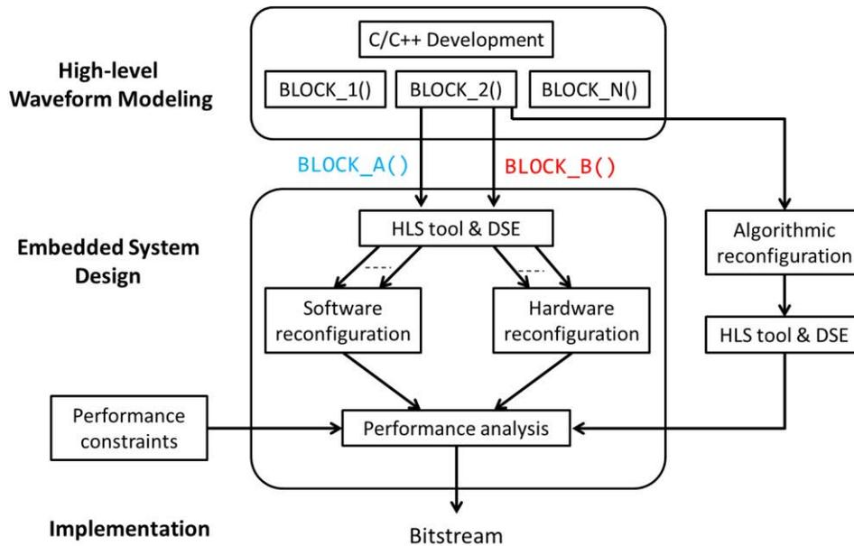
Figure 4.3 HLS-based design flow for a reconfigurable module using Software-Defined Reconfiguration.
