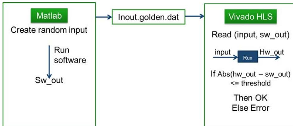
Figure 4.8 Example of code level verification in Vivado HLS based on a Matlab-provided reference.
