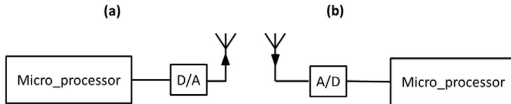
Figure 2.6 Ideal software-defined radio: (a) transmitter, (b) receiver.
