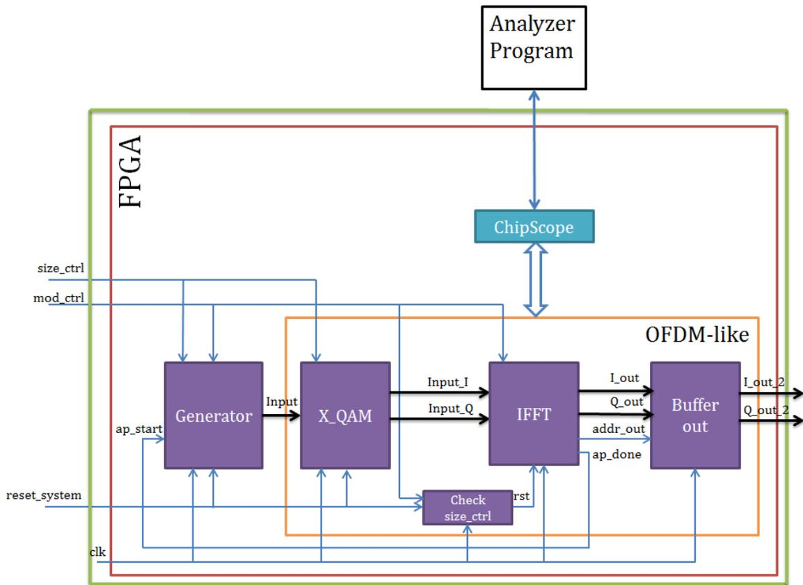
Figure 6.3 The architecture of the multi-mode FFT with software reconfiguration.
