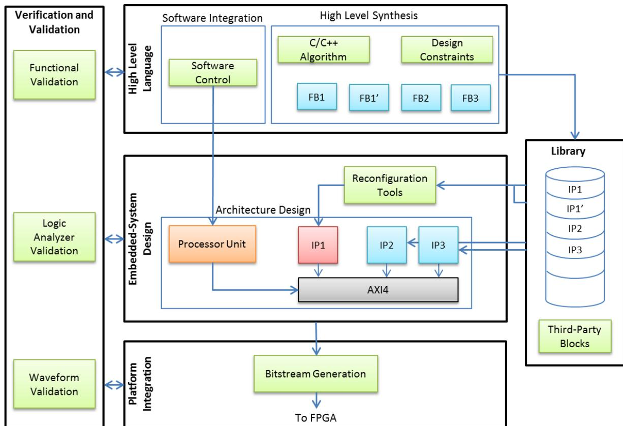
Figure 4.5 Proposed design flow for Flexible Radio using FPGA-based SDR.
