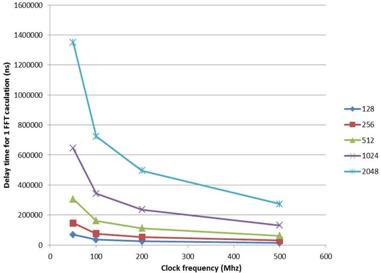
Figure 5.14 Time to compute 1 FFT vs frequency, U = 4
