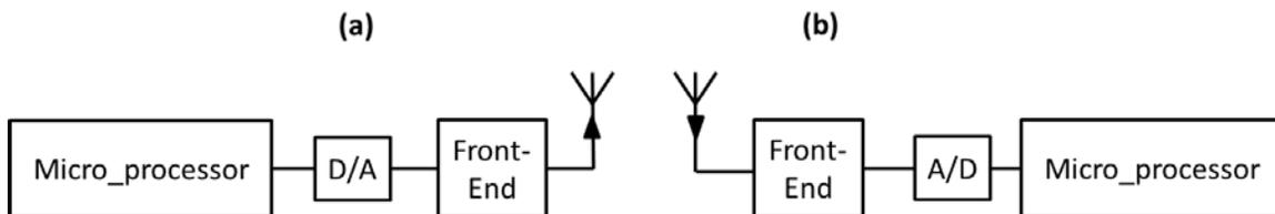
Figure 2.7 Realistic software-defined radio: (a) transmitter, (b) receiver.
