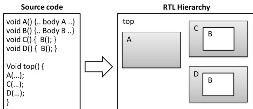
Figure 3.3 RTL hierarchy after HLS synthesis.
