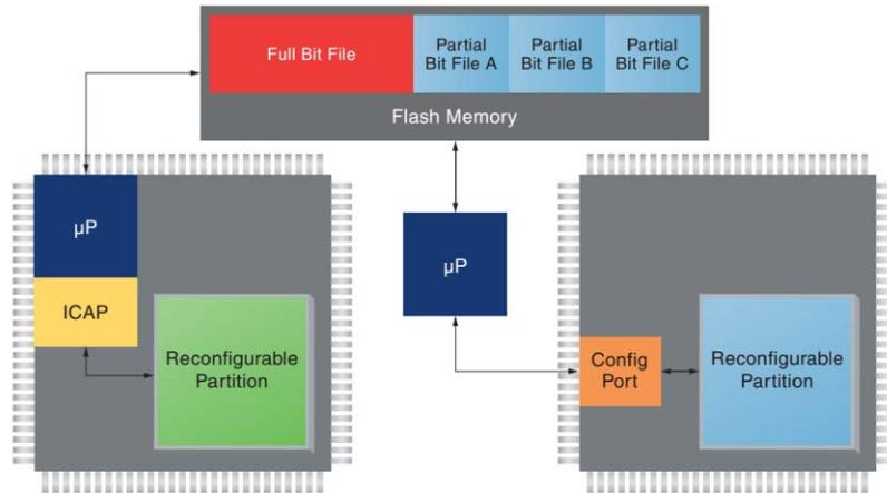
Figure 3.9 Two methods of delivering a partial bit file (with Xilinx devices) [69].
