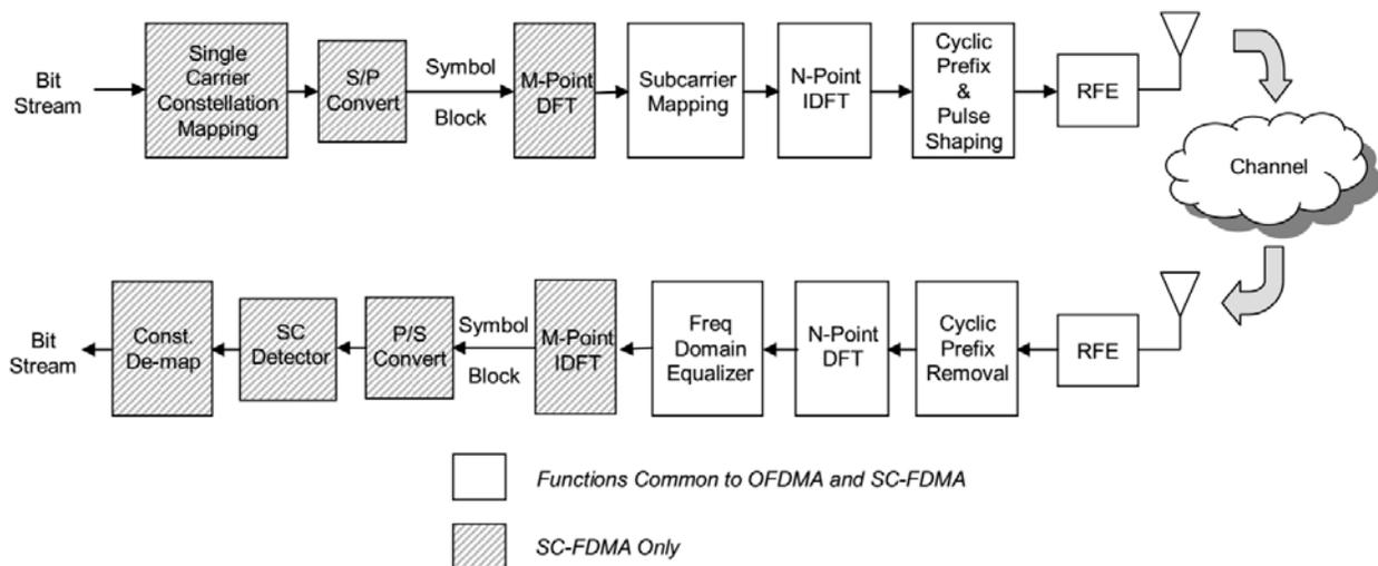
Figure 2.10 A basic SC-FDMA transmitter and receiver [29].
