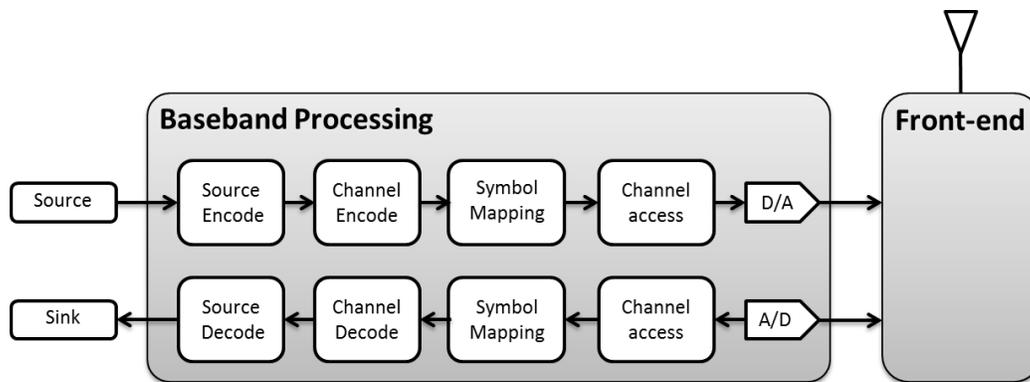
Figure 2.1 Digital radio system.
