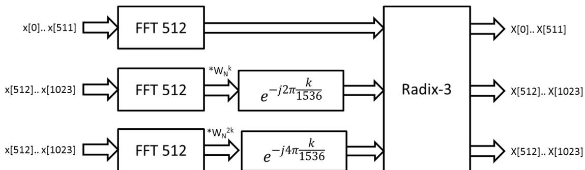
Figure 5.2 Structure of the 1536-point FFT
