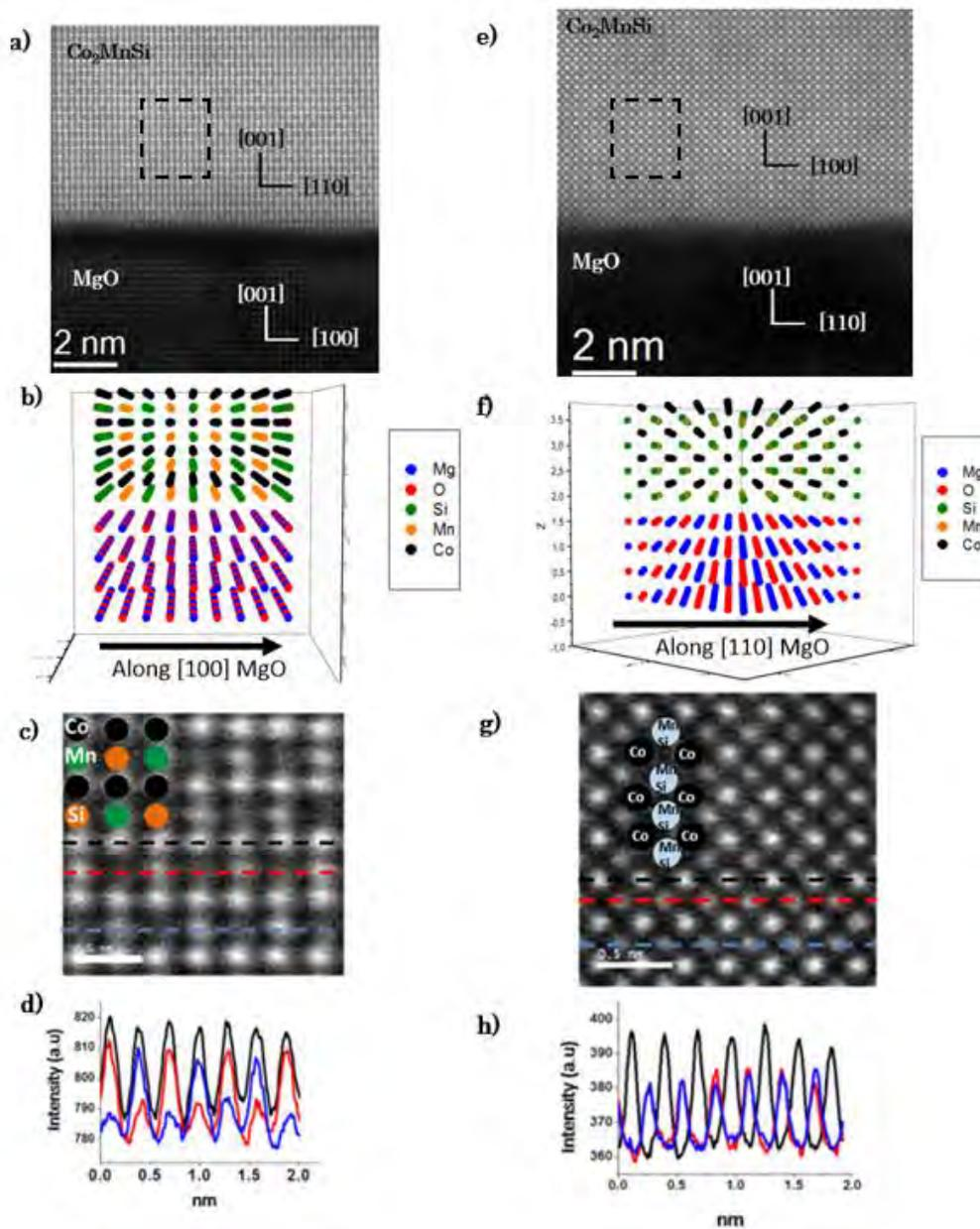
Figure 4.12: a) and e) are examples of HAADF-STEM of the reference sample N°3. b) and f) Sketched of the atomic arrangement in the different zone axis, considering the perfect  $L2_1$  structure. c) and g) Zoom corresponding to the black boxes in a) and e) showing the Co, Mn and Si positions. d) and h) Intensity profile for the dotted lines in c) and g).
