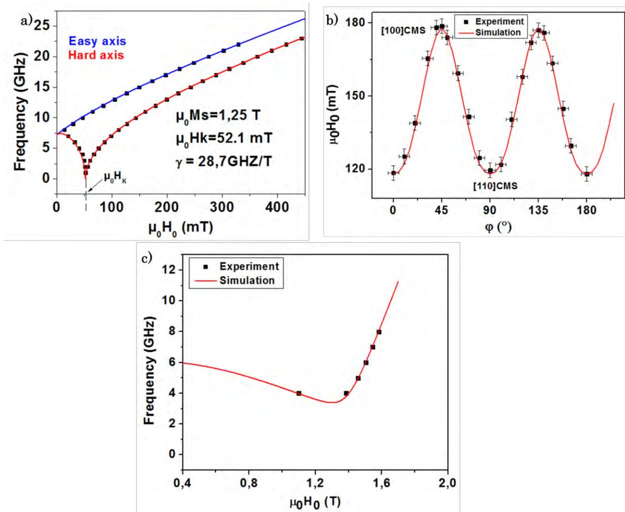
Figure 4.28: Example of measurements for the different experimental configurations used in this work. In a), dispersion relation  $f_{res}$  vs.  $\mu_0 H_0$  for in-plane measurements. The points corresponds to experimental data and the solid lines to the fit using equations 2.54 and 2.55. b), FMR angular measurements of  $\mu_0 H_0$  vs.  $\varphi$  at 13 GHz. c) Out-of-plane measurements of  $f_{res}$  vs.  $\mu_0 H_0$ . The line corresponds to the fit using equation 2.56.
