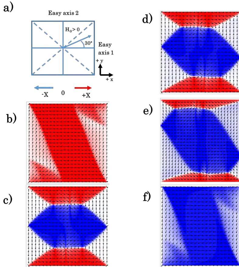
Figure 4.24: simulated switching mechanisms for fields applied at  $30^\circ$  from the easy axis 1. Switching from positive b) to negative f) applied field occurs through the growing of the central magnetic domain pointing in the  $-X$  direction as shown in c), d) and e).
