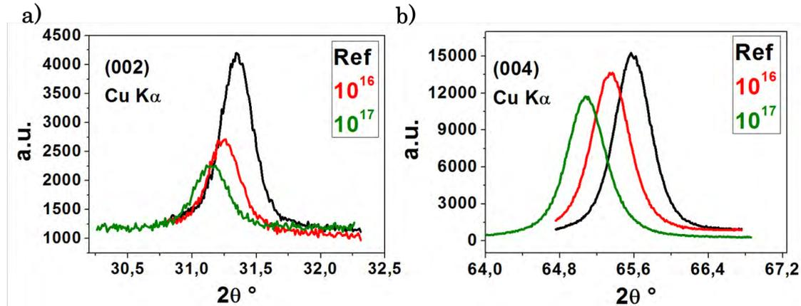
Figure 5.8: Evolution of 002 and 004 diffraction peaks as a function of irradiation fluence for the reference, irradiated at  $10^{16}$  and  $10^{17}$  ions/cm<sup>2</sup> of N°3 series samples performed by Cu source diffractometer.
