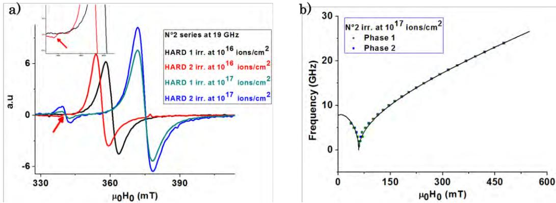
Figure 5.19: FMR absorption spectra comparison at 16 GHz of hard 1 and hard 2 axes of N°2 series samples irradiated at  $10^{16}$  and  $10^{17}$  ions/cm<sup>2</sup> in a). In b), the evolution of hard axes resonant peaks of N°2 sample irradiated at  $10^{17}$  ions/cm<sup>2</sup>.
