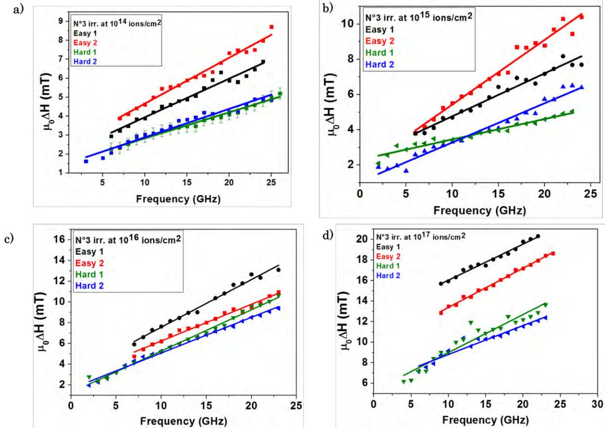
Figure 5.27:  $\Delta H$  vs.  $f_{res}$  measurements of N°3 series irradiated samples from  $10^{14}$  to  $10^{17}$  ions/cm<sup>2</sup> along the 4 axes directions shows clearly that the easy axes have higher  $\Delta H$  than hard axes.
