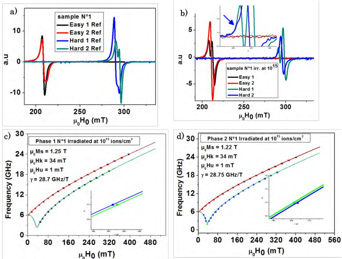
Figure 5.14: a) and b) presents the four easy and hard directions FMR spectra at 16 GHz of N°1 reference and irradiated at  $10^{15}$  ions/cm<sup>2</sup>. In c) and d)  $f_{res}$  vs.  $\mu_0 H_0$  curves for both phases of N°1 irradiated at  $10^{15}$  ions/cm<sup>2</sup>.
