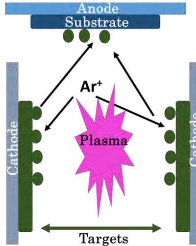
Figure 3.2: Graphical representation of the face to face configuration.
