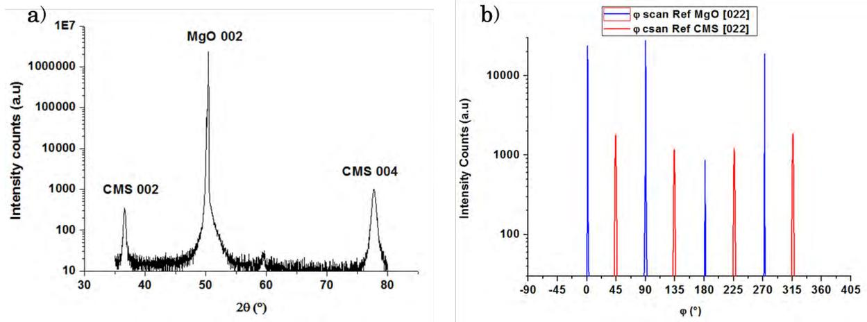
Figure 3.10: a)  $\theta - 2\theta$  X-ray diffraction scan showing the 002 and 004 peaks of CMS and 002 MgO peak. b)  $\varphi$  scan of the CMS with respect to the MgO substrate along the 022 direction clearly shows the  $45^\circ$  orientation.
