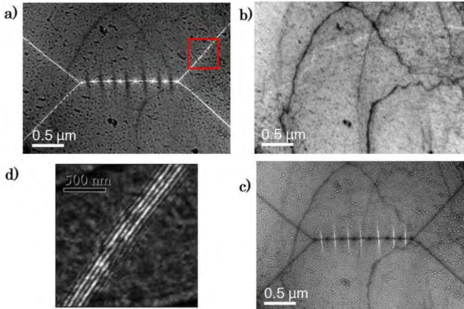
Figure 3.18: observation of domains walls in a) over-focus  $\Delta_z > 0$  and c) under-focus ( $\Delta_z < 0$ ). Image b) corresponds to the in-focus ( $\Delta_z = 0$ ) observation where no magnetic domains are observed. Figure d) shows the fringe spacing of the red box in a)
