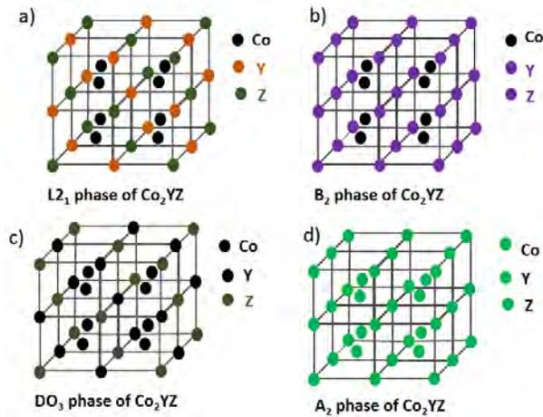
Figure 1.1: schematic presentation of  $\text{Co}_2\text{YZ}$  crystalline structure: a)  $L2_1$ , b)  $B_2$ , c)  $\text{D0}_3$  and  $\text{A}_2$  phases.
