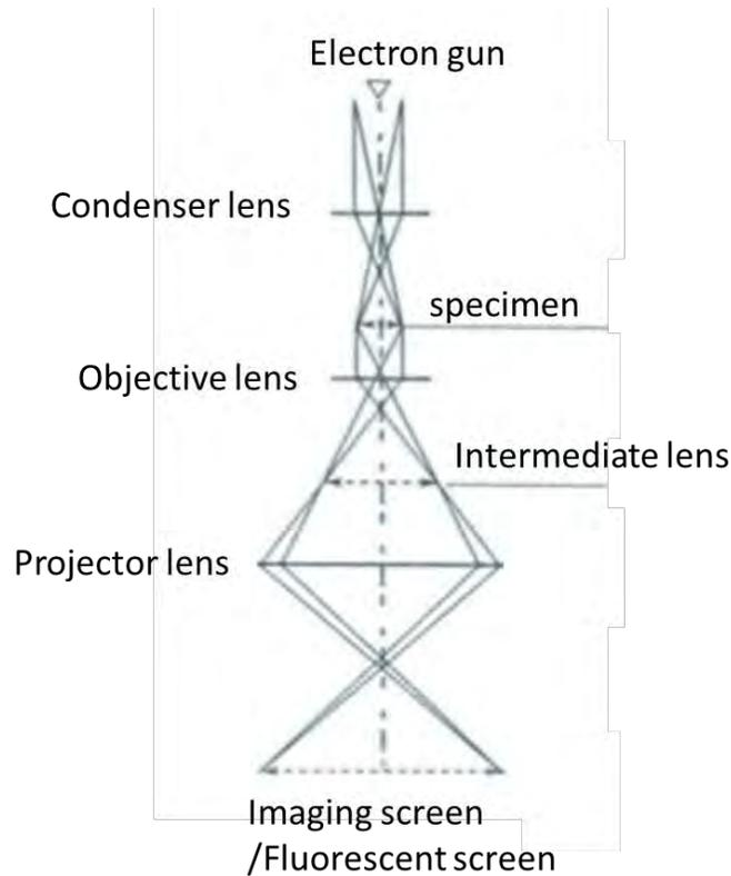
Figure 3.11: Schematic illustration of a transmission electron microscope.
