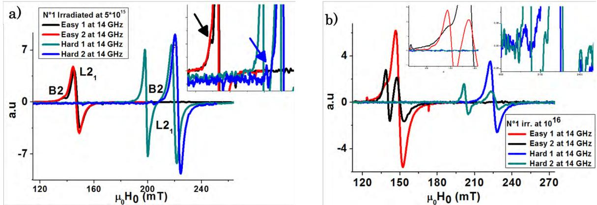
Figure 5.15: FMR absorption spectra obtained for the four easy and hard axes directions for a) N°1 irradiated at 5\*10<sup>15</sup> and b) N°1 irradiated for 10<sup>16</sup> ions/cm<sup>2</sup> fluence.
