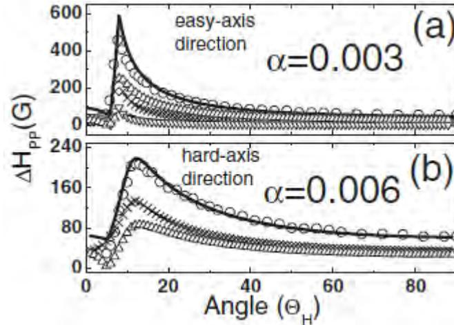
Figure 2.18: Angular dependence of linewidth  $\Delta H_{pp}$  of FMR spectra in out of-Plane geometry for  $\text{Co}_2\text{MnSi}$  film. Panels (a) and (b) respectively depict line-width variations versus out-of-plane angle  $\varphi_H$  in the easy- and hard-axis directions [48 Yilgin].
