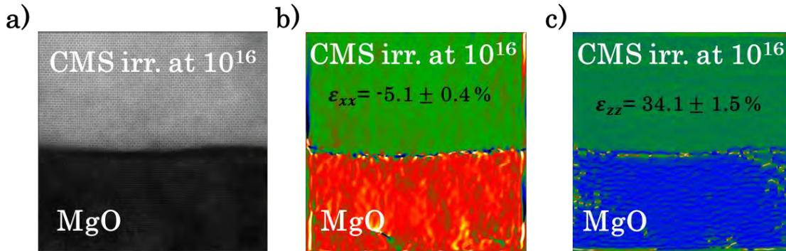
Figure 5.5: GPA analysis performed on sample N°1 irradiated at  $10^{16}$  ions/cm<sup>2</sup> shows the in-plane and out-of-plane deformation of  $-5.1 \pm 0.4$  and  $34.1 \pm 1.5$ , respectively.
