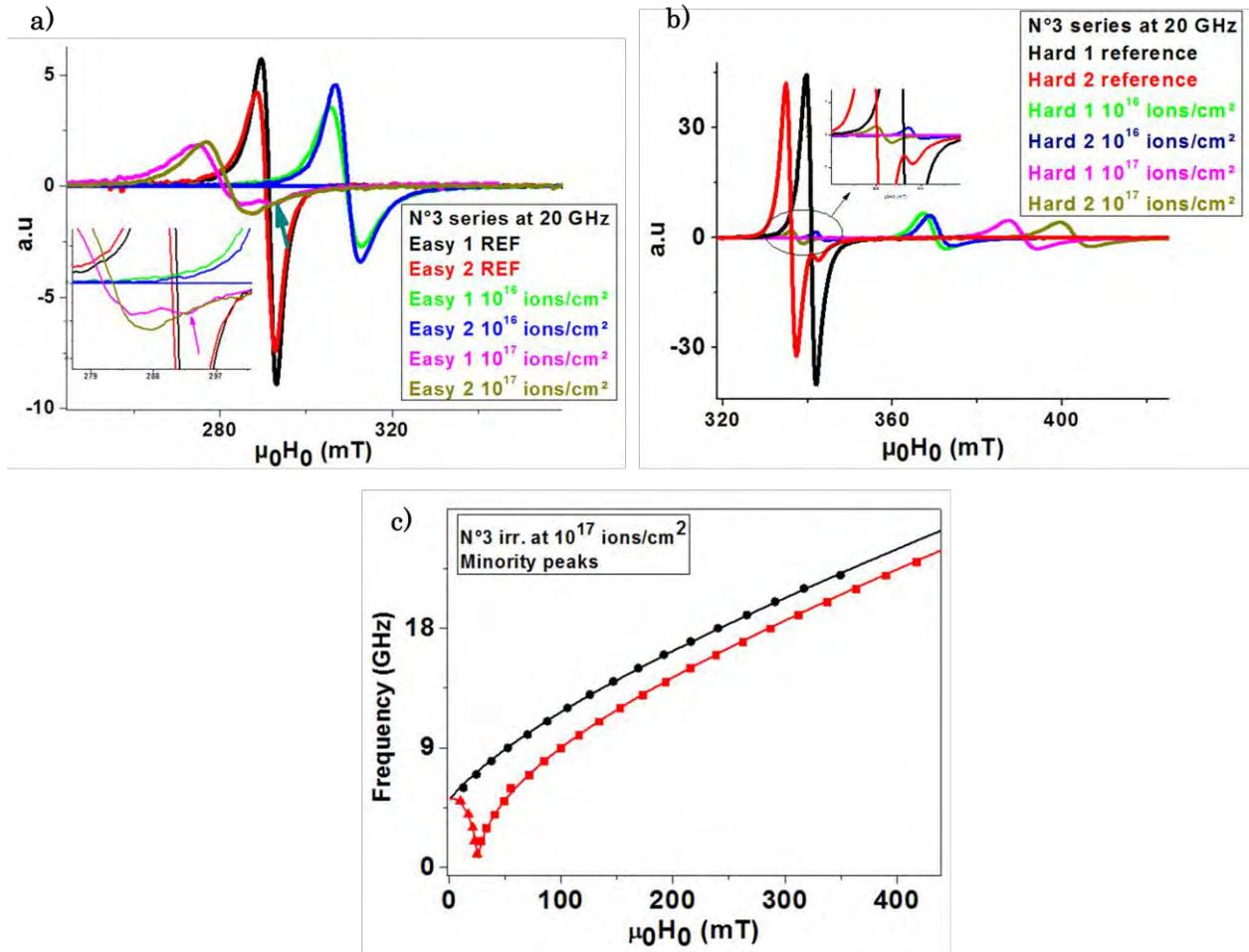
Figure 5.22: In a) and b) Comparison of the two easy and two hard axes respectively FMR absorption spectra at 20 GHz for  $\text{N}^3$  series for reference and irradiated samples at  $10^{16}$  and  $10^{17}$  ions/cm $^2$ . Figure c)  $f_{res}$  vs.  $\mu_0 H_0$  at lower magnetic fields (minority peaks) are traced for  $\text{N}^3$  sample irradiated at  $10^{17}$  ions/cm $^2$ .
