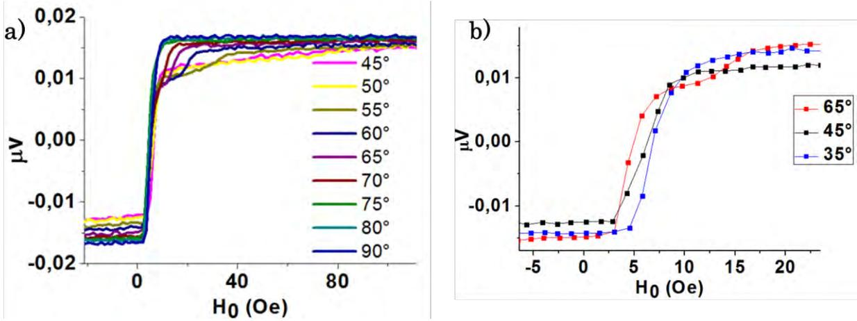
Figure 4.19: a) Evolution of the LMOKE component for sample N°1 at different angle  $\alpha$ . The field is swept from negative to positive fields. We clearly observe some “plateau” for angles between 50° and 70°. However, in b) the “plateaus” are absent for angles below 45°.
