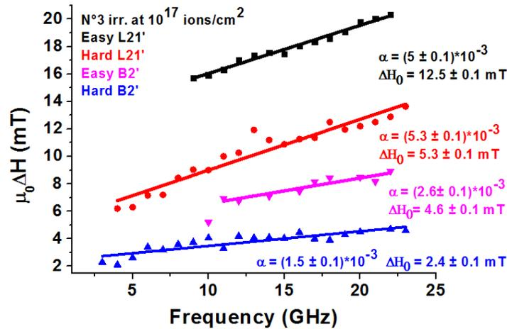
Figure 5.30: A comparison of the damping factor  $\alpha$  and the linewidth  $\Delta H_0$  for two crystal order of N°3 sample irradiated at  $10^{17}$  ions/cm<sup>2</sup>.
