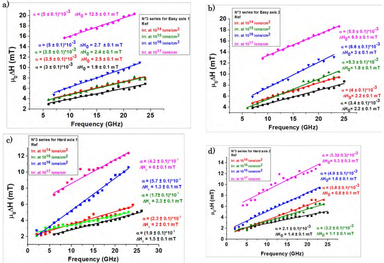
Figure 5.28: Evolution of damping coefficient and extrinsic linewidth contribution  $\Delta H_0$  as a function of irradiation dose from  $\Delta H$  vs.  $f_{res}$  measurements for N°3 series along the two easy and two hard axes.
