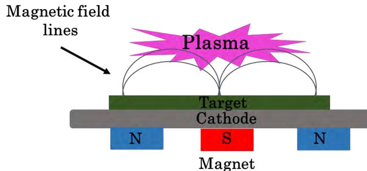
Figure 3.3: Graphical representation of magnetron sputtering configuration.
