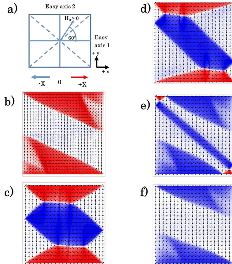
Figure 4.25: simulated switching mechanisms for an external field applied at  $60^\circ$  from the easy axis 1. The switching occurs through the propagation of the  $90^\circ$  domain walls in order to favor domains with magnetization pointing in the negative Y direction as shown in d) and e).
