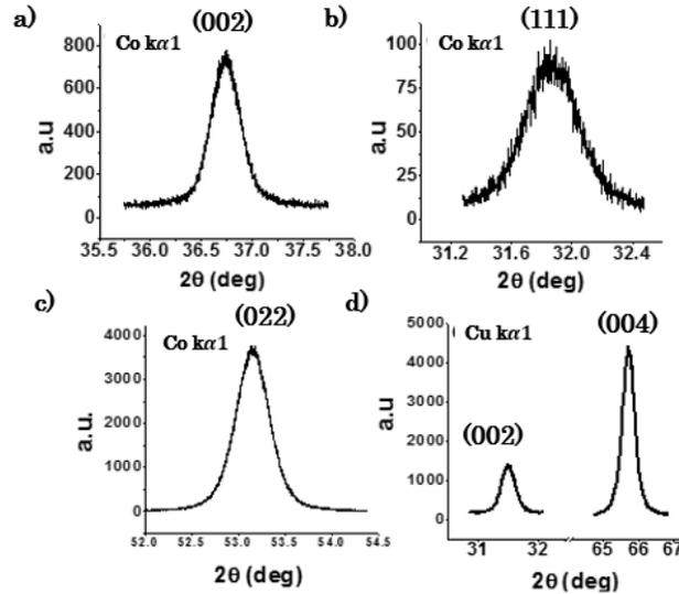
Figure 4.8:  $\theta - 2\theta$  scan for Co K $\alpha$ 1 and Cu K $\alpha$ 1 sources at different diffraction peaks. (Values in ordinates are raw values indicating the number of photons received by the optical detector. The correction factors are included in the calibration process performed prior to the experiment).
