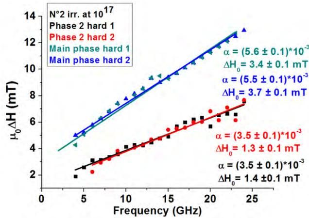
Figure 5.26: Comparison between the two phases in hard axis 1 and 2 for sample N°2 irradiated at  $10^{17}$  ions/cm<sup>2</sup> as the damping factor  $\alpha$  and extrinsic linewidth  $\Delta H_0$  is lower for the second phase than the main phase.
