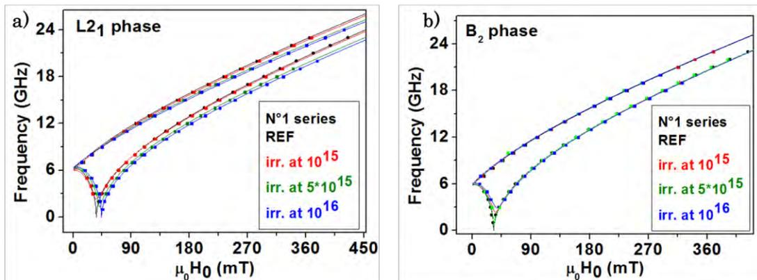
Figure 5.16: Evolution of the  $f_{res}$  vs.  $\mu_0 H_0$  curves for both phases of N°1 series. In a) shows the L<sub>21</sub> phase evolution as irradiation dose increases while in b) all curves have the same behavior and are identified for the B<sub>2</sub> phase.
