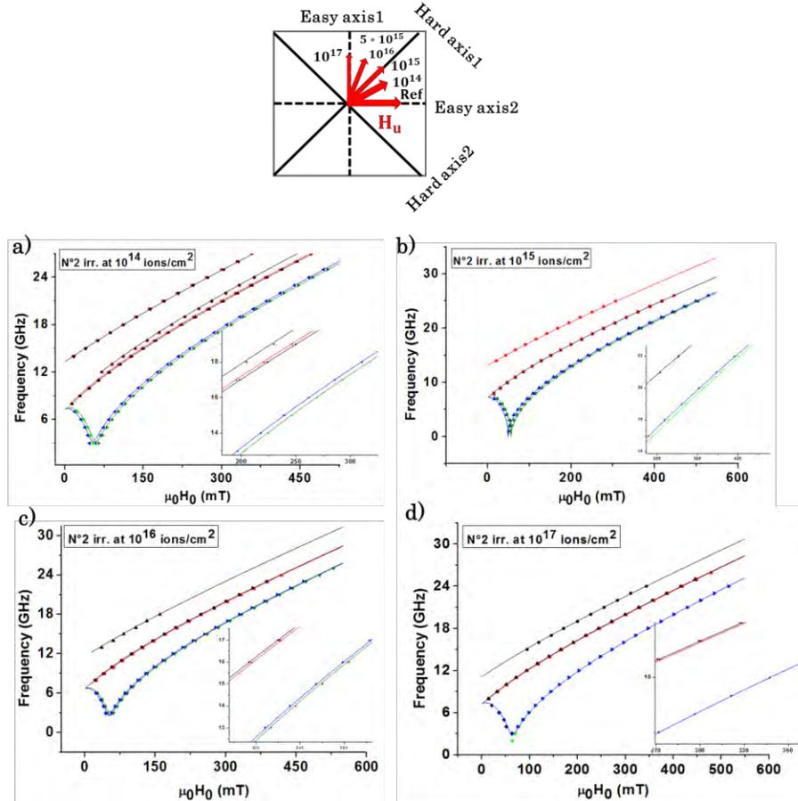
Figure 5.18:  $f_{res}$  vs.  $H_0$  curves for N°2 series irradiated samples at  $10^{14}$ ,  $10^{15}$ ,  $10^{16}$  and  $10^{17}$  ions/cm<sup>2</sup> in a), b) c) and d) respectively. The box shows the uniaxial anisotropy rotation from Easy axis 2 for reference sample to Easy axis 1 at  $10^{17}$  ions/cm<sup>2</sup>.
