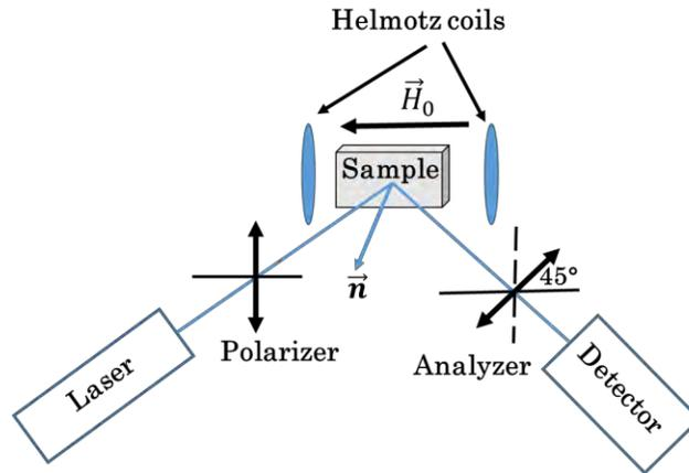
Figure 3.21: schematic illustration of MOKE experimental set-up.
