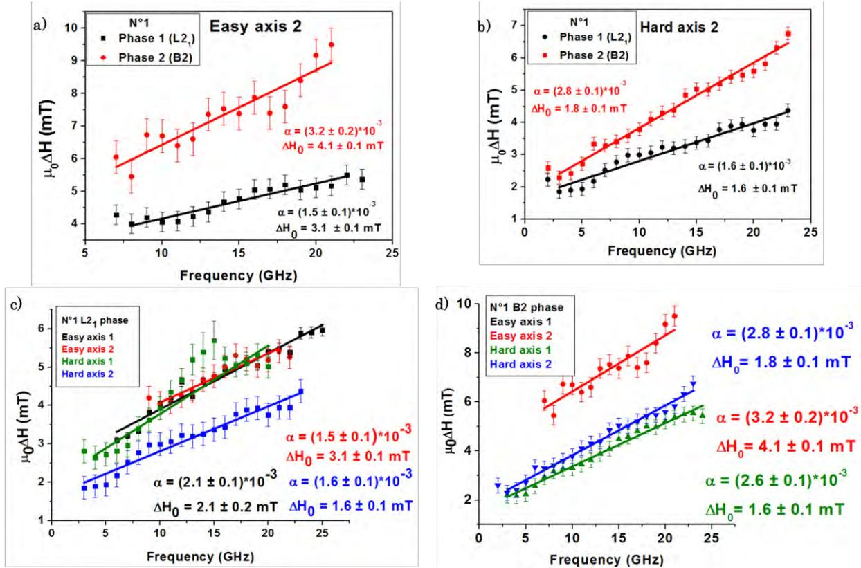
Figure 4.35: line width measurements as a function of the applied frequency along easy and hard axes for the two observed L2<sub>1</sub> and B2 phases of sample N°1. In a) and b) the two modes are distinguished for easy 2 and hard 2 axes, respectively. While in c) and d), line width values ( $\Delta H$ ) of L2<sub>1</sub> and B2 phases and their linear fit are traced for each easy and hard axis showing their corresponding damping coefficient  $\alpha$  and  $\Delta H_0$ .
