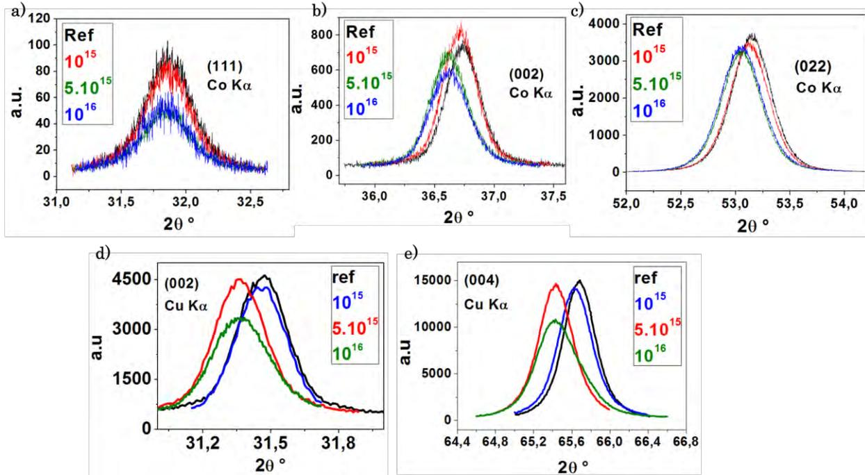
Figure 5.4: X-ray diffraction  $2\theta$  scan for reference and 3 irradiated samples of N°1 for Co and Cu diffractometer sources. a), b) and c) represents the 111,002 and 022 peaks acquired by Co source. d) and e) presents the 002 and 004 peaks acquired by Cu source.
