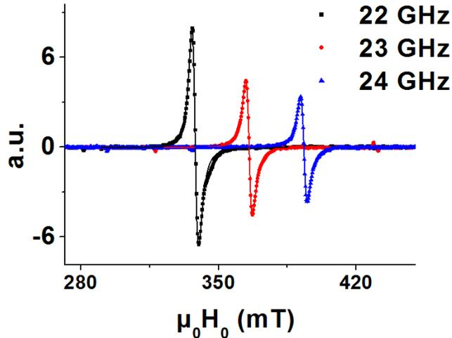
Figure 4.27: A typical FMR spectra at different frequencies.
