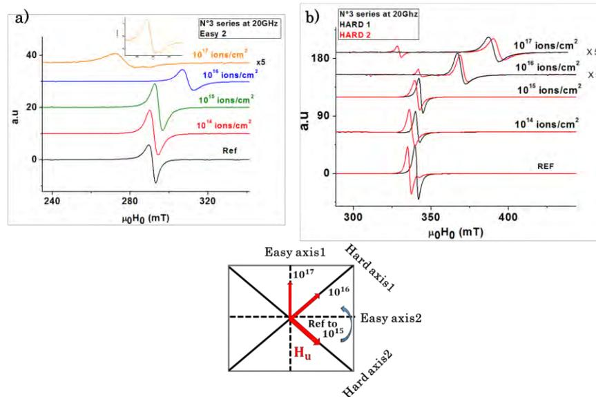
Figure 5.20: Absorption spectra as a function of magnetic external field  $\mu_0 H_0$  for N°3 series samples at 20 GHz along the two easy and the two hard axes in a) and b) respectively. The box shows the uniaxial anisotropy rotation from hard axis 2 for reference sample to easy axis 1 at  $10^{17}$  ions/cm<sup>2</sup>
