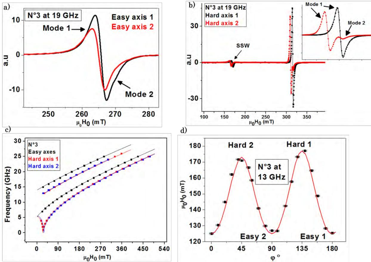
Figure 4.34: FMR absorption spectra for CMS N°3 for in-plane configuration along a) easy axes and b) hard axes at 19 GHz. c)  $f_{res}$  vs.  $H_0$  for in-plane SSW and uniform mode configurations. In d), angular dependence of resonance fields at 13 GHz.
