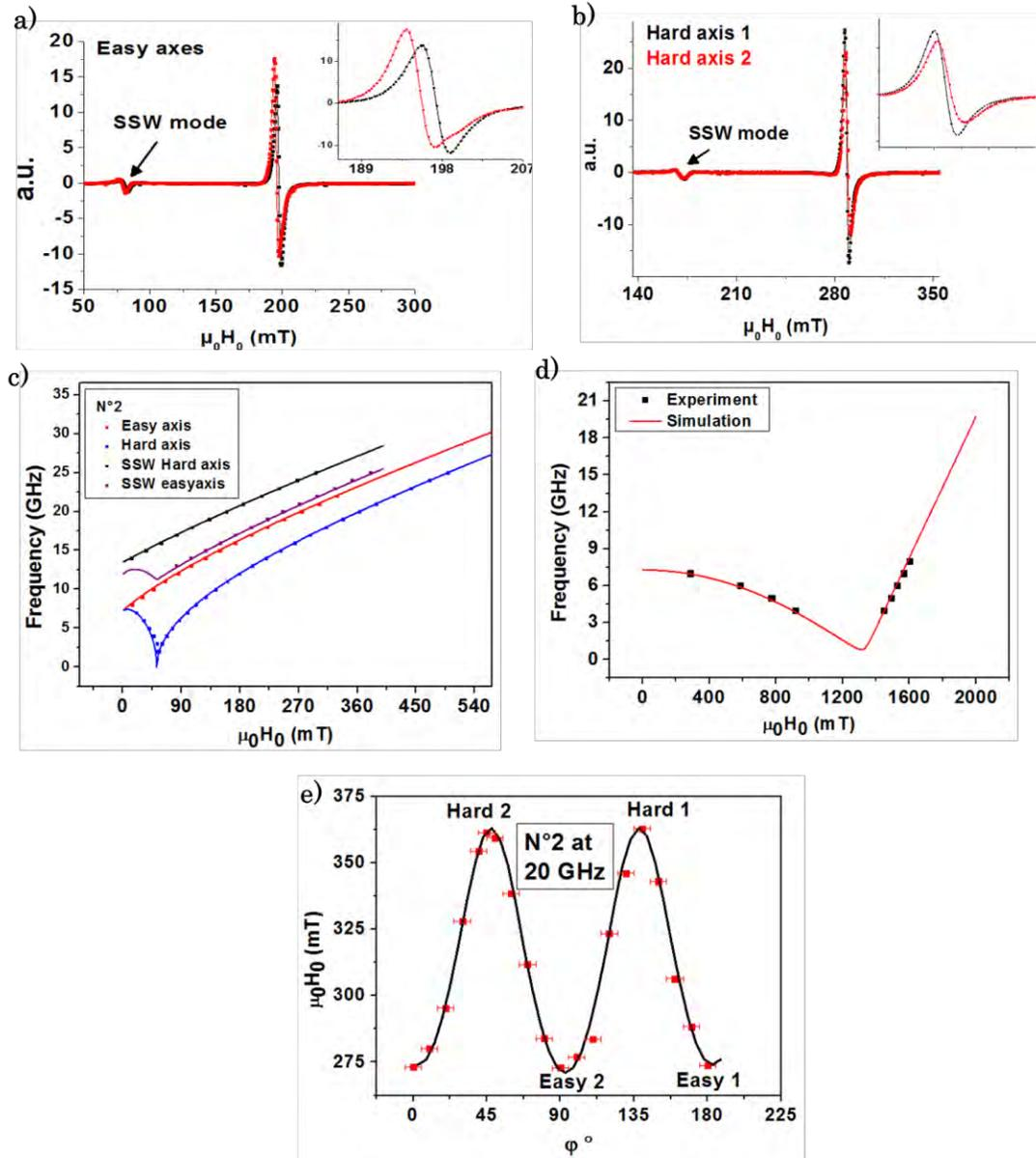
Figure 4.33: FMR absorption spectra for CMS N°2 for in-plane configuration along a) easy axes at 18 GHz and b) hard axes at 17 GHz.  $f_{res}$  vs  $\mu_0 H_0$  for c) in-plane and d) out-of-plane configurations. In e), angular dependence of resonance fields at 20 GHz.
