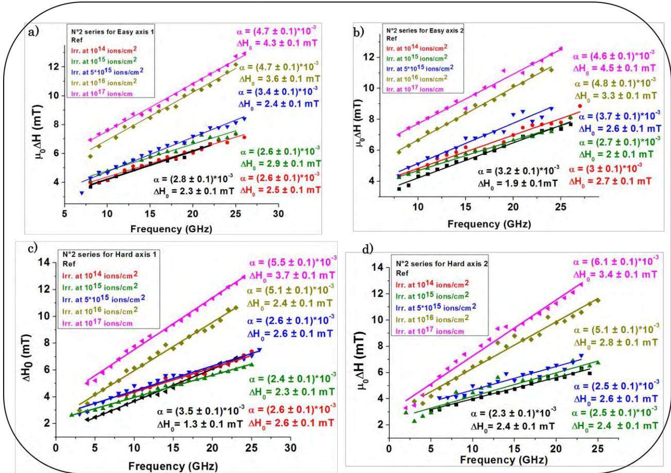
Figure 5.25: Evolution of damping coefficient and extrinsic linewidth contribution  $\Delta H_0$  as a function of irradiation dose from  $\Delta H$  vs.  $f_{res}$  measurements for N°2 series along the two easy and two hard axes.
