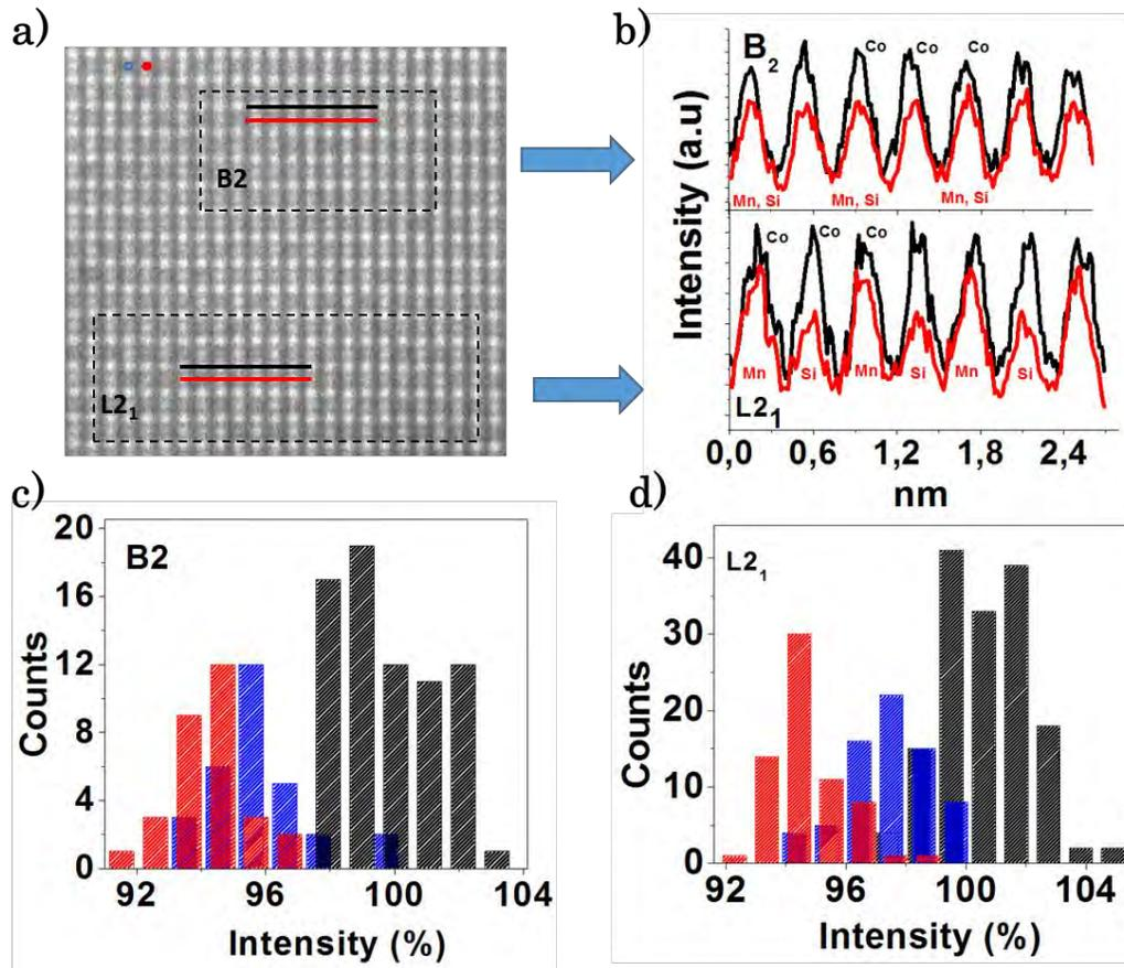
Figure 5.7: effect of irradiation on the atomic order seen by HAADF-STEM image in a) with a profile intensity on two selected lines indicating L2<sub>1</sub> and B2 regions in b). Statistics were done on selected areas to distinguish the two phases in c) and d).
