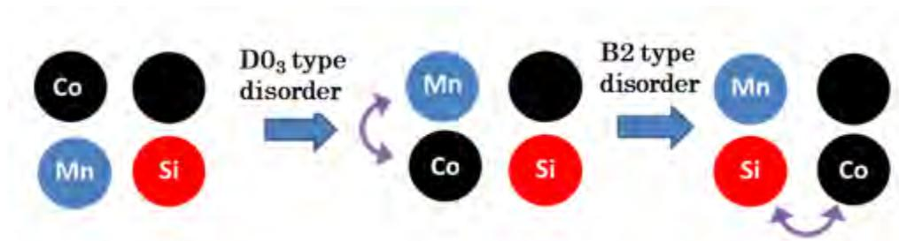
Figure 5.10: proposed scenario of the irradiation effect on CMS samples starting from L2<sub>1</sub> phase to D0<sub>3</sub> (Co-Mn disorder) and then a B'2 (Co-Si disorder) phase.
