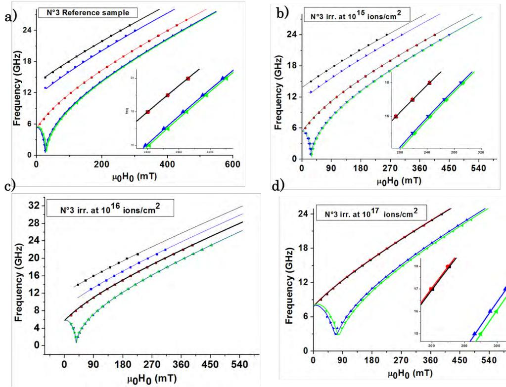
Figure 5.21:  $f_{res}$  vs.  $\mu_0 H_0$  curves for N<sup>o</sup>3 series for reference in a) and irradiated samples at  $10^{15}$ ,  $10^{16}$  and  $10^{17}$  ions/cm<sup>2</sup> in b), c) and d) respectively.
