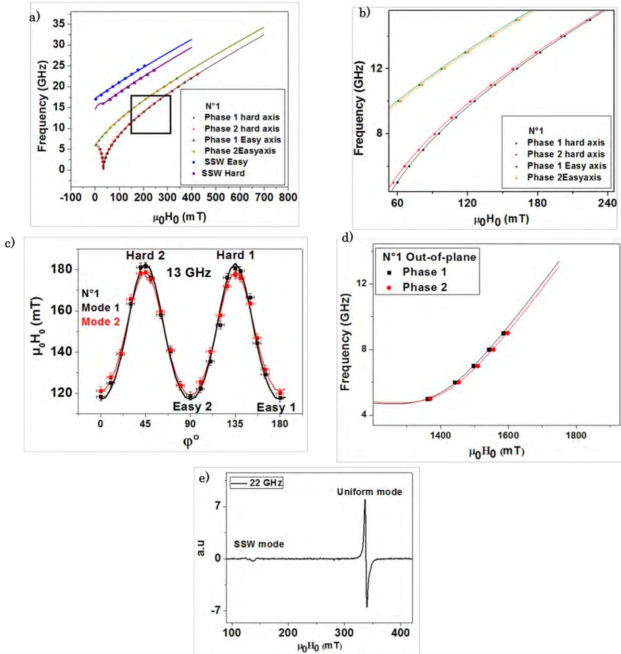
Figure 4.31: Dispersion relation  $f_{res}$  vs.  $\mu_0 H_0$  in CMS N°1 for a) in-plane and d) out-of-plane configuration. Figure b) corresponds to a zoom on the two modes for the black box in a). c) Angular dependence of the resonance field at 13 GHz. e) FMR signal at 22 GHz in the easy direction showing both the FMR and SSW modes.
