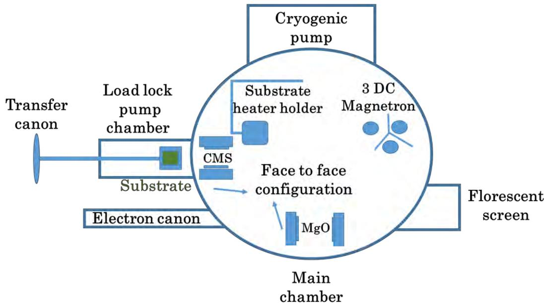
Figure 3.4: graphical representation of PLASSYS sputtering at CEMES.
