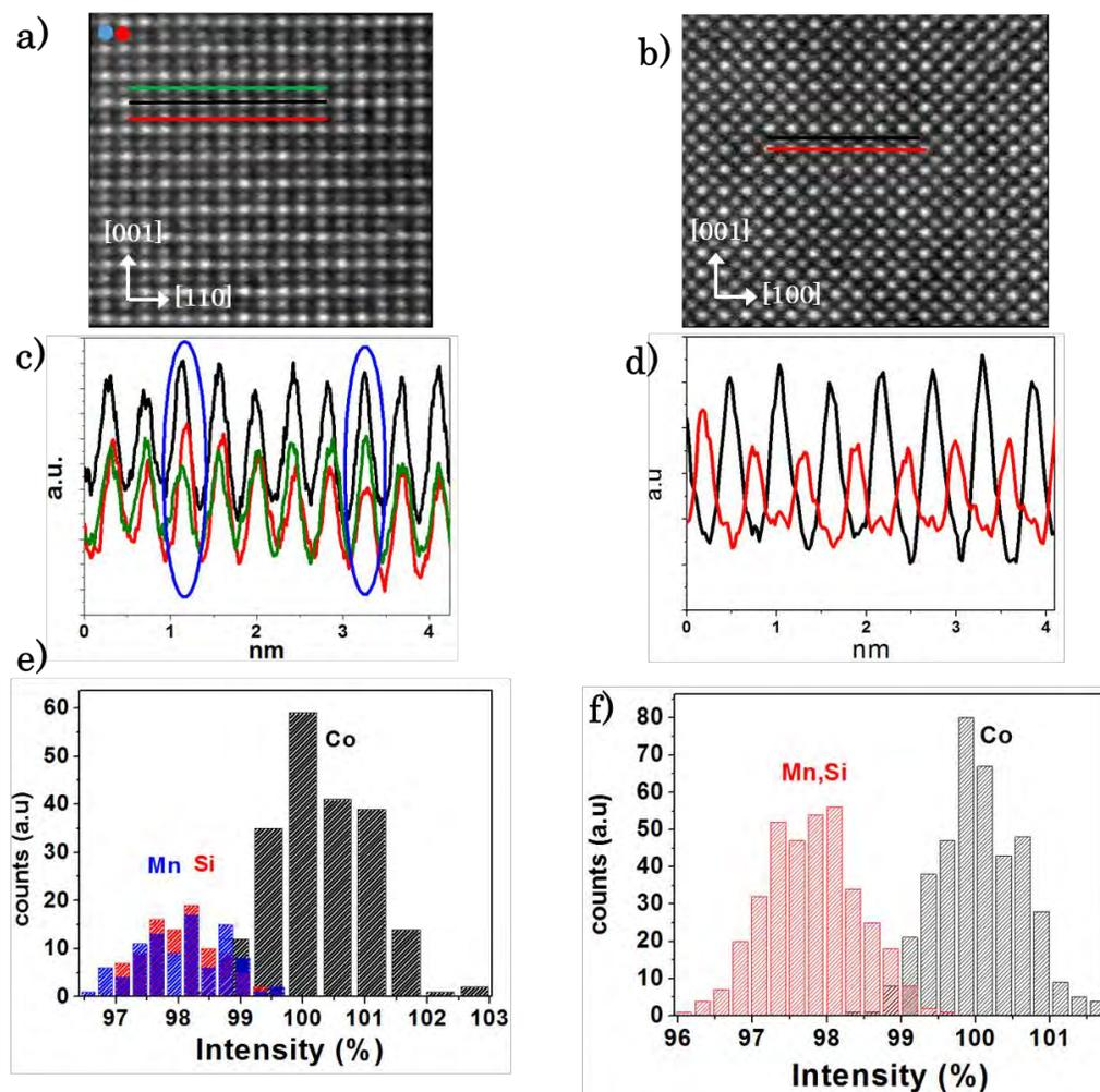
Figure 5.9: HAADF-STEM has been performed on the sample irradiated at  $10^{17}$  ions/cm<sup>2</sup> for the series N°3 along [110] and [100] CMS directions in a) and b) respectively. Intensity profiles in c) show some remaining L2<sub>1</sub> regions in blue circles while in d) Mn and Si are indistinguishable. Statistics in e) and f) show that Co has higher intensities than Mn and Si.
