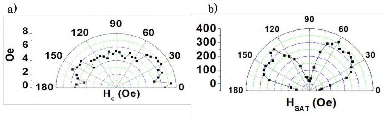
Figure 4.18: Sample N°1 twofold symmetry for a) coercive and b) saturation fields from 0° to 180°.
