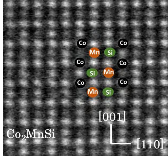
Figure 3.15: An HAADF-STEM image of CMS layer where the atomic columns of Co, Mn Si are clearly shown.
