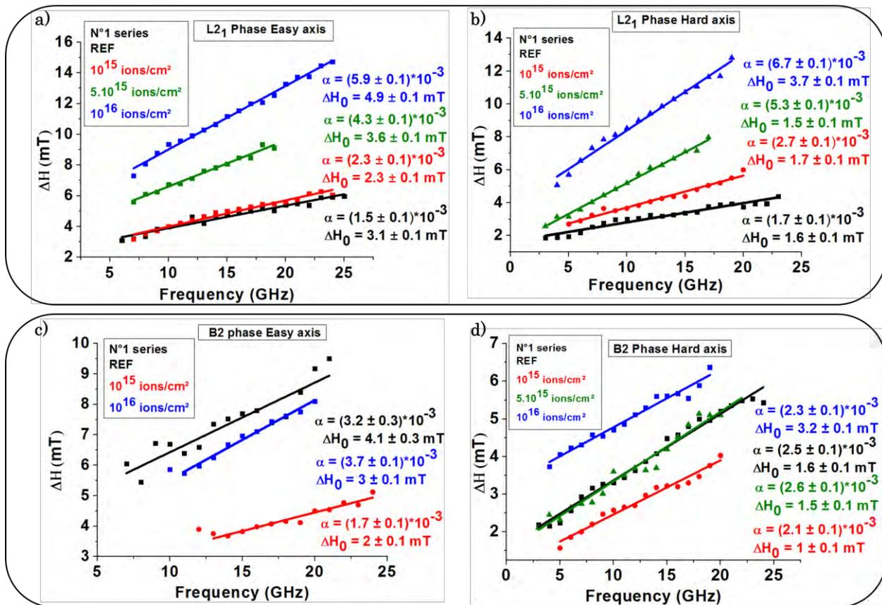
Figure 5.23: Evolution of linewidth measurements  $\Delta H$  vs.  $f_{res}$  for N°1 series for both L2<sub>1</sub> and B2 phases. In a) and b) we can see the evolution of damping coefficient and extrinsic linewidth contribution  $\Delta H_0$  for L2<sub>1</sub> phase as irradiation dose increases, while in c) and d) the damping factor is kept almost constant for B2 phase with an increase in  $\Delta H_0$ .
