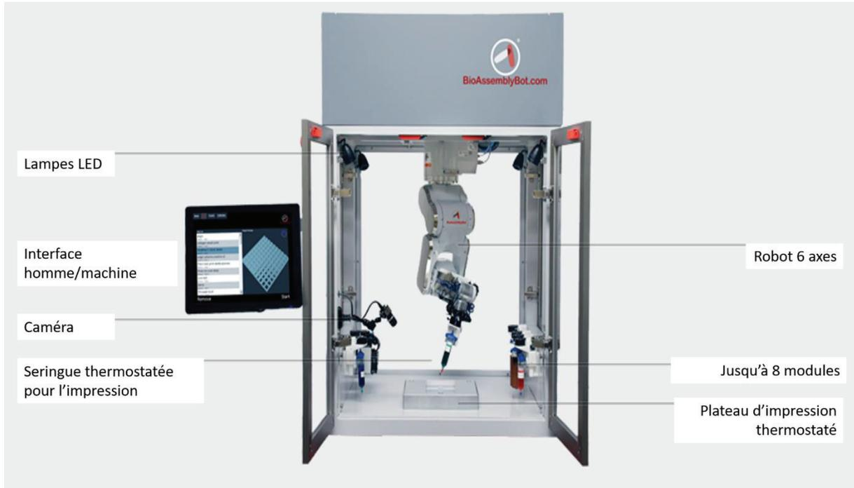
Figure 83. Photo de la machine BioAssemblyBot® (<https://lifesciences.solutions/bioassemblybot/>)
