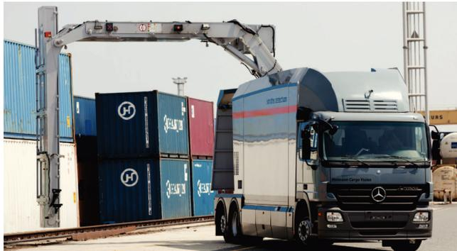
(b) scanning arm deployed
