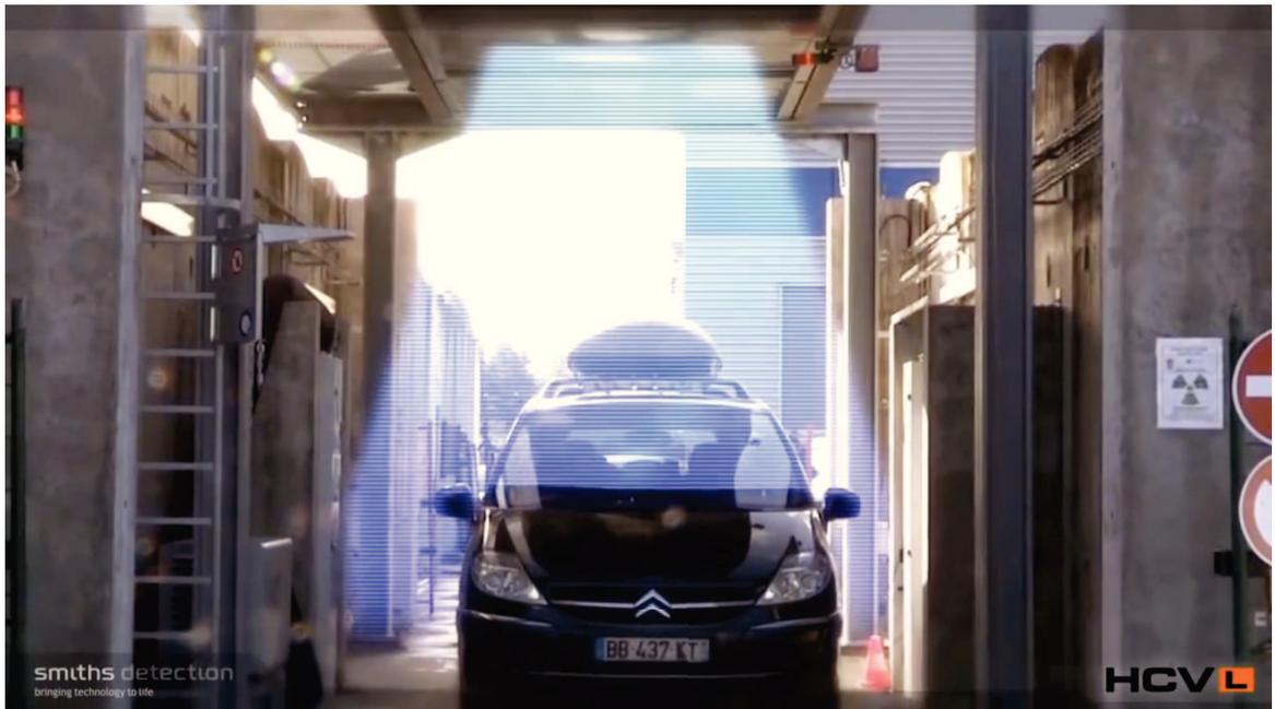
Figure 6.37 – Illustration of X-ray beam during scanning.
