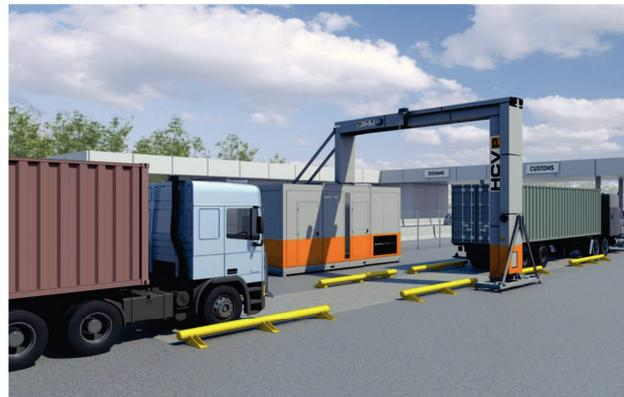
Figure 18 – HCVP scanning machine
