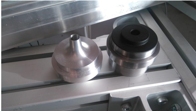
Figure 2. 1: evaluated nozzles. Thin lip (left) and thick lip (right).
