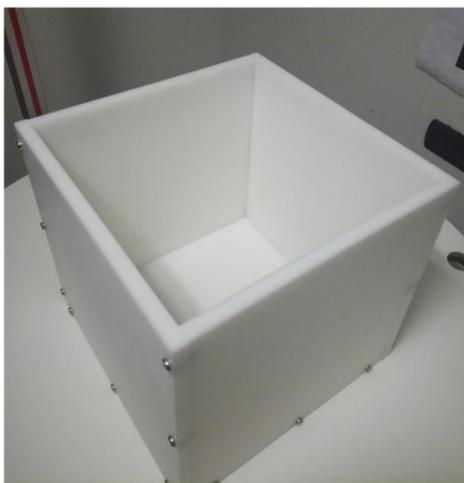
Figure 5-6: Open Field apparatus for mice.
