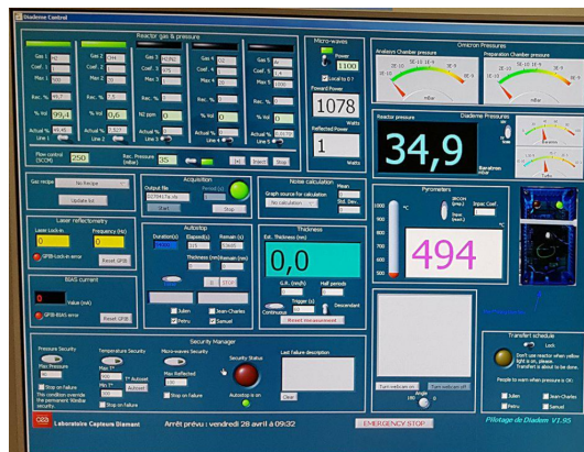
Figure 3.4: Diadem system user interface LabView
