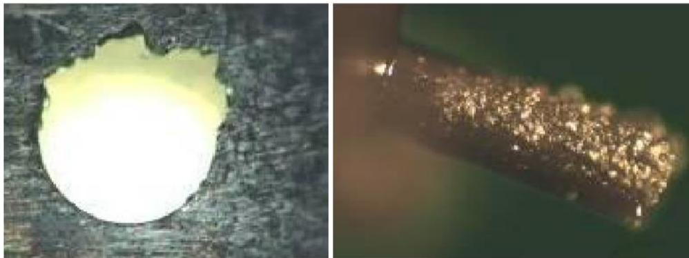
Figure 3.6. Images provided by Delphi Diesel Systems UK and showing cavitation erosion at the exit of an injection hole together with an impression made of the inside of the damage hole in a Diesel fuel injector (taken from Grant agreement of CaFE project grant no. 642536).
