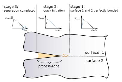
FIGURE 1.9: Schematic illustration of the different stages of crack initiation and growth in cohesive zone model.
