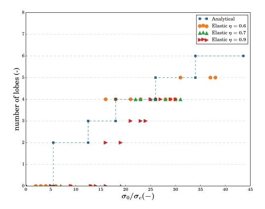
FIGURE 4.27: Number of lobes *n* resulting from the destabilization process of an initially circular blister at different loading ratios  $\frac{\sigma_0}{\sigma_c}$ . Numerical results are obtained using cohesive zone model for a mode mixity dependence parameters of 0.9, 0.7 and 0.6 and Poisson's ratio of the film  $\nu = 0.44$ . The analytical results are obtained for  $\eta = 1$  and  $\nu = \frac{1}{3}$ .
