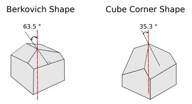
FIGURE 2.5: Berkovich and cube corner indenter tip geometries
