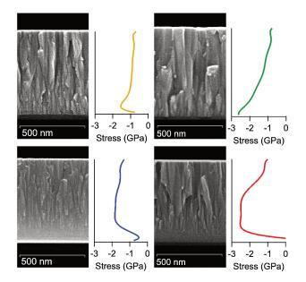
FIGURE 3.21: FEG-SEM images showing the influence of substrate potential and oxygen doping on the microstructure of molybdenum thin films. Top left: Mo at floating potential, top right: Mo at -75 V, bottom left: Mo with 2 sccm of  $O_2$  at floating potential and bottom right:Mo with 2 sccm of  $O_2$  at -75 V. [29]
