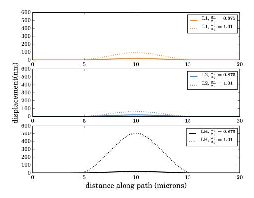
FIGURE 3.18: Straight blisters' profiles for different elastic-plastic behaviours: L1 (Ludwik: $\sigma_y = 400 \text{ MPa}, K = 50 \text{ MPa}, n = 0.25$ ), L2: (Ludwik: $\sigma_y = 400 \text{ MPa}, K = 130 \text{ MPa}, n = 0.25$ ), LH (Linear hardening: $\sigma_y = 400 \text{ MPa}, K = 80 \text{ MPa}$ )
