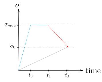
FIGURE 4.20: Different loading histories: Linear loading (red) and tri-linear loading (blue)
