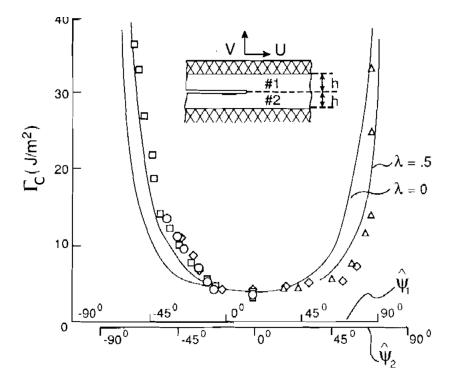
FIGURE 1.8: Data from [65] for an epoxy  $\sharp 1$  / glass  $\sharp 2$  interface:  $\psi_1$  axis is obtained using  $l_1 = 12,7mm$  and  $\psi_2$  using  $l_2 = 127\mu m$ . The solid curves represent  $G_c(\psi_2)$ as given by equation 1.35
