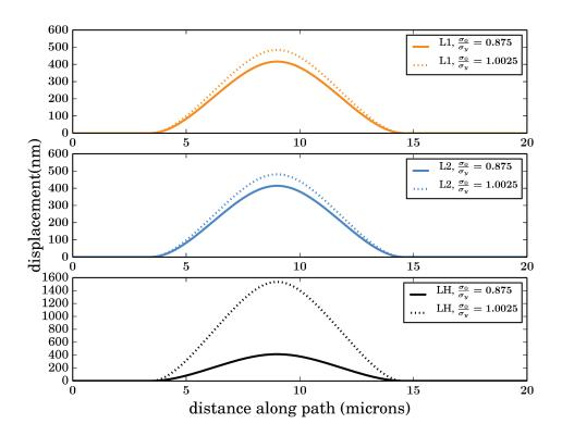
FIGURE 3.15: Straight blisters' profiles for different elastic-plastic behaviours: L1 (Ludwik: $\sigma_y = 800 \text{ MPa}, K = 50 \text{ MPa}, n = 0.25$ ), L2: (Ludwik: $\sigma_y = 800 \text{ MPa}, K = 130 \text{ MPa}, n = 0.25$ ), LH (Linear hardening: $\sigma_y = 800 \text{ MPa}, K = 80 \text{ MPa}$ )
