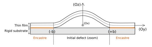
FIGURE 3.1: Mechanical model for the buckling of a thin film.
