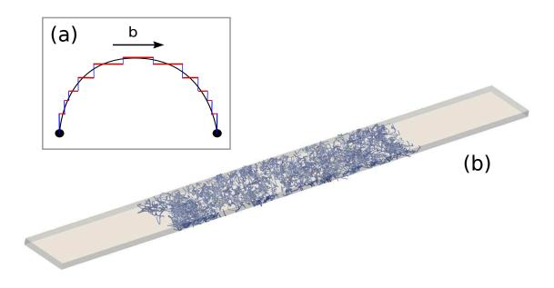
FIGURE 4.30: (a) Edge-screw discretization of a dislocation line. Blue lines are edge dislocations and red lines are screw dislocations. (b) Coupling finite element method with discrete dislocation dynamics. The Frank–Read sources are distributed randomly in a rectangular single crystal that represents the thin film. Different colours represent different slip systems.
