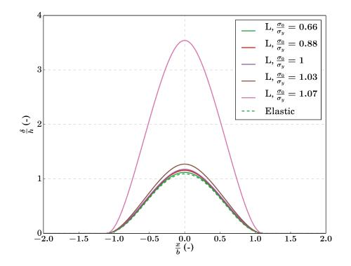
FIGURE 3.5: Comparison between elastic and elastic-plastic straight blisters' profiles. The y-axes represents normalized deflection  $\frac{\delta}{h}$ , where  $\delta$  is the out-of-plane displacement of the film and h the thickness of the film (fixed). All cases are subject to the same residual stresses ( $\sigma_0 = 800$  MPa). The elastic-plastic behaviour is described by Ludwik hardening with the following fixed parameters K = 130 MPa, n = 0.25. We vary  $\sigma_y$
