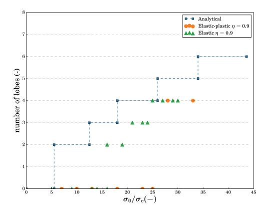
FIGURE 4.29: Number of lobes n resulting from the destabilization process of an initially circular blister at different loading ratios  $\frac{\sigma_0}{\sigma_c}$  for an elastic and an elastic-plastic thin film. Numerical results are obtained using cohesive zone model for a mode mixity dependence parameters of 0.9 and Poisson's ratio of the film  $\nu = 0.44$ . The analytical results are obtained for  $\eta = 1$  and  $\nu = \frac{1}{3}$ .
