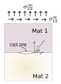
FIGURE 1.5: Crack at an interface between two materials
