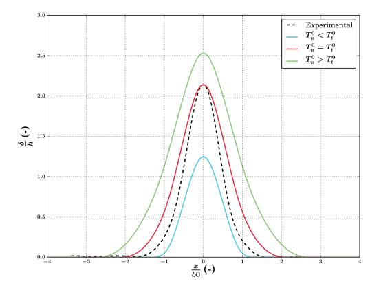
FIGURE 4.18: Comparison between the profiles obtained for different values of maximum normal and shear stress  $T_n^0$  and  $T_t^0$ . The cases  $T_n^0 < T_t^0$ ,  $T_n^0 = T_t^0$  and  $T_n^0 > T_t^0$ correspond respectively to the following couples  $(T_n^0, T_t^0)$ : (60, 120), (60, 60) and (60, 40) MPa
