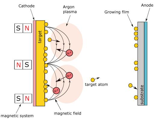
FIGURE 2.1: Scheme of magnetron sputtering device
