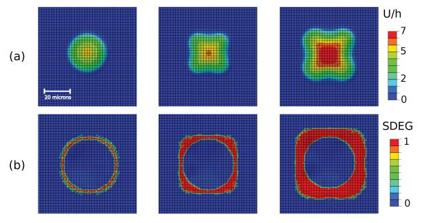
FIGURE 4.25: Various stages of growth of a circular defect submitted to constant loading  $\sigma_0$ . The row (a) features the evolution of the normalized out-of-plane displacement  $\frac{U}{h}$  and the row (b) shows the corresponding degradation variable of the interface SGEG. SDEG=0 means that the interface is intact, SDEG=1 means that the fracture is completed and intermediate SDEG values corresponding to an ongoing fracture process.
