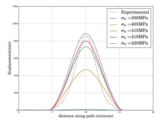
FIGURE 3.23: Comparison between the experimental blister's profile and elasticplastic numerical model results in the case of straight blister (Ludwik strain hardening  $\sigma_y = 400 \text{ MPa}, K = 50 \text{ MPa}, n = 0.25$ ) for different  $\sigma_0$  values
