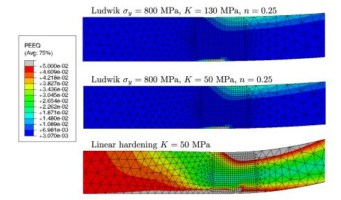
FIGURE 3.16: Effect of the hardening law on plastic strain at the base of straight blisters ( $\sigma_0 = 802 \text{ MPa}$ )
