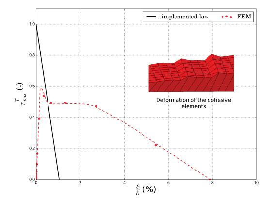
FIGURE 4.9: This graph features the implemented cohesive law and the corresponding cohesive response obtained via FEM implicit analysis with a time step  $\tau = 0.1$ and a viscous relaxation time of  $\mu = 1.e-4$ . The graph also shows the state of cohesive elements in contact with the distorted 3D elements showed in figure 4.8.
