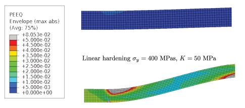
FIGURE 3.17: Effect of the hardening law on plastic strain at the base of straight blisters ( $\sigma_0 = 404 \text{ MPa}$ )
