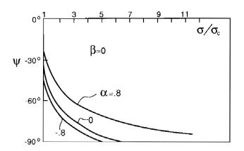
FIGURE 1.14: Mixed mode angle at the crack tip as a function of the normalized stress  $\sigma/\sigma_c$ , from [48]
