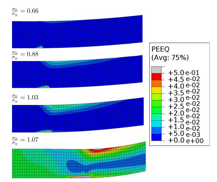
FIGURE 3.6: Equivalent plastic strain mapping for the cases  $\frac{\sigma_0}{\sigma_y} = 0.66$ ,  $\frac{\sigma_0}{\sigma_y} = 0.88$ and  $\frac{\sigma_0}{\sigma_y} = 1.03$ . All cases are subject to the same residual stresses ( $\sigma_0 = 800$  MPa). The elastic-plastic behaviour is described by Ludwik hardening with the following fixed parameters K = 130 MPa, n = 0.25. We vary  $\sigma_y$
