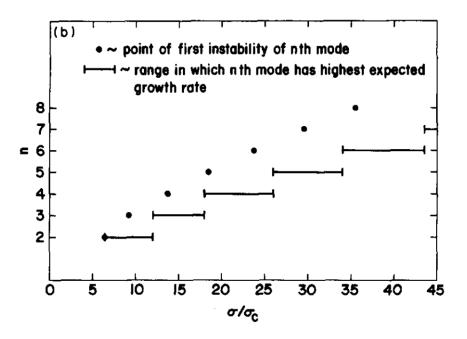
FIGURE 1.18: destabilization of circular blister: Number of lobes as a function of the loading ratio  $\frac{\sigma_0}{\sigma_c}$  for  $\eta = 1$  and  $\nu = \frac{1}{3}$
