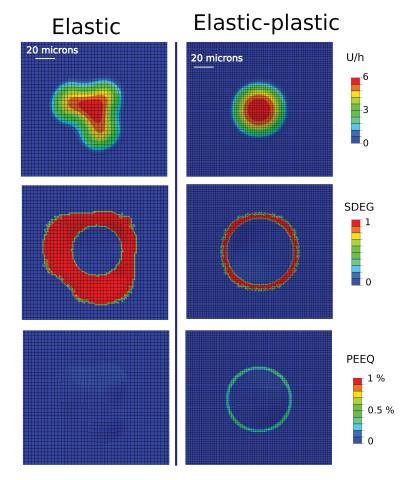
FIGURE 4.28: Various stages of growth of a circular blister submitted to constant load  $\sigma_0$  in the case of an elastic and an elastic-plastic behaviour ( $\sigma_y = 800 \text{ MPa}, K = 50 \text{ MPa}, n = 0.25$ ). Each case features the mapping of the normalized out-of-plane displacement  $\frac{U}{h}$  at the equilibrium point, the corresponding degradation variable of the interface SGEG and the distribution of the plastic deformation.
