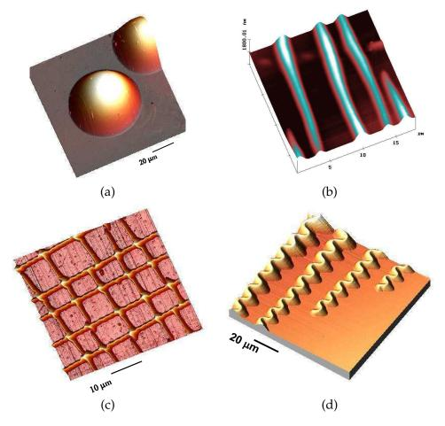
FIGURE 1: Examples of buckling delamination structures. (a) Circular blisters – Au(630 nm) on Si. (b) Straight sided blisters – stainless steel. (c) Intersecting blisters – Stainless steel on polycarbonate. (d) Telephone cords blisters –  $Y_2O_3(30-50nm)$  on GaAs. (Courtesy of C. Coupeau et col., Institut P')
