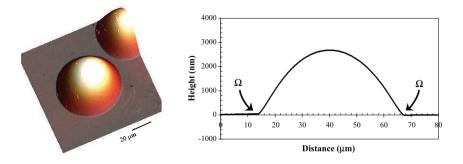
FIGURE 2.4: Buckling structure observed in gold film, 630 nm thick, deposited on silicon substrate. A marked bending  $\Omega$  of the buckling structure is observed at the base of the circular blister.[18]
