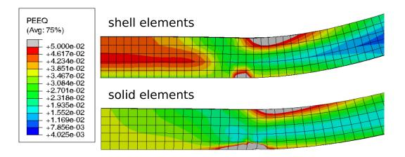
FIGURE A.3: Equivalent plastic strain mapping obtained in the case of solid and shell elements for the same  $\sigma_0 = 850$  MPa and the same hardening law (Ludwik  $\sigma_y = 800$  MPa, K = 130 MPa, n = 0.25)
