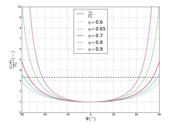
FIGURE 4.4: Interfacial toughness ratio  $\frac{G_c(\Psi)}{G_{I_c}}$  as function of the mode mixity angle  $\Psi$  for several values of  $\eta$
