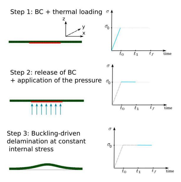
FIGURE 4.22: Scheme of the steps applied to ensure the occurrence of bucklingdriven delamination at constant load  $\sigma_0$ . In the first step, the bottom nodes of the defect area of the film are blocked along the z - axis and the thermal loading of the film is performed. In the  $2^{nd}$  step, the defect nodes are released and a small pressure is applied ton trigger buckling. In the final step, buckling-driven delamination occurs at constant loading.
