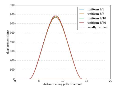
FIGURE A.4: Effect of mesh refinement on the buckling profile of straight blisters. The profiles are obtained for the same ratio  $\frac{\sigma_0}{\sigma_y} = 1.03$ , the same hardening law (Ludwik  $\sigma_y = 800$  MPa, K = 130 MPa, n = 0.25) and different solid element sizes. (see figure A.5)
