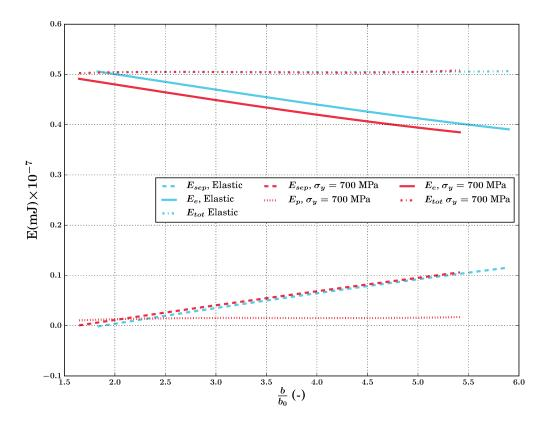
FIGURE 4.14: Energy as a function of the normalized position of the crack front  $\frac{o}{b_0}$ , where b is the half width of the blister during propagation and  $b_0$  the half width of the initial defect.  $E_e$  represents the elastic energy,  $E_p$  the plastic energy and  $E_{sep}$  the energy used to fracture the interface. The figure feature two cases: purely elastic thin film ( $\sigma_0 = 700$  MPa) and elastic-plastic thin film ( $\sigma_0 = \sigma_y = 700$  MPa).
