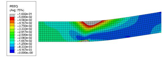
FIGURE 3.9: Equivalent plastic mapping of the case ( $\frac{\sigma_0}{\sigma_c} = 0.5$ ,  $\frac{\sigma_0}{\sigma_u} = 1.05$ )
