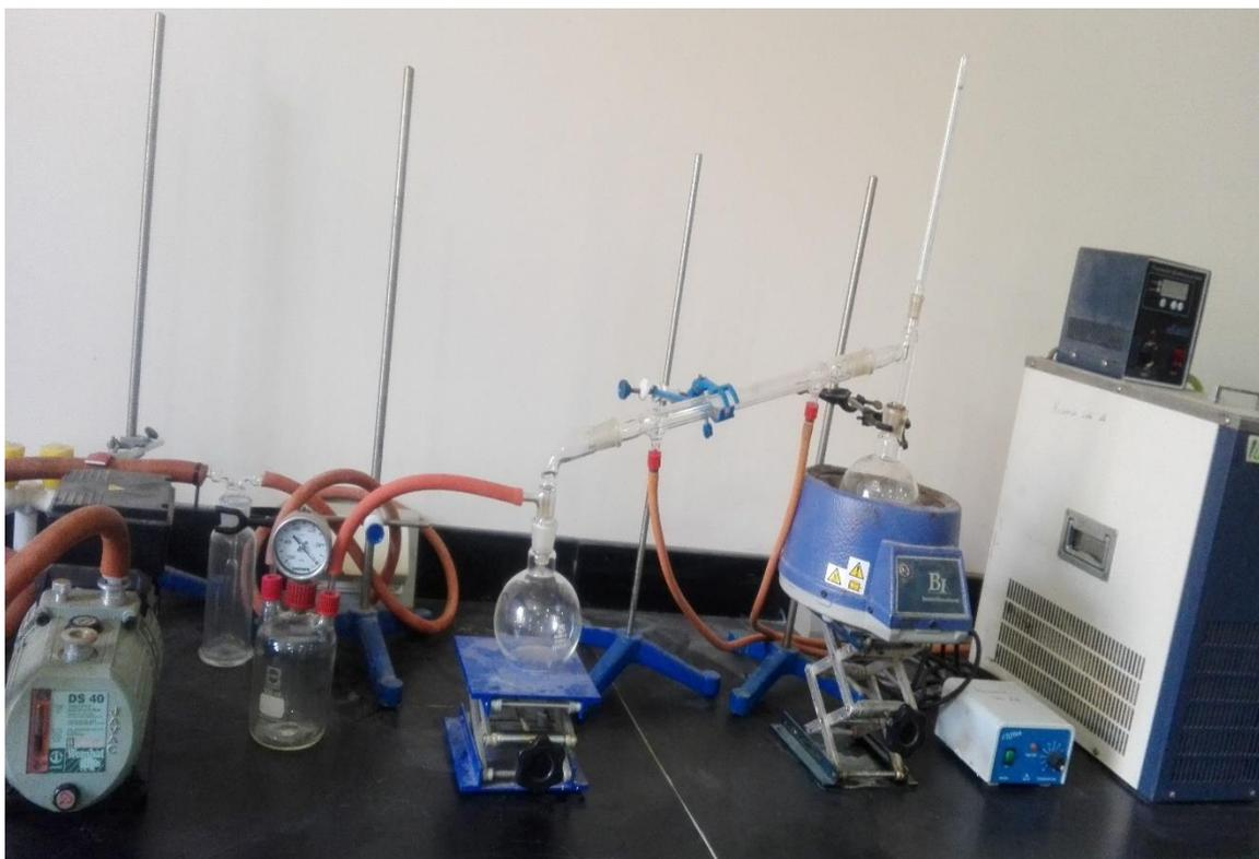
*Figure 3-13. Vacuum Distillation Apparatus*
