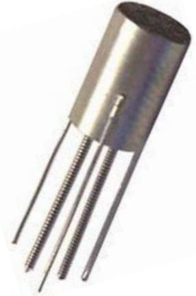
**Figure 104: Photo of an alkaline Emitter used in the ion gun.**
