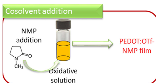
Figure II.5. From the synthesis of PEDOT:OTf and PEDOT:OTf-NMP to its treatment with sulfuric acid. a) Synthesis of PEDOT:OTf. b) Synthesis of PEDOT:OTf-NMP. After the addition of EDOT, all previous steps are the same. c) Treatment with sulfuric acid: the obtained PEDOT:OTf (with or without a co-solvent) is dipped into diluted sulfuric acid.
