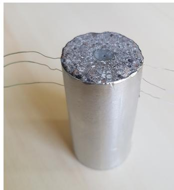
**Figure 4.8:** Specimen wrapped with adhesive aluminium tape
