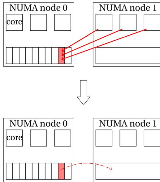
Figure 2.7: Carrefour migration heuristic: when a hot page is accessed only by remote cores of the same node (top part of the diagram), this hot page is migrated on the accessing NUMA node
