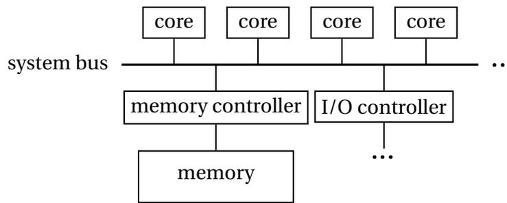
Figure 2.1: The architectural view of a multicore architecture
