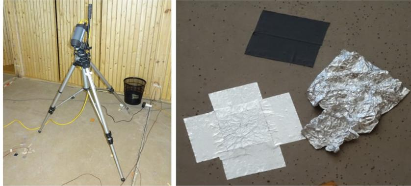
Figure 2.12: Experimental set-up for infrared measurements. On the left-hand side: Infrared camera. On the right-hand side: A fully crumbled aluminum foil (isotropic and diffuse reflector), a black foil placed on the concrete-slab surface (reference).
