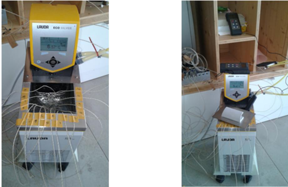
Figure A.6: Thermocouples inside the thermostatic Bath.
