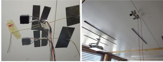
Figure 2.9: Image of the measurement zone on the ceiling surface.
