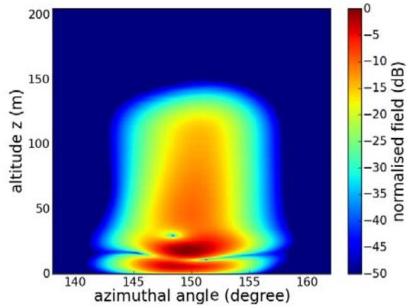
(a) Normalized final electric field (dB) using the proposed 3D method
