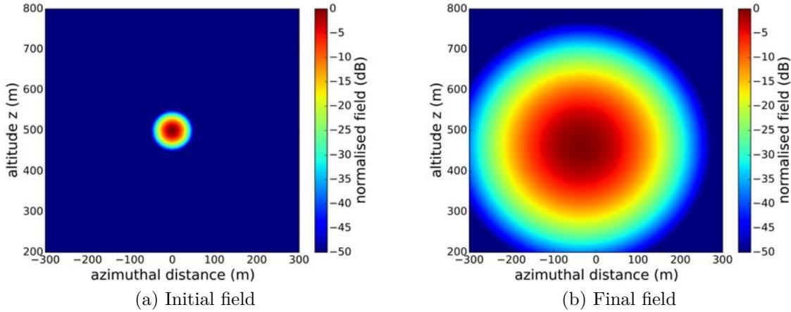
Figure 2.5: Initial and final normalized electric fields (dB) about the direction of propagation.
