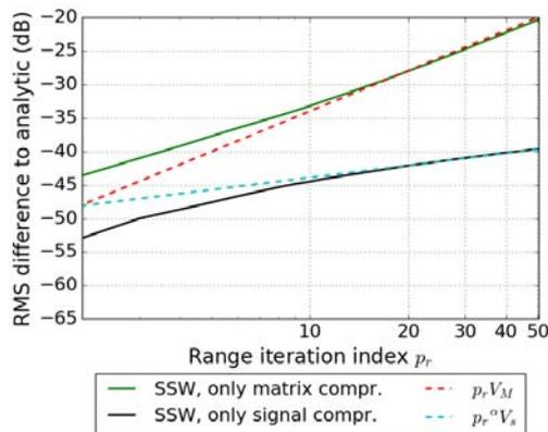
(a) RMS differences of SSW fields to SSF on range iterations
