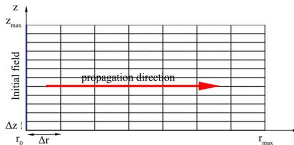
Figure G.2: Discretisation de 2D-SSF.
