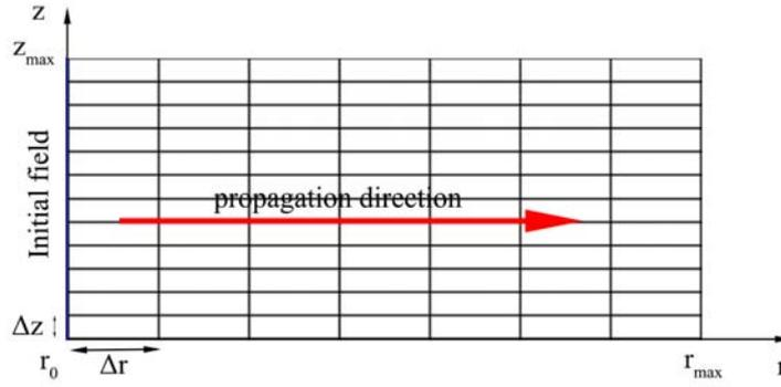
Figure 1.4: Discretization for the SSF.
