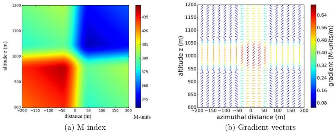
Figure 2.7: Refractivity (M-units/m) on the  $z - \theta$  plane.
