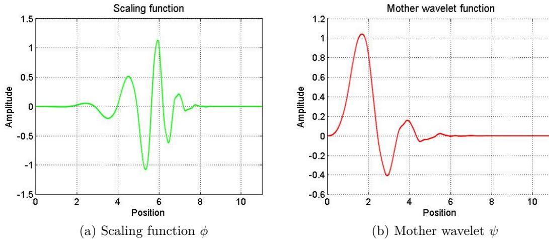
Figure 3.1: Scaling function  $\phi$  and mother wavelet  $\psi$  of *Daubechies* of order 6.
