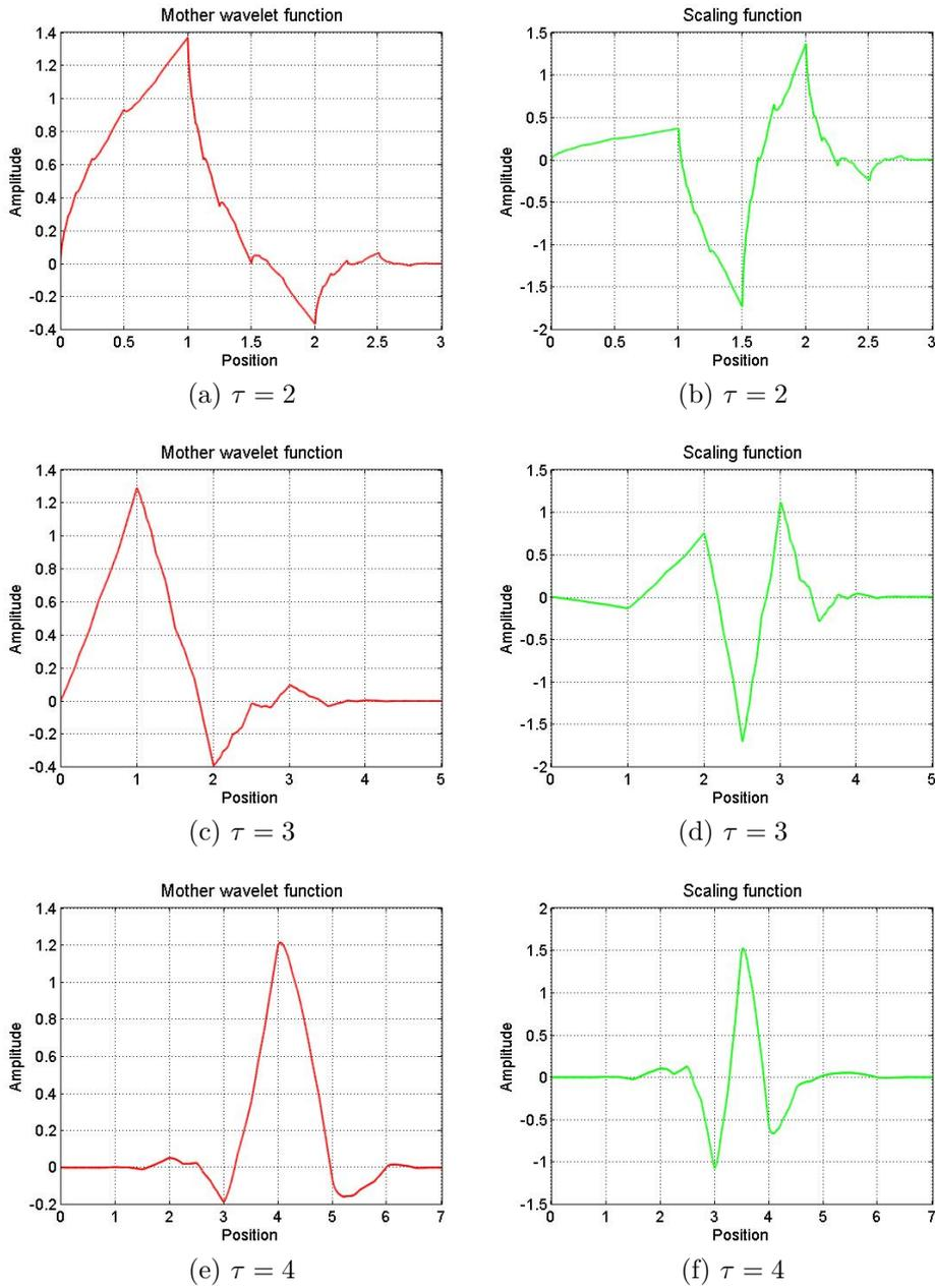
Figure 3.5: Symlets mother wavelet  $\psi$  and scaling function  $\phi$  of order  $\tau$ .
