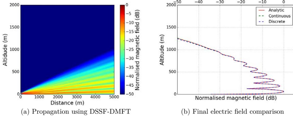
Figure 1.10: Propagation of a 2D complex source over a dry ground.
