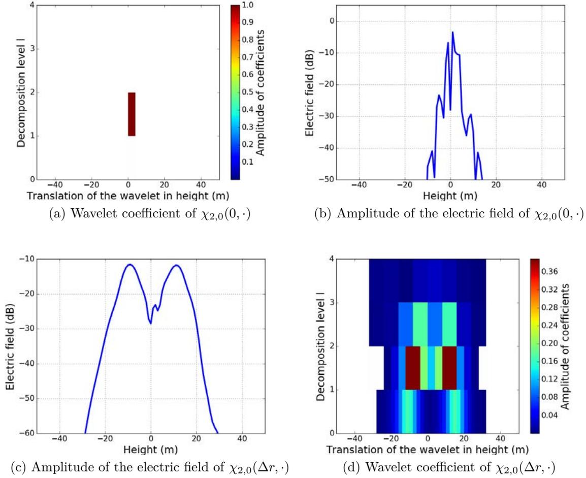
Figure 4.4: Propagation of the *symlets 6* wavelet  $\chi_{2,0}(0, \cdot)$ .
