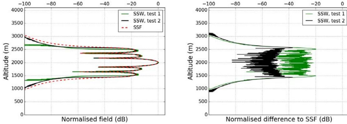
(a) Normalized electric fields at the final step obtained by SSF and SSW
