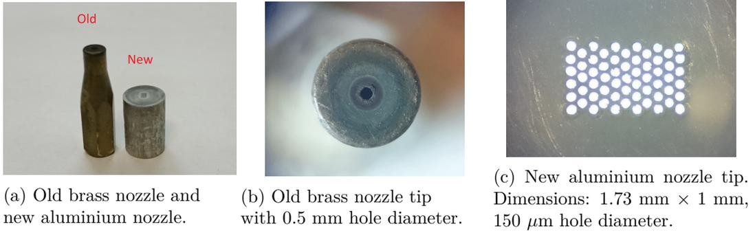
Figure 1.15 – Side and top views of both nozzles used in our setup.
