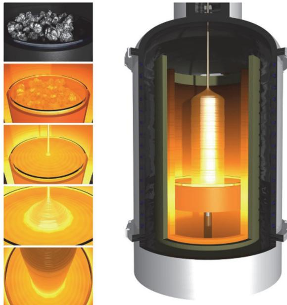
**Figure 3.2** Schematic diagram of the silicon crystal growth process using Czochralski method [48].
