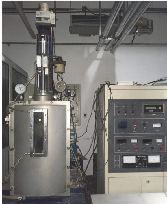
**Figure 3.3** TDJ-L50 Czochralski crystal growth furnace.
