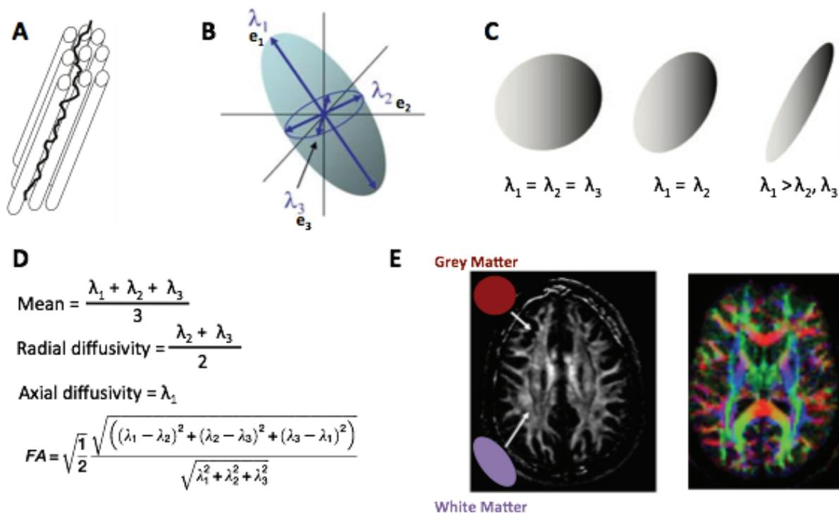
**Figure 32: DTI principle** - (A) Schematic illustration of water molecule diffusion within a fiber bundle (B) Diffusion tensor model in each voxel (3 eigenvectors and associated eigenvalues) (C) Schematic representation of the geometric shape and diffusion properties of the tensor (D) Measures derived from the tensor, in each voxel (E) Fractional anisotropy maps (with and without RGB color code depending on  $\lambda_1$ ) - Adapted from Mori et al, 2006; Berg and Rushworth, 2009
