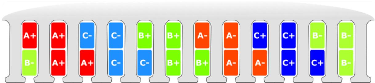
Figure A-5: Winding of a 2-pole 12-slot 3-phase machine with two layers per slot (double-layer winding). The coil span is reduced by one slot pitch ( $coil\ span = 5\ slots$  instead of  $oil\ span = 6\ slots$ ).
