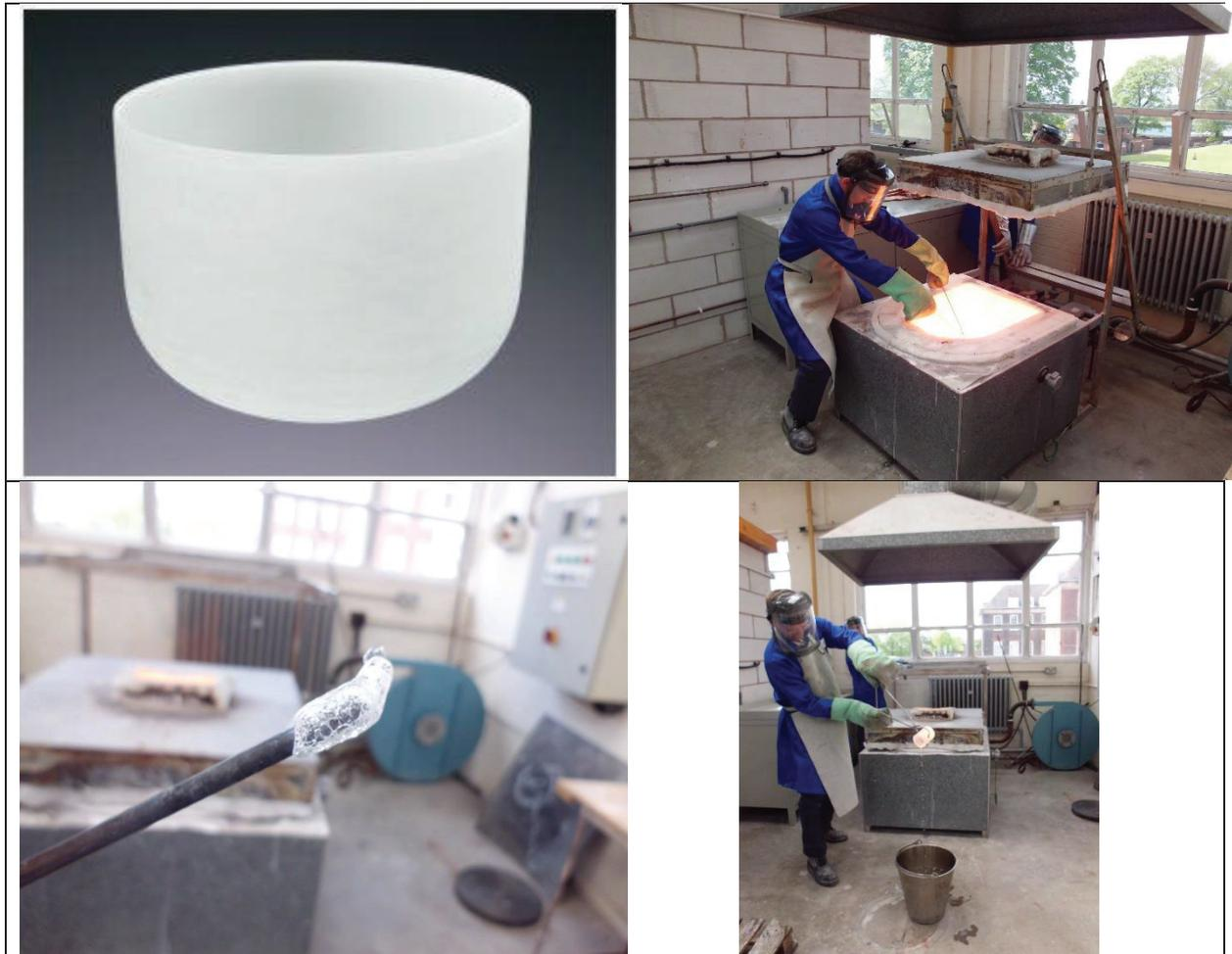
*Figure 19* Glass melting procedure: quartz crucible placed in the kiln, checking the glass melt and pouring it to obtain the frit.
