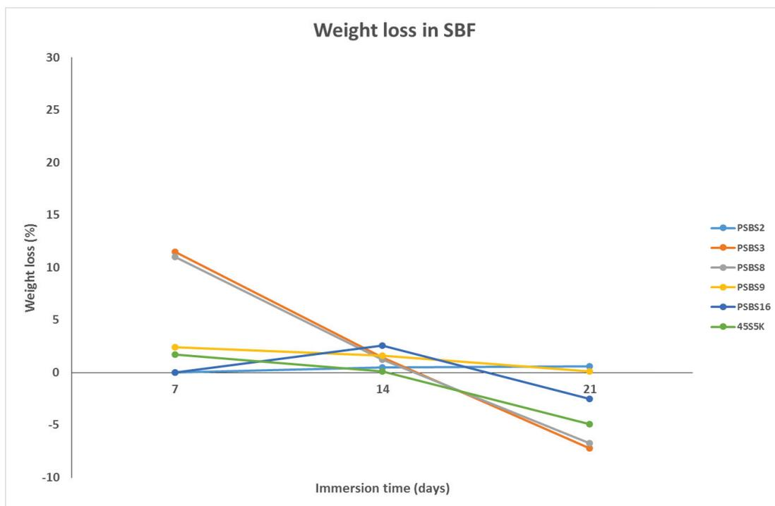
Figure 75 Weight loss of glass disks immersed in SBF at different time-points: 7, 14 and 21 days.
