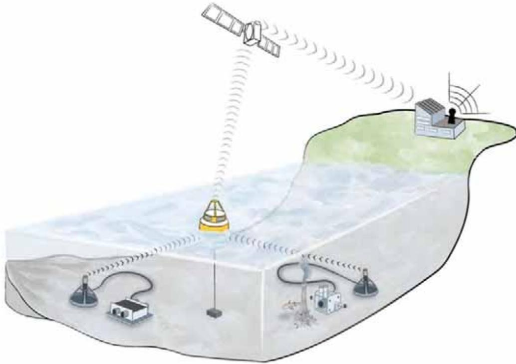
*Figure II - 8 Cartoon of the Emso Azores node infrastructure (www.fixO3.eu). At the seafloor, the two stations send data to the buoy BOREL. The Buoy then sends the data to the Ifremer center on shore.*
