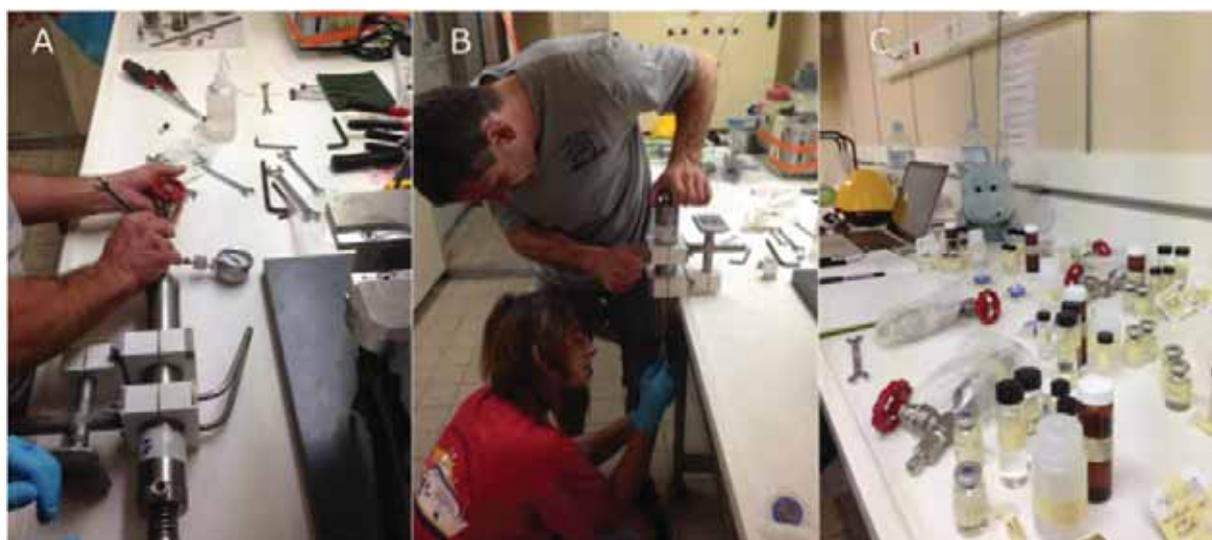
Figure III - 7 Photographs taken during the process of sample extraction in MoMARsat 2013. A: Mounting of a stainless steel canister to extract the gases; B: Extracting the fluid with a plastic syringe to be filtered through a 0.45 $\mu$ m Millipore filter and dispatched in several aliquots (C) Labelled aliquots of fluids and gazes dispatched on the working table.
