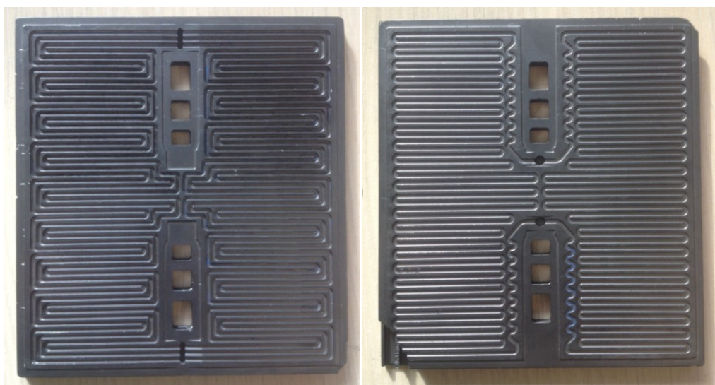
Figure 1.4 Actual geometry form of gas channel of NEXA PEMFC: the left one is cathode air channel, the right one is anode hydrogen gas channel
