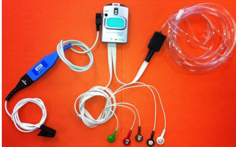
Figure 4.2: The prototype cardiorespiratory Holter device with associated sensors (ECG electrodes, SaO<sub>2</sub> ear sensor and nasal pressure cannula).
