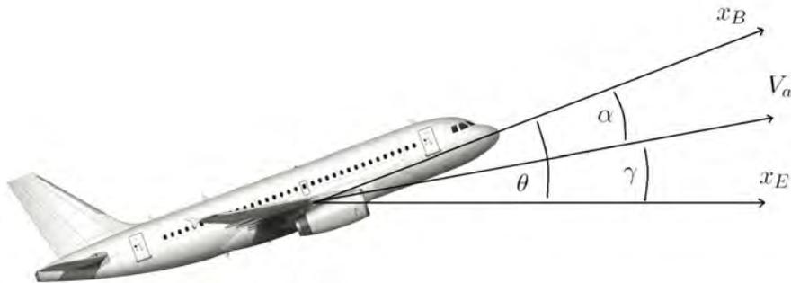
FIGURE 3.5: Flight Path Angle.
