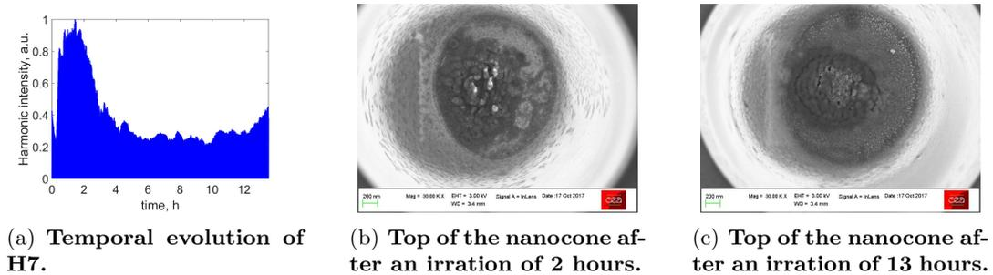
**Figure 5.9.:** Measurements of H7 at a peak intensity of  $0.063 \text{ TW}/\text{cm}^2$  and SEM-images of nanocones after laser irradiation.
