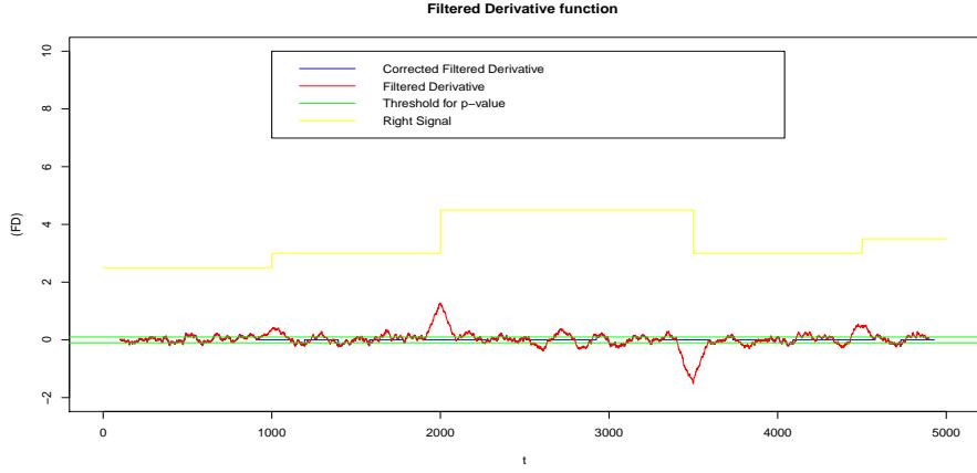
FIGURE 2.4 – *Filtered Derivative function with noise ( $\sigma = 1$ ).*
