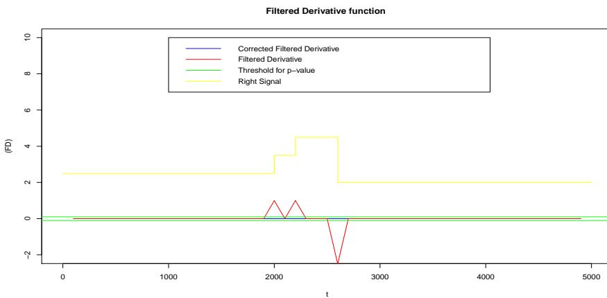
FIGURE 2.8 – The Filtered Derivative without noise and  $A=100$ .
