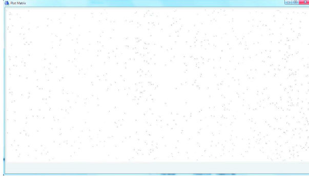
Figure 5.12 – Accumulation of 10^4 events at a thresholds of 5 times the noise acquired in the dark for one sensor.
