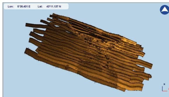
Figure 6.5 – High resolution Backscatterer mosaic of the survey conducted in La Ciotat (France) in December 2015. The visualization is shown by superposing each survey line. The map is presented via Delph Roadmap software, under resolution of 0.1m.
