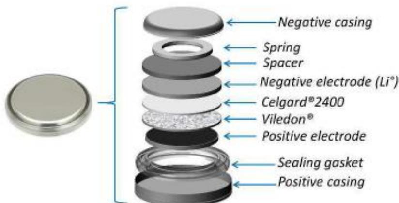
Figure 2-6. Exploded view of 2032 coin cells components in half-cell configuration versus metallic lithium, reproduced from [255].
