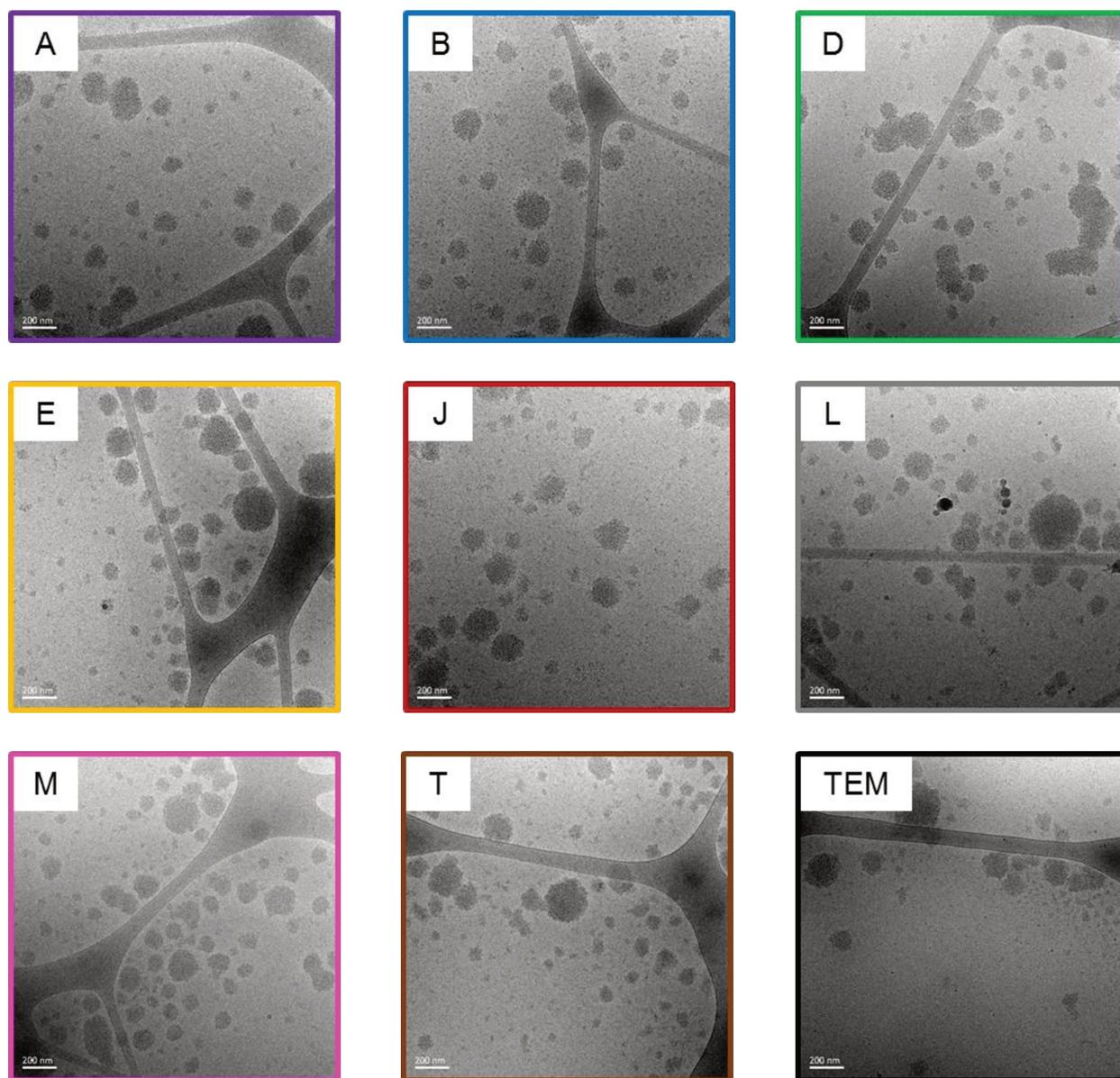
**Figure 6: Cryo-TEM micrographs of the selected suspensions.** Large black strands crossing the images are carbon grids; circular or merged spots are casein micelles or aggregated casein micelles; dark round spots in suspension L are ice particles that formed during storage of the grids in liquid nitrogen.
