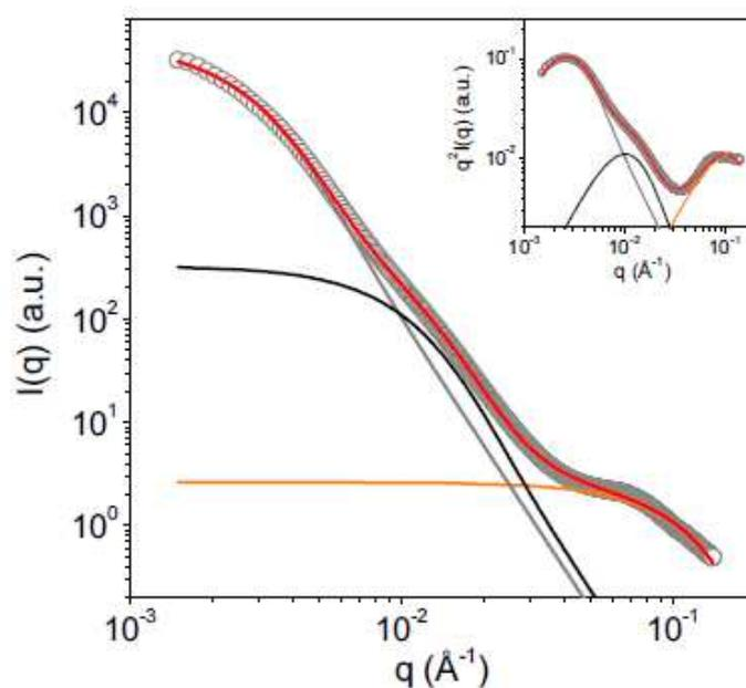
**Figure 13: SAXS pattern of a 25 g kg<sup>-1</sup> suspension of pure casein micelle in milk ultrafiltrate obtained on synchrotron facilities** (Bouchoux et al. 2010). Open circles are the experimental data; red line corresponds to the best-fit form factor model defined in Bouchoux et al. The contributions of each structural level are displayed in grey (casein micelle), black (hard region) and orange (CaP nanocluster).
