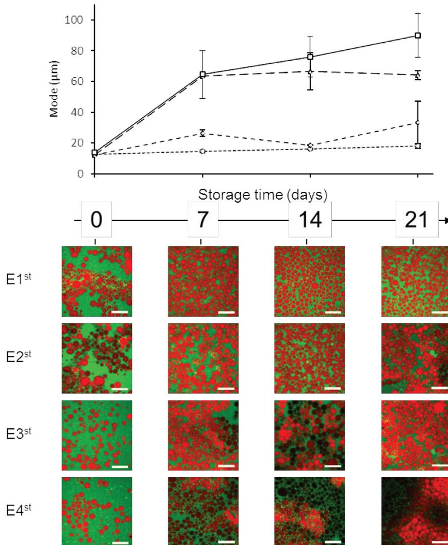
**Figure 7. Microscopic evolution of the emulsions over time (E<sup>st</sup>).** Droplet size (mode) and confocal micrograph evolution as a function of storage time: E1<sup>st</sup> (○)(····), E2<sup>st</sup> (◇)(- - -), E3<sup>st</sup> (△)(—) and E4<sup>st</sup> (□)(—). Microscopy images were recorded at 50°C using a thermal plate warmer. Milkfat emulsion droplets (in red) are surrounded by casein (in green). Contrast differences are attributed to the
