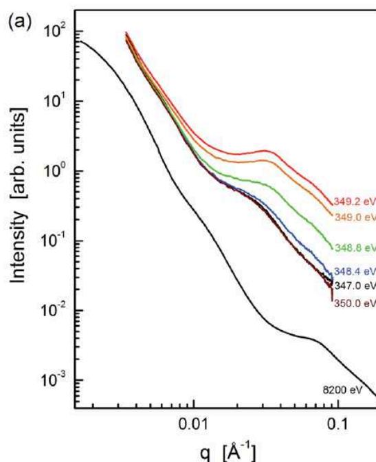
**Figure 14: Resonant X-ray scattering pattern of skim milk (Ingham et al., 2015).** The energy beam varied near the Ca L2-edge as labelled (color lines). The black line corresponds to typical synchrotron SAXS data collected at 8200 eV.
