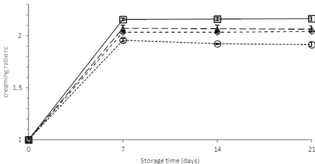
**Figure 6. Time evolution of creaming ratios  $r_c$  of emulsions prepared for the determination of emulsion stability ( $E^{st}$ ).** Creaming ratio defined as  $r_c = H / h$  where  $H$  is the total height of the emulsion and  $h$  the thickness of the creamed layer. Standard deviation bars are represented behind the point marks.
