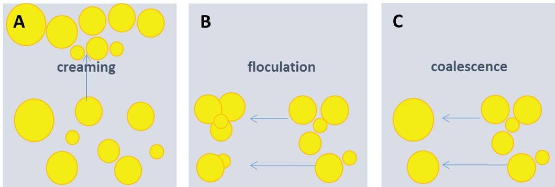
Figure 18. Schematic representation of the mechanisms responsible for the instability of milkfat-in-water emulsions. A. Gravity creaming, B. Floculation and C. Coalescence of the milkfat droplets.
