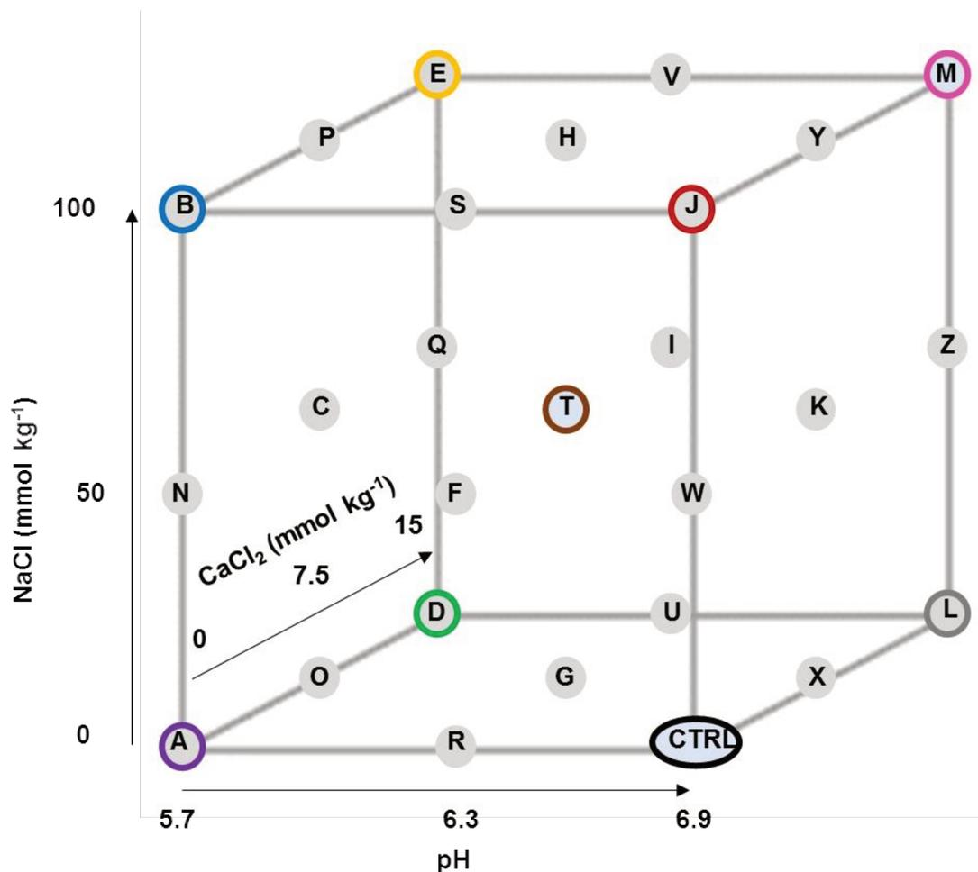
**Figure 1: Cubic representation of the experimental design.** Each of the 27 suspensions is represented by a letter or designated as CTRL (control suspension, pH 6.9, no salts added). The pH of the suspensions was set to 5.7, 6.3 or 6.9 and the suspensions contained 0, 50 or 100 mmol kg<sup>-1</sup> of added NaCl and 0, 7.5 or 15 mmol kg<sup>-1</sup> of added CaCl<sub>2</sub>.
