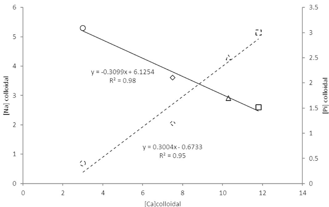
**Figure 2. Correlations between colloidal Ca, Na and Pi concentrations.** Colloidal Pi (—) and colloidal Na (- - -) as a function of colloidal Ca for: S1<sub>d</sub> (○), S2<sub>d</sub> (◇), S3<sub>d</sub> (△) and S4<sub>d</sub> (□). Concentration are in mmol kg<sup>-1</sup>.
