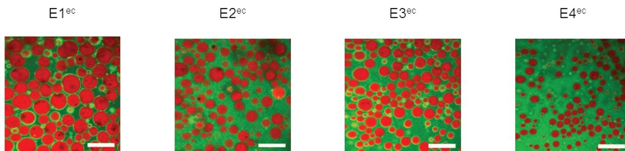
**Figure 5. Confocal laser scanning microscopy images of the emulsions prepared for determination of emulsifying capacity (E<sup>ec</sup>).** Microscopic images were recorded at 50°C using a thermal plate warmer. Milkfat emulsion droplets (in red) surrounded by casein (in green). Scale bars measure 50 μm.
