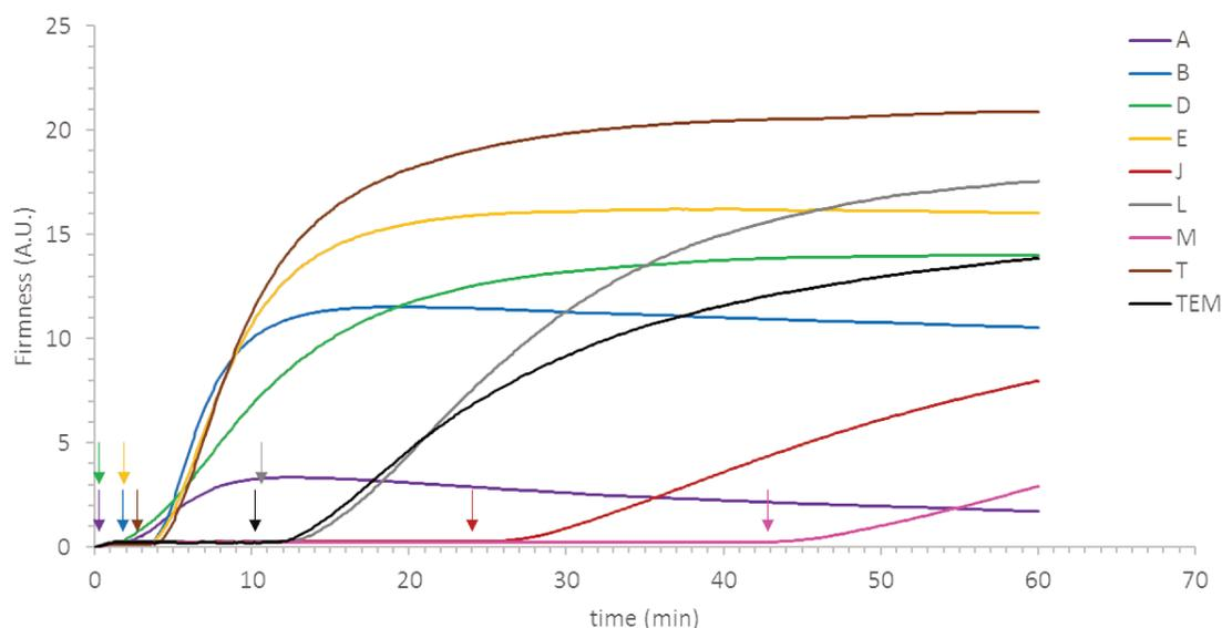
**Figure 8: Firmness evolution as a function of time for the selected samples.** Arrows are pointing at the RCT of each suspensions, while firmness was defined as the maximum firmness reached within the 60 min after the addition of chymosin to the suspensions. Values of the RCT and firmness are reported in Table 3.
