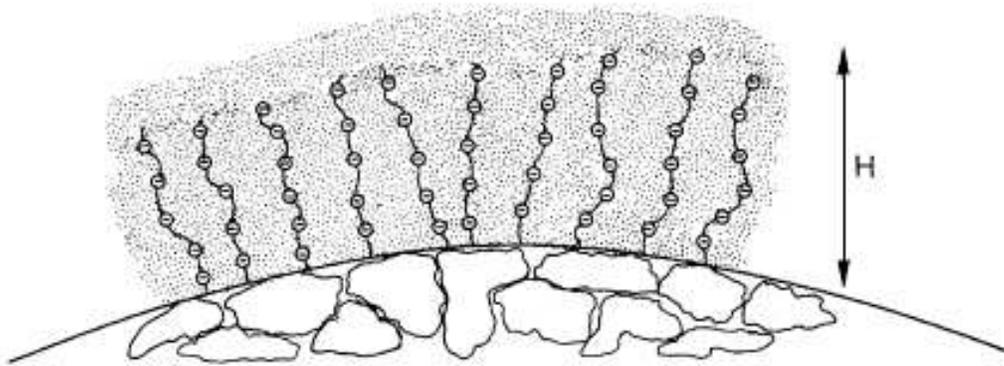
**Figure 6: Schematic representation of the  $\kappa$ -casein hairy layer.** The small dots represents the salts ions in solutions that interacts with the charge casein chains. H letter defines the thickness of the layer (between 5 and 10 nm). From de Kruif, (1999).
