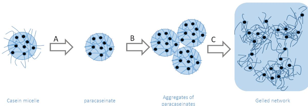
**Figure 19. Schematic representation of the mechanism responsible for the rennet coagulation of casein micelles.** A. hydrolysis of CMPs, B. aggregation of paracaseinates and C. gel formation and reorganization.
