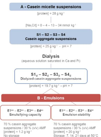
**Figure 1. Preparation of CA suspensions and emulsions.** d, ec and st represent «dialyzed», «emulsifying capacity» and «stability», respectively.
