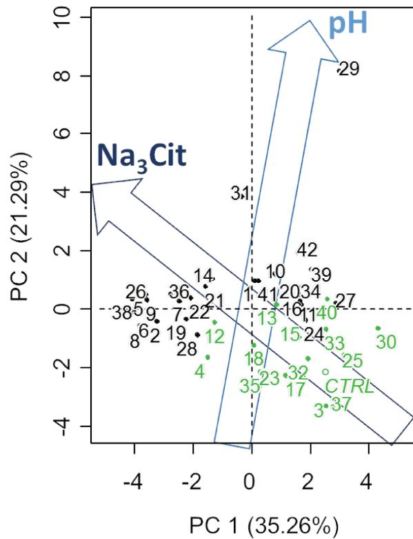
**Figure 2: PCA showing the similarity map for the suspensions in the plane determined by the first two PCs.** Coagulating and non-coagulating suspensions are colored in green and black, respectively. Arrows remind the directions of the pH and Na<sub>3</sub>Cit variables in the correlation circle represented in the same PCs plane (see Fig. 1A).
