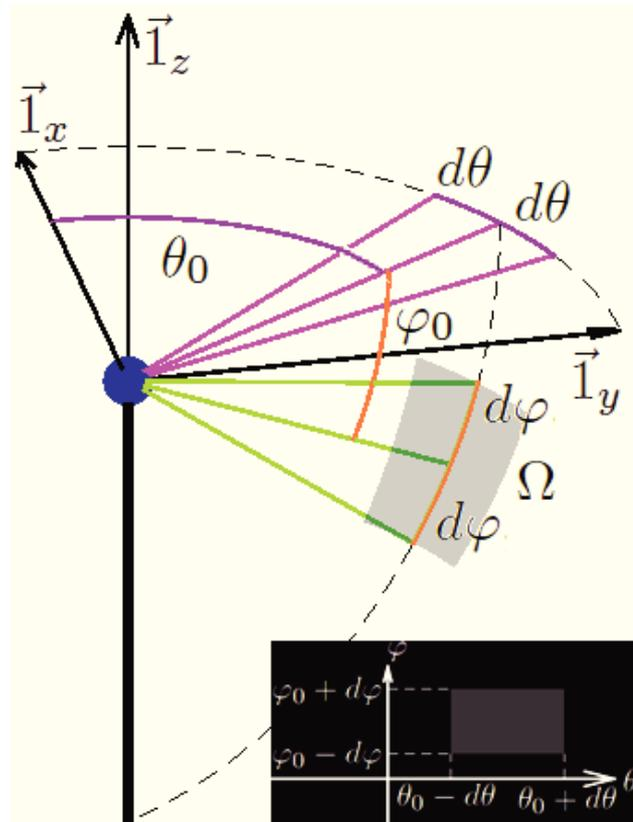
**Figure 5.6:** Illustration of angular parameters of the source. The grey surface  $\Omega$  represents a portion of the source as a unit sphere captured by the spherical coordinates  $(\theta_0 \pm d\theta, \varphi_0 \pm d\varphi)$
