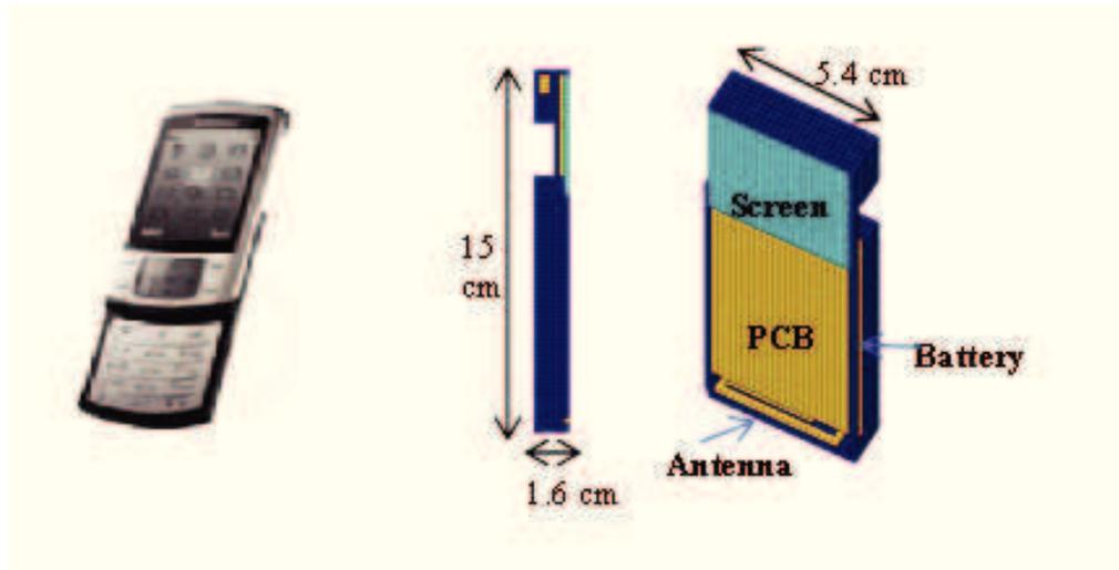
**Figure 2.9:** Example of digital model of mobile phone
