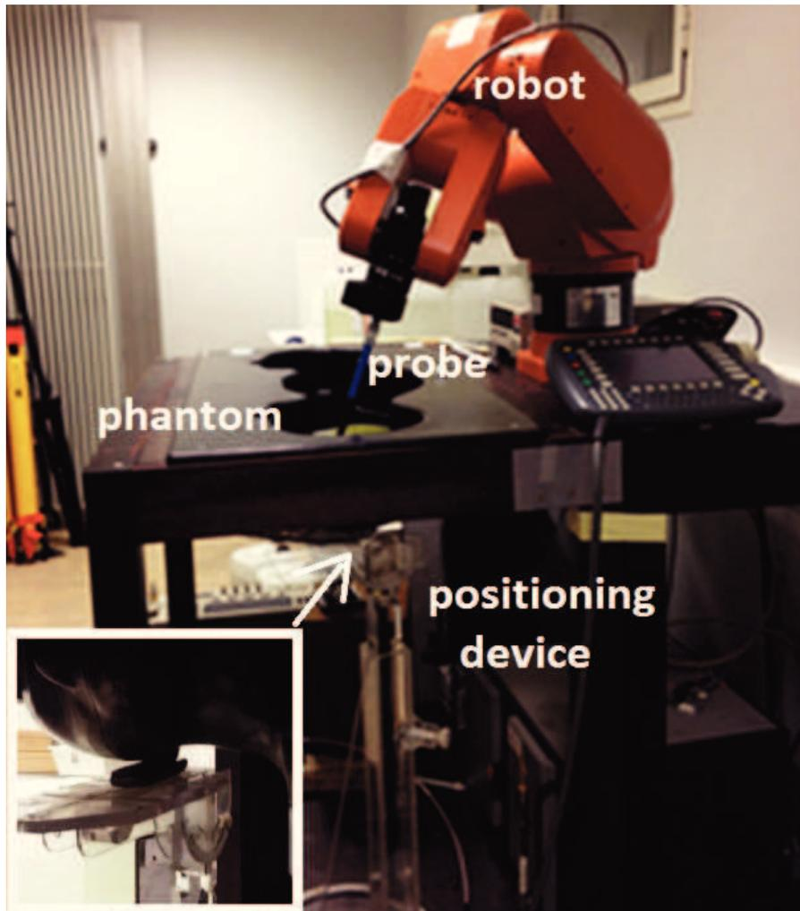
**Figure 2.10:** Dosimetric measurement setup for SAR measurement
