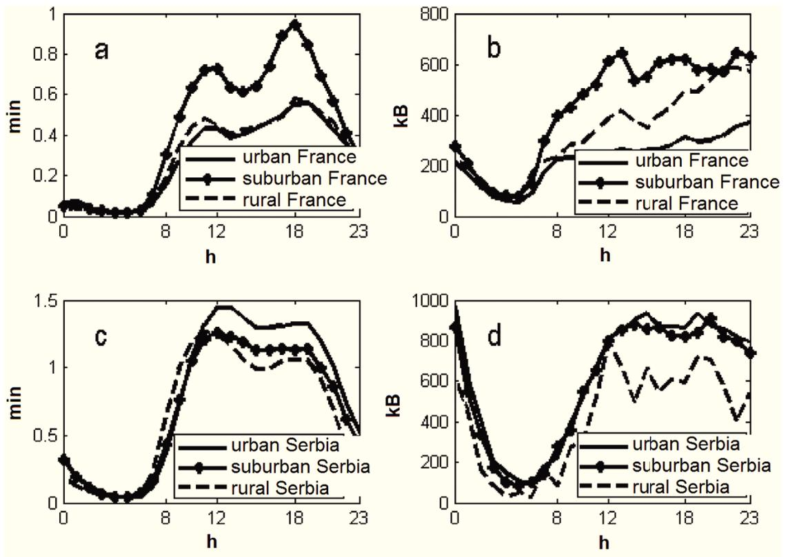
**Figure 3.3:** (a): Time variations of mean voice usage and (b) data usage per user over 24 h in macro 3G network of Orange France; (c) variation of mean voice usage and (d) data usage per user over a day in macro 2G and 3G network of Telekom Srbija.
