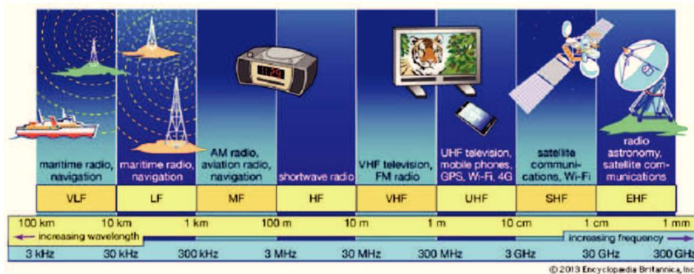
**Figure 2.1:** Commercially exploited bands of the RF spectrum.
