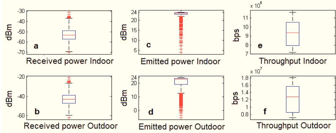
**Figure 5.10:** Received power from eNB, emitted power by mobiles in data service and mobiles' uplink throughput in indoor and outdoor environments
