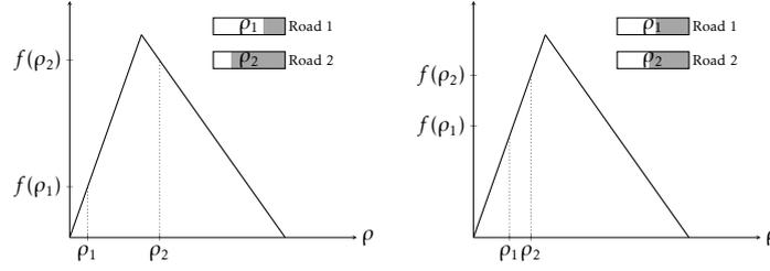
Figure 4.1 – Illustration of the density balancing idea. Considering the figure on the left, a value of TTD is obtained for  $J = f(\rho_1) + f(\rho_2)$  which corresponds to an uneven distribution of vehicles in the two roads. Balancing the densities improves this by keeping a similar value of  $J$  but better distributing the total charge.
