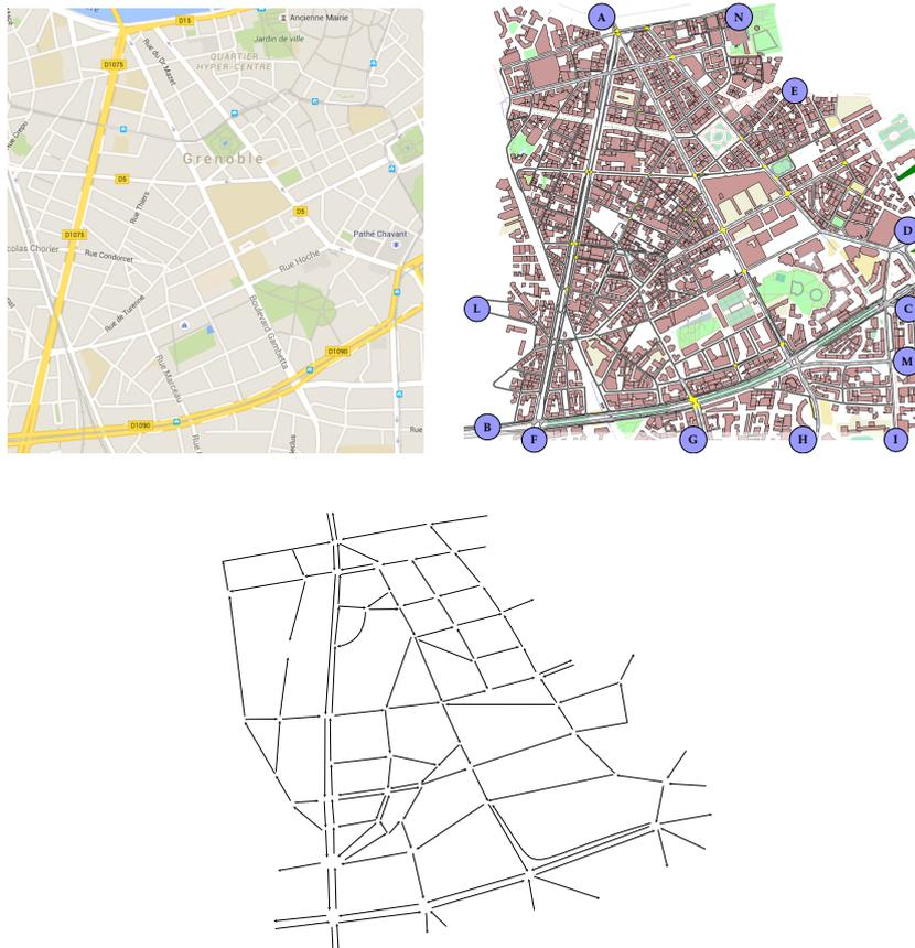
Figure 5.4 – From top left, clockwise: an image of Grenoble, from Google Maps; the Aimsun model used in the microscopic experiments, with markers for the detector positions, that correspond to the inflows of the model (see also Figure 5.5); the graph we superimposed to the network, in order to represent connectivity between roads. A demo of our experiments is available online at the url [48].
