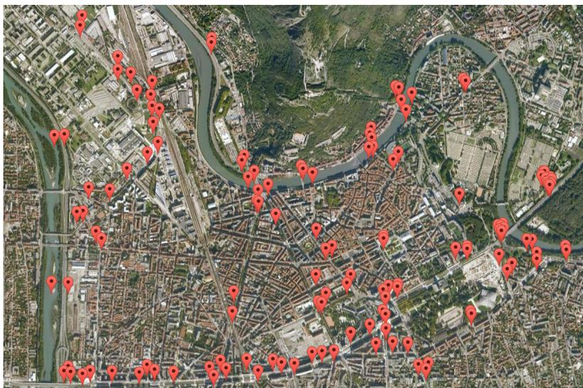
Figure 8.2 – Positions of the loop detectors installed in Grenoble. We used the measured data about flow of vehicles in order to set up the demand into the Aim-sun model and to calibrate every junction with reasonable values of split ratios. The view of the city is taken from Google Earth.
