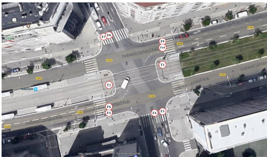
Figure 8.4 – Topology and traffic lights for the illustrative intersection. The background image is taken from Google Earth.
