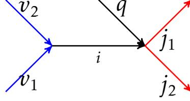
Figure 7.1 – Illustration of the required sharing of information for the variables  $\bar{u}$ . The subproblem created for road  $i$  is defined in a small neighborhood that involves upstream roads in  $\mathcal{N}_i^- = \{v_1, v_2\}$ , downstream roads in  $\mathcal{N}_i^+ = \{j_1, j_2\}$ , and roads in  $\mathcal{I}_i = \{i, q\}$ . In order to solve the problem distributedly, variables need to be shared within this neighborhood.
