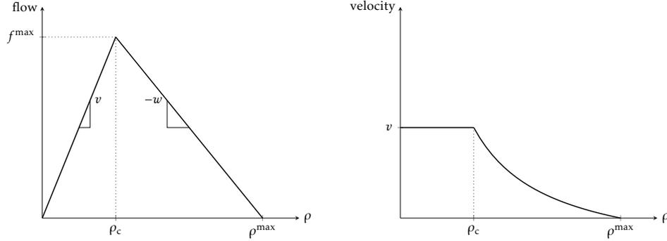
Figure 3.1 – Fundamental diagrams density-flow and density-speed that describe correlation between important quantities in traffic systems. The value of density  $\rho_c$  is usually said *critical density*, and it represents the switching point between a free-flow condition and a congested one.
