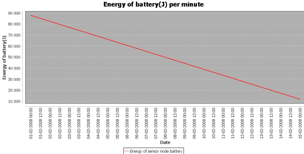
Figure 5.2.3: Battery energy of libelium node when the sample frequency equals the communication one
