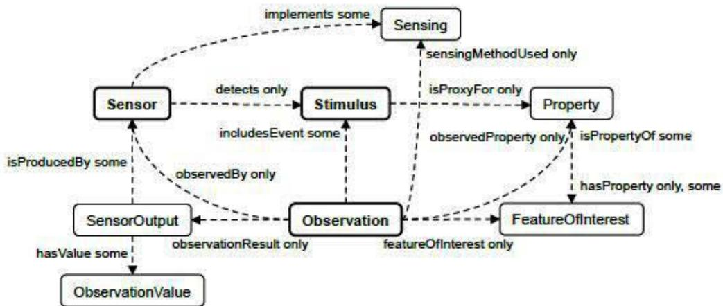
Figure 2.3.1: Stimulus-Sensor-Observation pattern of SSNO (Compton *et al.*, 2012)
