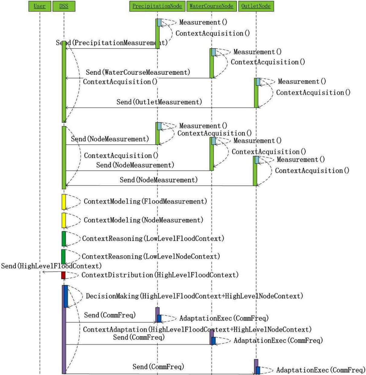
Figure 4.4.1: Sequence diagram of an adaptive context system integrating two different context-aware systems
