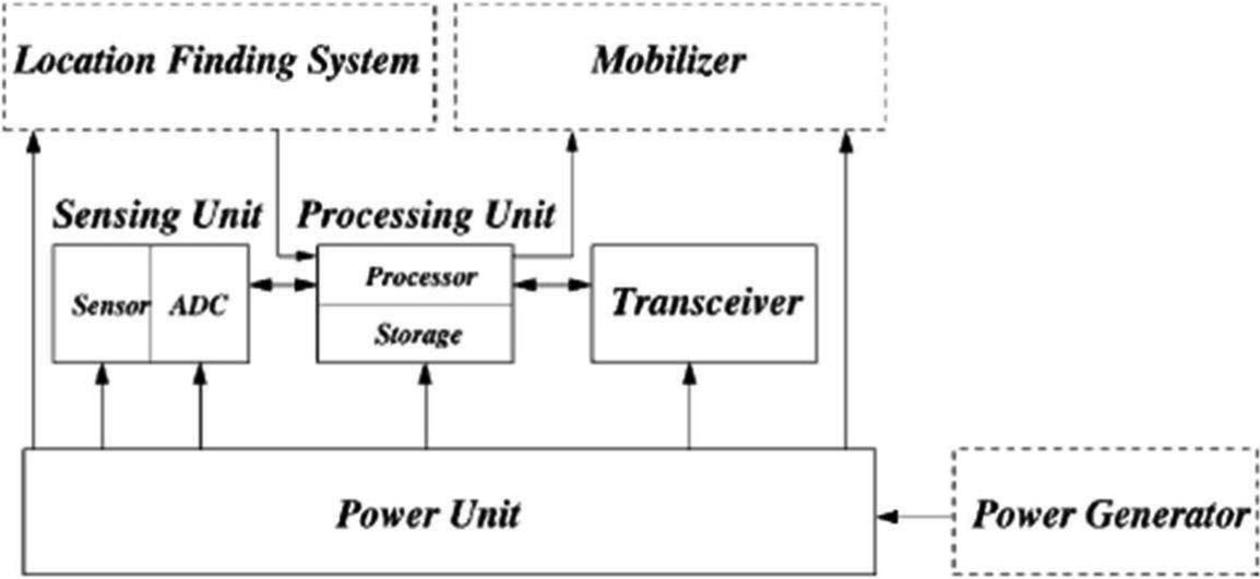
Figure 5.2.1 Sensor node components (Akyildiz et al., 2002) (Akyildiz et al., 2002b) (Wang et al., 2004)
