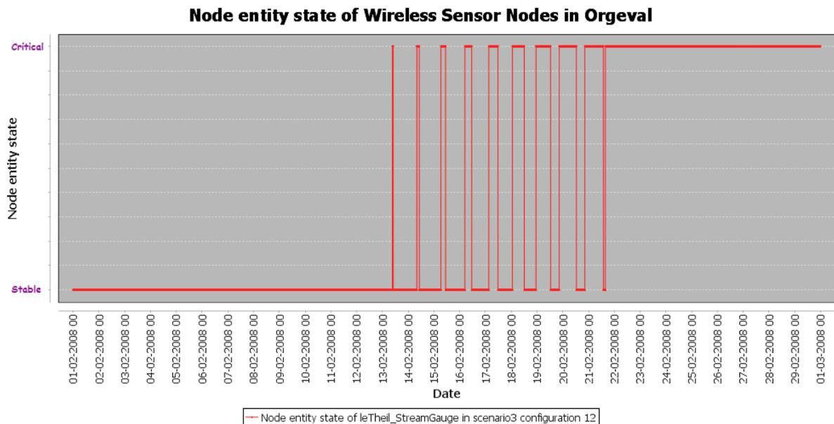
Figure 6.5.4: Node entity states evolution of the outlet node in scenario 3 configuration 12 for February, 2008
