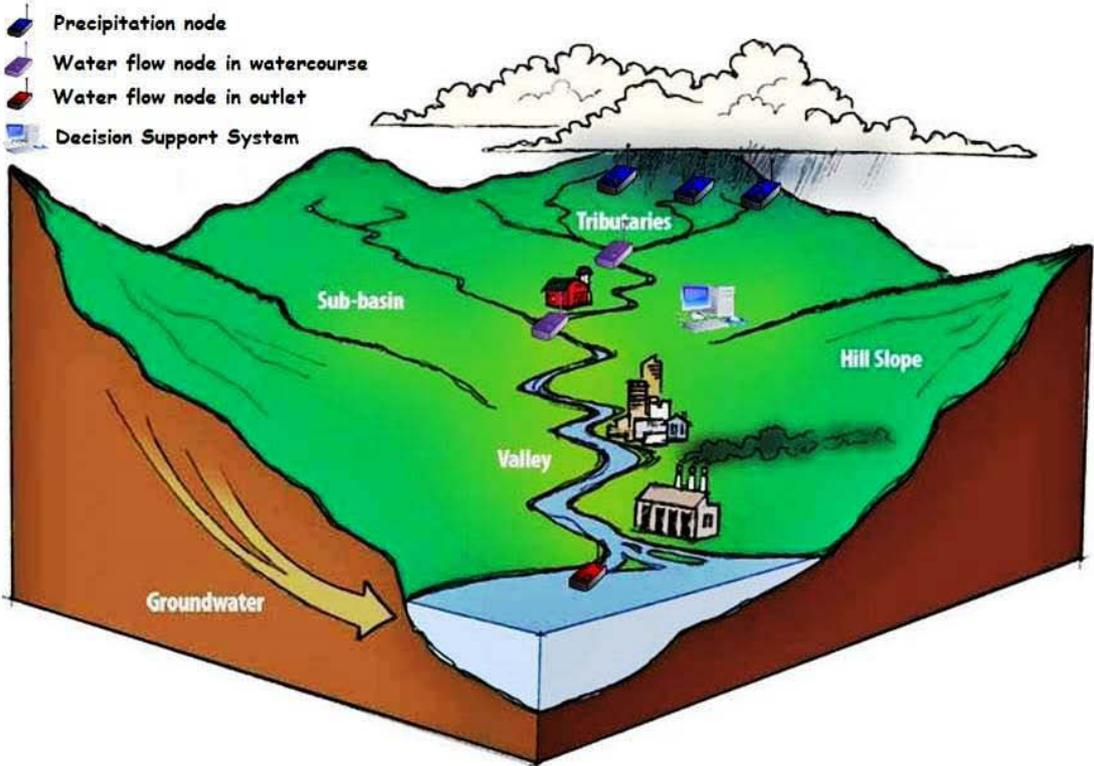
Figure 4.2.1: Example of watershed monitoring (Heathcote, 1998)
