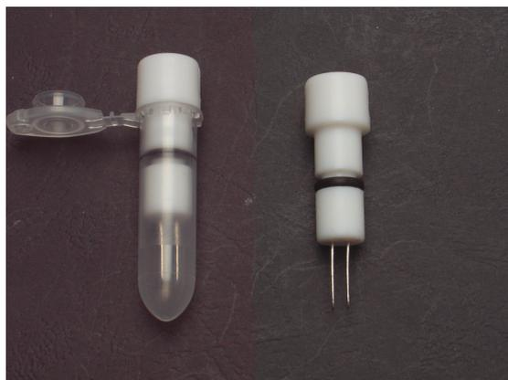
**Figure 3.1:** Picture of the home-made PTFE electroformation cap, with and without the growth chamber consisting of a centrifugation microtube.
