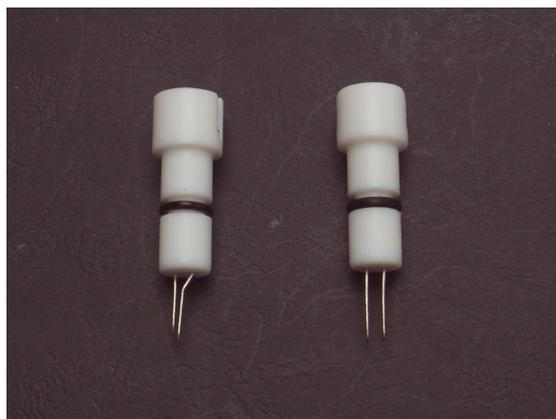
**Figure 3.3:** Picture of two home-made PTFE electroformation caps with different gaps between the platinum electrodes, (left) 1 mm and (right) 2.5 mm.
