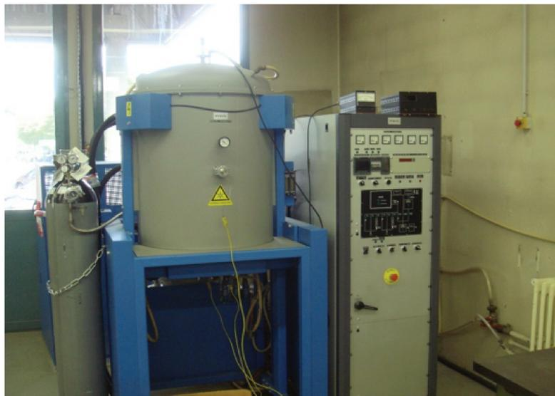
FIGURE 3.2: LAL furnace for vacuum brazing process of components.
