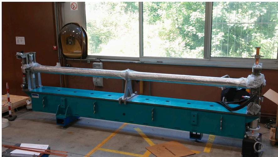
FIGURE 2.12: Picture of the LIL accelerating section lent by the SOLEIL laboratory.
