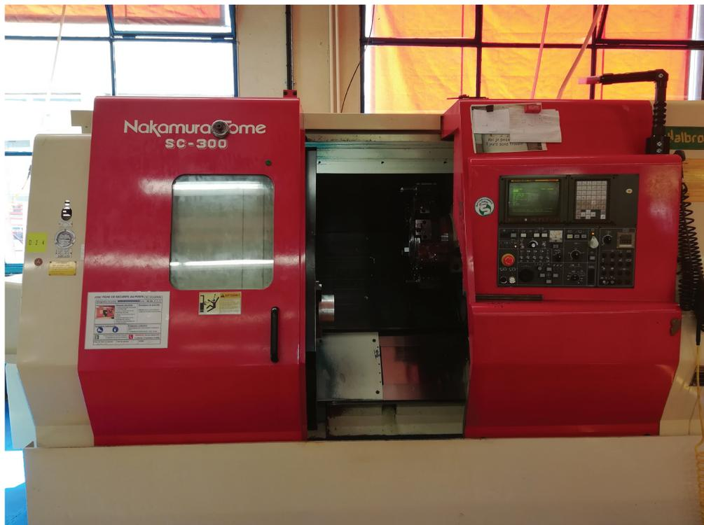
FIGURE 3.3: Multi-tasking precision lathe for machining process at LAL.
