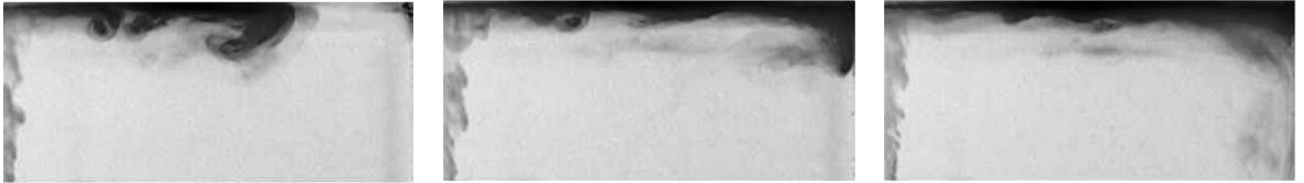
Figure 1.9: Instantaneous experimental images from [KH07] with \phi > 1.5 . Left: outflow from plume, middle: side-wall spreading flow, right: slumping back mode.
