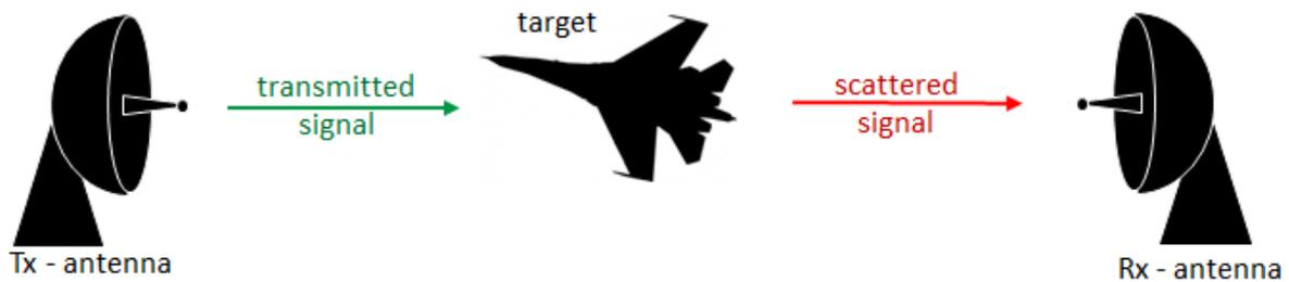
Figure 1.4 Forward scatter radar
