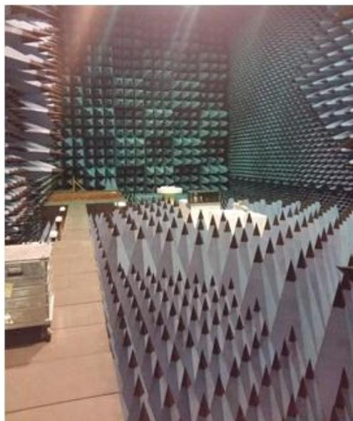
Figure 1.19 CHEOPS anechoic chamber
