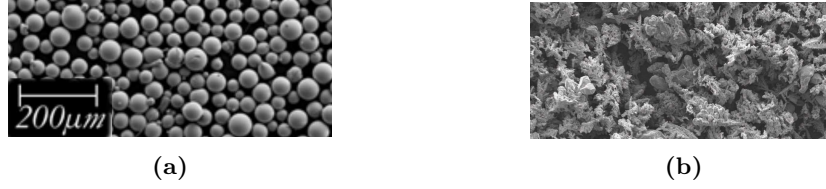
Figure 2.13: SEM views of the initial state of the powders at identical scales. (a) Atomized amorphous \text{Zr}_{57}\text{Cu}_{20}\text{Al}_{10}\text{Ni}_8\text{Ti}_5 : spheroidal powder. SEM view from [73, p.41]. (b) Electrolytic crystalline copper: dendritic powder.
