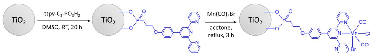
**Scheme IV-10.** Synthesis route to TiO<sub>2</sub>/Mn<sup>I</sup> NPs
