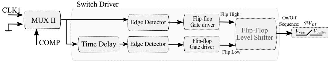
Figure 4.14: Switch Control Block
