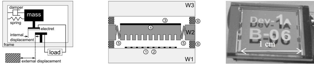
Figure 2.7: Left: schematic, middle: device cross section Right: Top view [49].
