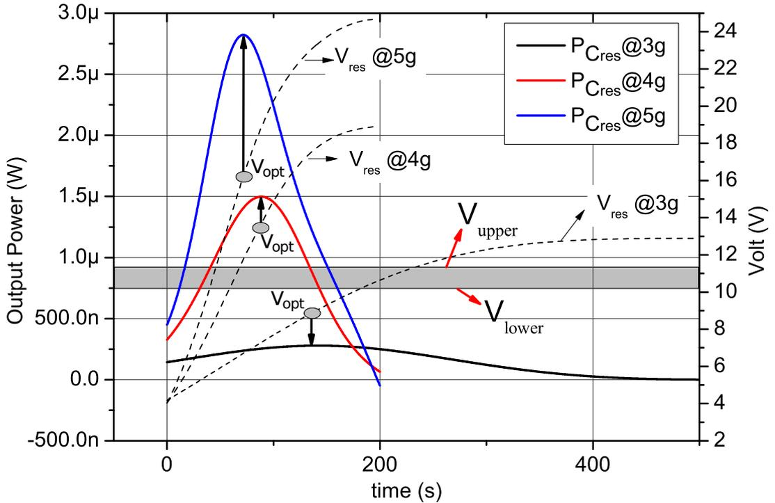
**Figure 3.5:** Series-Parallel Charge Pump CC measurements for  $V_{res}$  and  $P_{C_{res}}$  different  $g$  with vibration frequency of 187.2 Hz,  $C_{res} = 1\mu F$  and  $C_{store} = 2.8nF$ .
