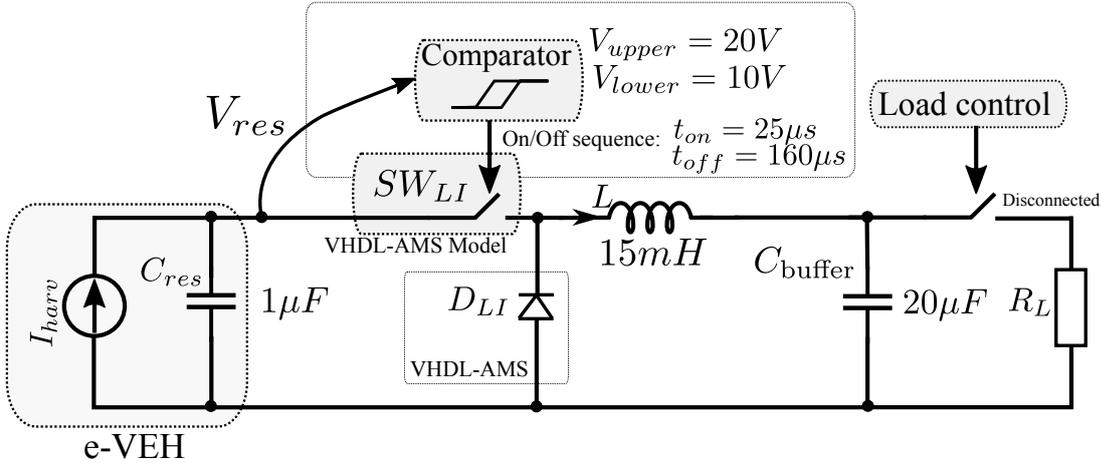
Figure 3.11: Multiple Energy-Shot transfer LI VHDL-AMS model
