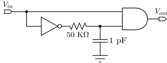
**Figure 4.19:** Rise-edge detection circuit for  $SW_{LI}$  command generation;
