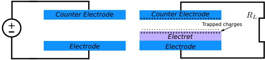
**Figure 2.2:** Electret-Free (Left) versus Electret (Right)
