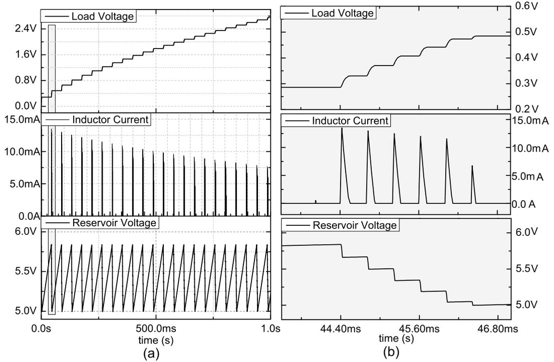
**Figure 3.12:** VHDL-AMS model of multiple shot energy transfer showing inductor current  $i_L(t)$ , reservoir  $V_{res}(t)$  and load  $V_{load}(t)$  voltages with design parameters  $L = 10mH$ ,  $C_{res} = 1\mu F$ ,  $C_{load} = 20\mu F$ ,  $V_{resH} = 6V$ ,  $V_{resL} = 5V$ ,  $I_{harv} = 2mA$ ,  $I_{Lmax} = 15mA$ ,  $t_{on} = 25\mu s$  and  $t_{off} = 160\mu s$  where (a)  $0s < t < 1s$  and (b)  $44ms < t < 47ms$ .
