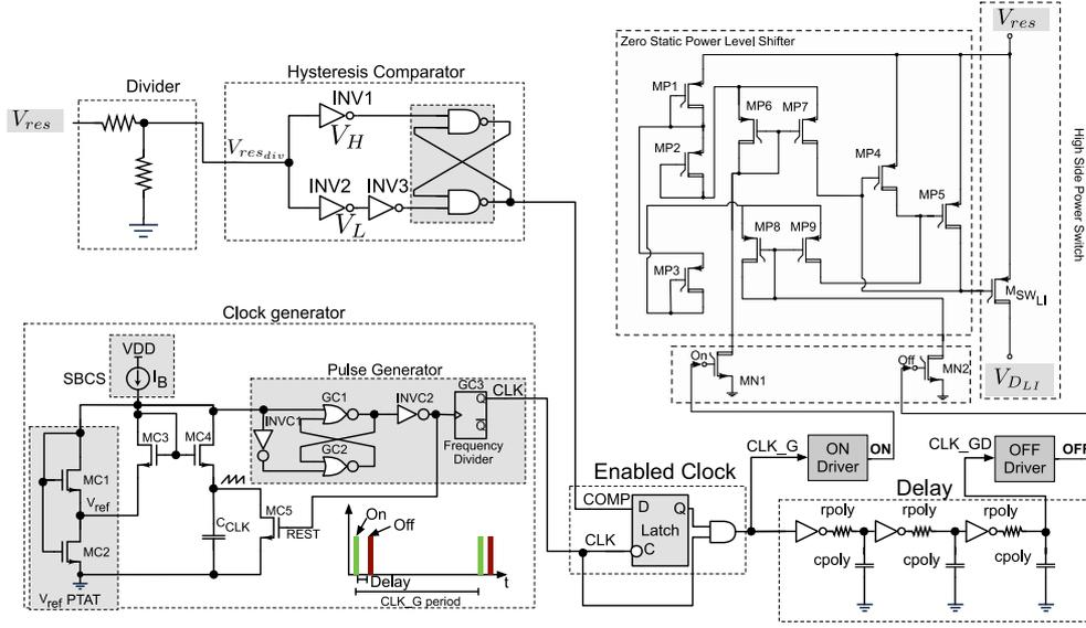
Figure 5.13: Modified Load Interface system blocks
