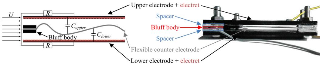
**Figure 2.11:** Flutter-and-electret-based airflow energy harvester by [54]
