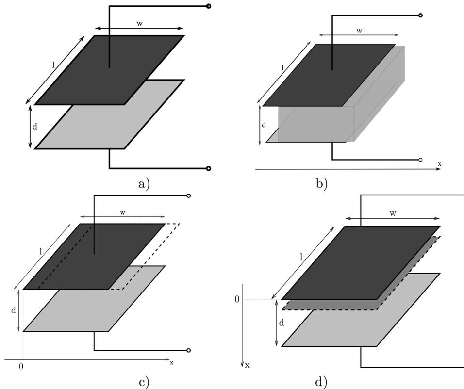
**Figure 1.6:** Different transducer geometries (a) parallel plate (b) a movable dielectric (c) out-of-plan parallel electrodes (d) gap-closing capacitors.
