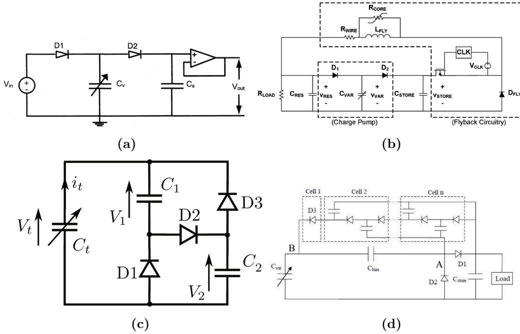
**Figure 2.15:** Self-Synchronized energy extraction showing (a) Charge-Pump by Roundy et al. [6] (b) Charge-pump with flyback by Yen et al.[24] (c) Bennet's doubler by [33] (b) Modified Bennet's doubler by [67]
