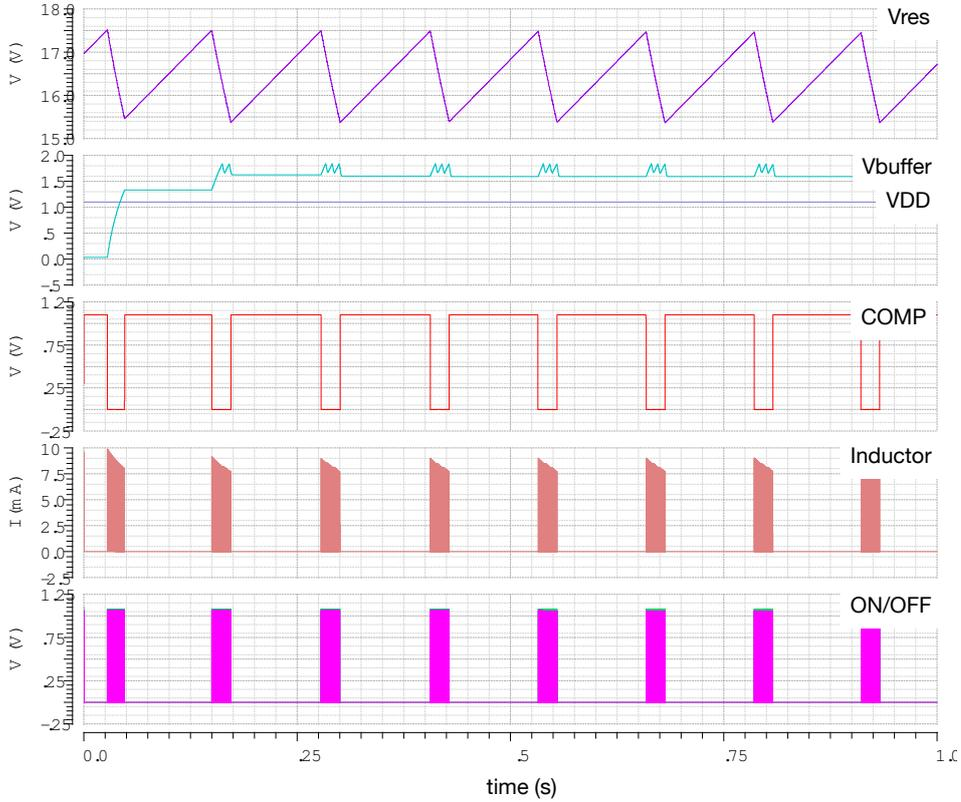
**Figure 5.17:** Simulation results showing  $V_{res}$ ,  $V_{buffer}$ ,  $COMP$ ,  $I_L$  and  $ON/OFF$  commands
