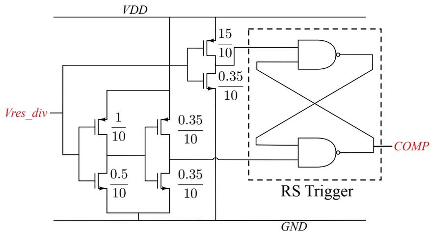
**Figure 5.9:** Hysteresis comparator schematic - COMP1
