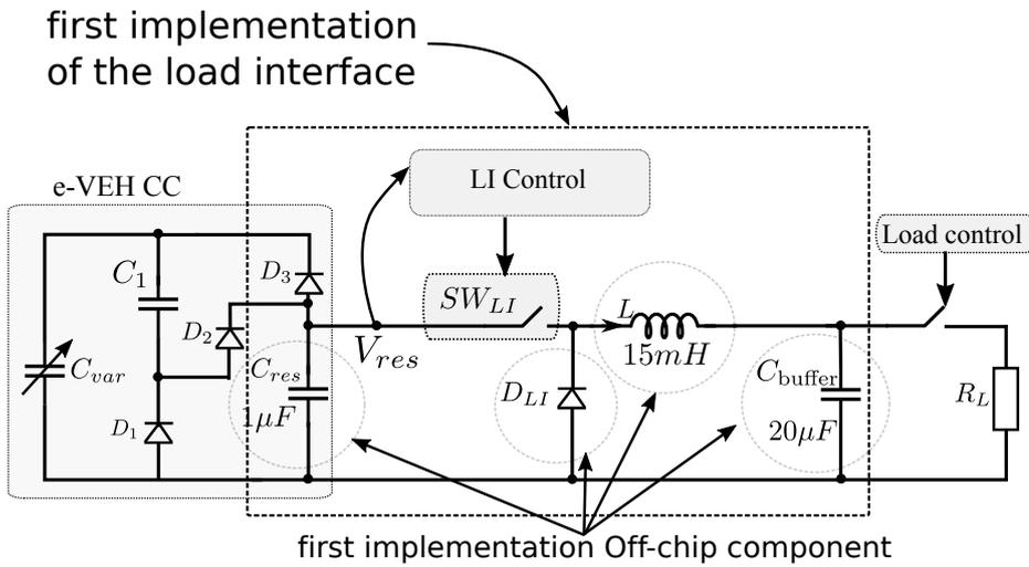
**Figure 4.2:** Load Interface showing off chip blocks
