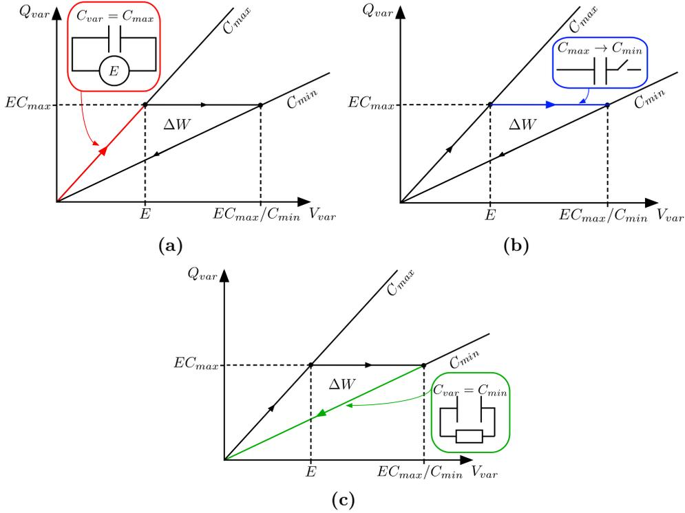
**Figure 1.8:** Charge constrained Q-V diagram energy conversion cycle
