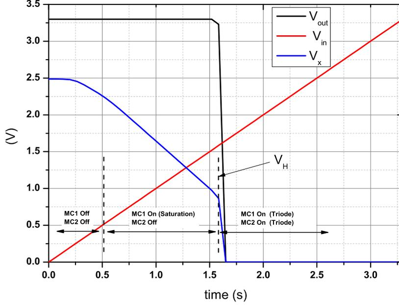
Figure 4.9: Transition of  $V_x$  with  $V_{in}$  increases
