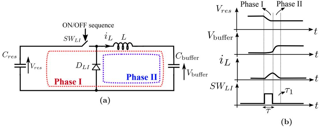
Figure 3.4: Buck converter interface (a) Buck Load schematic (b) Switch time digram
