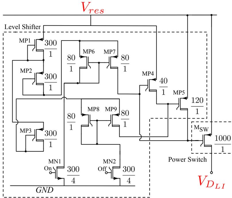
Figure 5.10: Power Switch with zero-static current level shifter
