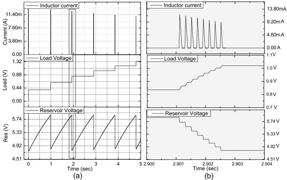
**Figure 4.21:** Load interface MOSFET simulation of multiple energy-shot transfer showing inductor current  $i_L(t)$ , reservoir  $V_{res}(t)$  and load  $V_{load}(t)$  voltages where (a)  $0s < t < 5s$  (b)  $2.9s < t < 2.904s$
