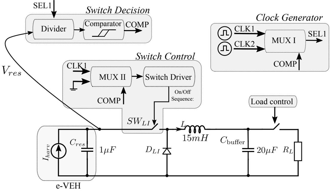
**Figure 4.3:** Load interface architecture implementing the  $V_{res}$  regulation
