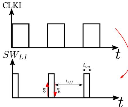
Figure 4.18: Switch Driver command to  $SW_{LI}$
