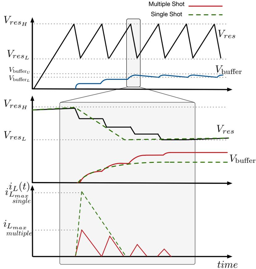
**Figure 3.10:** Reservoir voltage  $V_{res}(t)$ , buffer voltage  $V_{buffer}(t)$  and inductor current  $i_L(t)$  illustration of multiple energy-shot transfer (solid line) single shot transfer (dashed-line)
