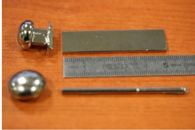
Figure 2.1.2: Zr<sub>65</sub>Cu<sub>15</sub>Al<sub>10</sub>Ni<sub>10</sub> BMG casted in plate and cylindrical shape and the exceeding material removed on the left.
