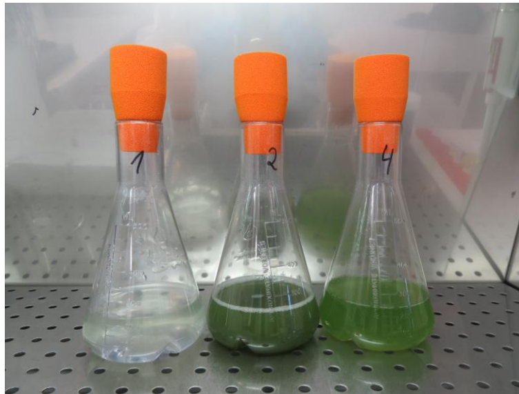
Figure 2-4. Photograph of three reactors illustrating the different optical appearance at different biomass concentrations. Reactor 1 contains a low biomass concentration but no suspended sediments. Reactors 2 and 4 contain about the same biomass concentration (slightly higher in Reactor 4) but reactor 2 appears much more turbid, which is due to a high load of fine-grained suspended sediments.
