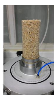
Figure 4.14: Frozen eroded specimen prepared for triaxial compression test.
