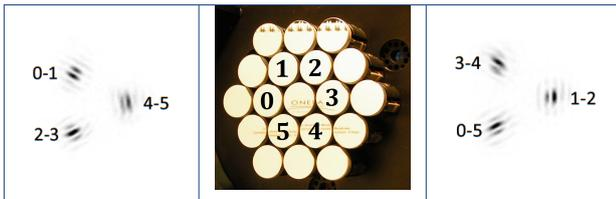
**Fig. 2.** NIRTA segmented mirror (middle). Diversity images (left and right), with superimposition groups and corresponding baselines.
