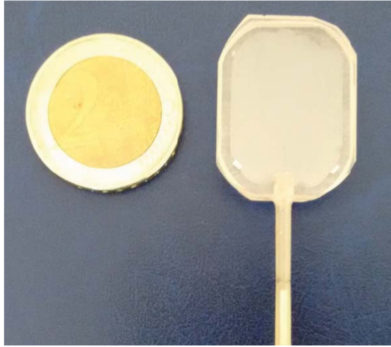
Figure 1.4: Photograph of the micro-cell. For the gap formation thicker platinum trips are used. 2 Euros provides the scale.
